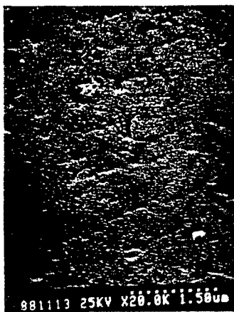
Fig.5 SEM photograph of a YBCO thin film sputtered in Ar+O 2 (30%) at substrate temperature of 600-650°C, and plasma oxidized afterwards
