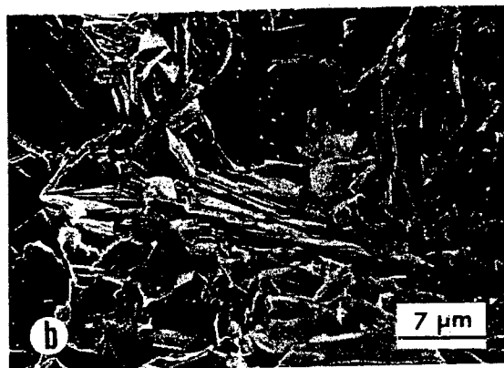
Fig.5 SEM images showing the stages of crystal growth from the 30 to 37 A phases. The specimens were heated finally at 870°C for 12 hr (a) and at 875°C for 12 hr (b).
