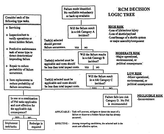
During an RCM analysis, engineers use a decision logic tree to assign the proper mix of maintenance. Figure 1.
