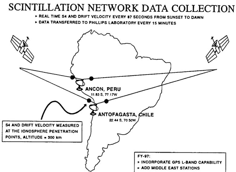
**Figure 1.** Schematic diagram of the UHF portion of the South American data collection system.
