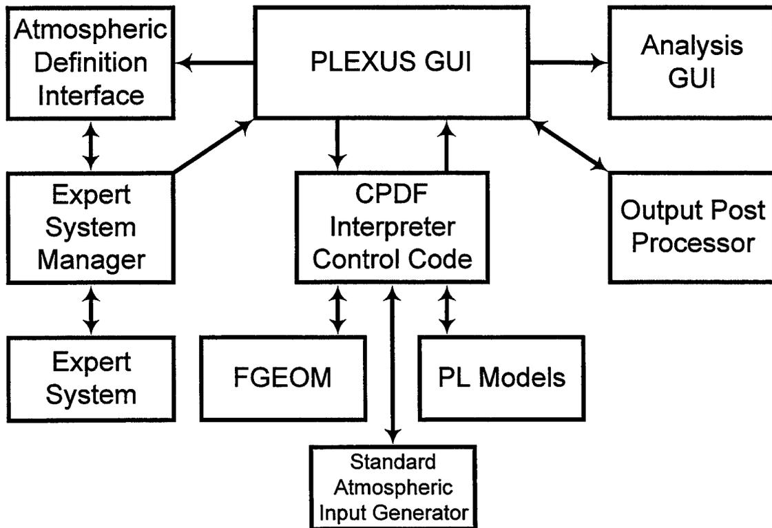
*Figure 1. The Initial PLEXUS Architecture For PC Platforms*
