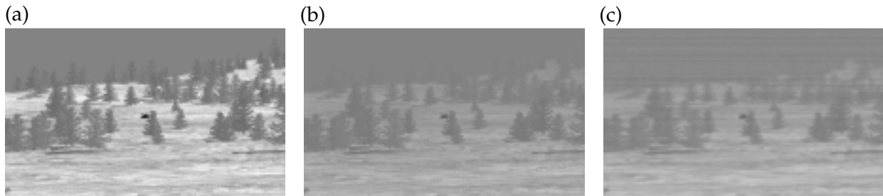
Figure 9. (a) Input image with (b) atmospheric transmission and (c) sensor modeling applied.
