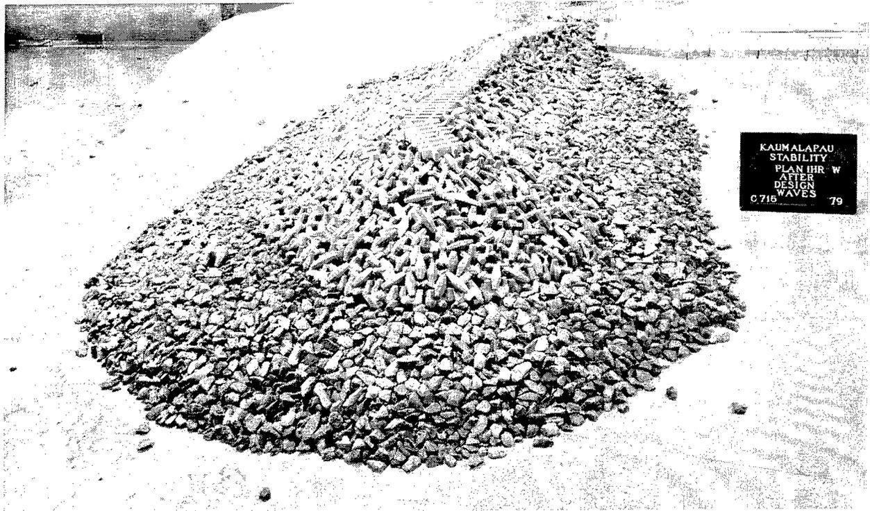
Photo B73. Plan 4H, breakwater head after 9.8- and 12-sec waves at design height and 16-sec waves up to  $H_o = 6.6$  m from 251-deg direction, repeat test
