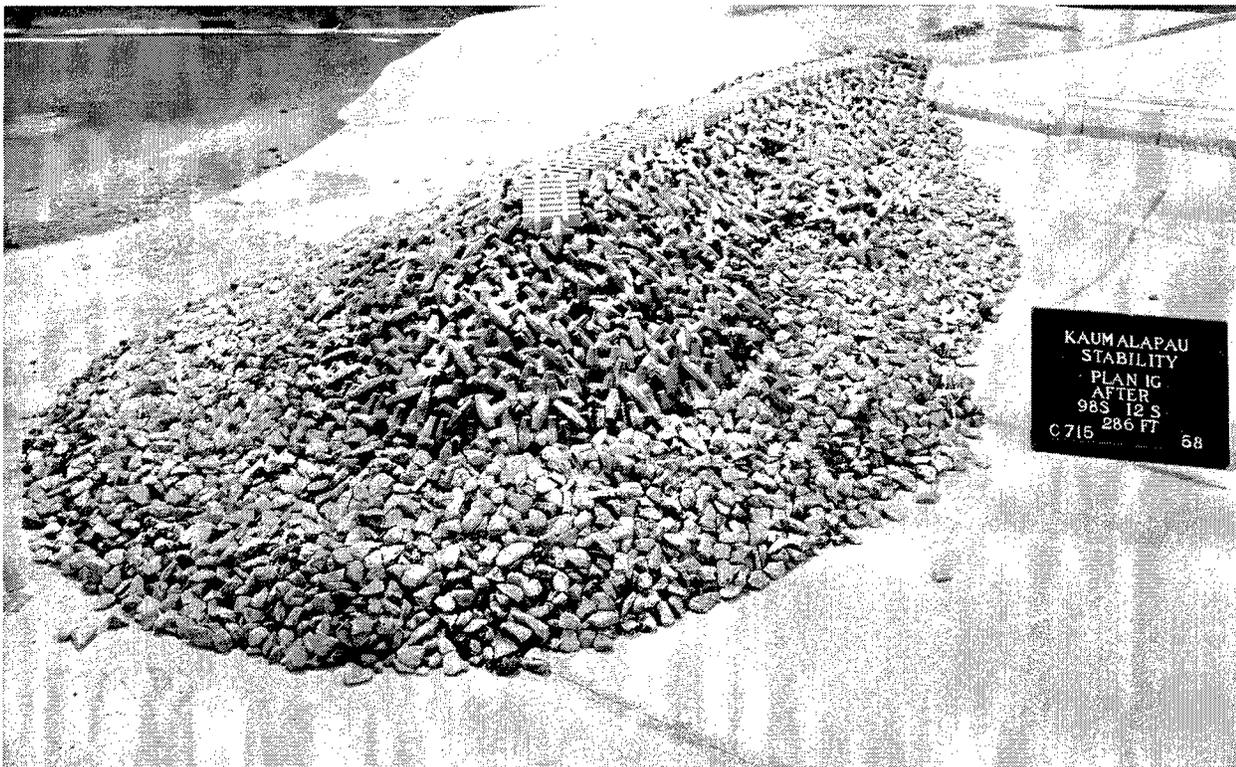
Photo B52. Plan 4G, breakwater head after maximum 9.8- and 12-sec waves
