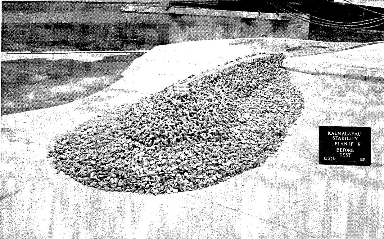
Photo B31. Plan 4F, breakwater head before experiments
