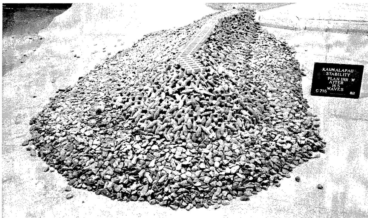
Photo B76. Plan 4H, breakwater head after 9.8- and 12-sec waves and 16-sec waves up to  $H_o = 8.5$  m from 251-deg direction, repeat test
