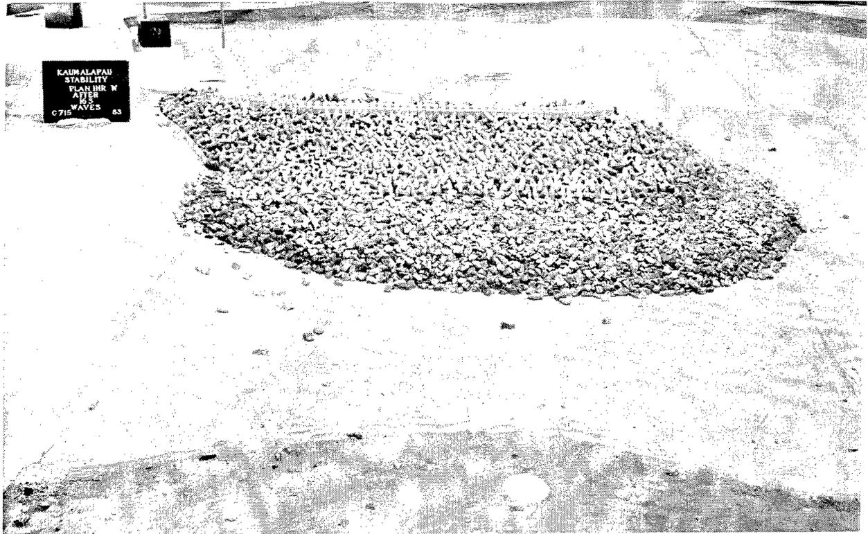
Photo B77. Sea-side view of Plan 4H after maximum 9.8- and 12-sec waves and 16-sec waves up to  $H_o = 8.5$  m from 251-deg direction, repeat test
