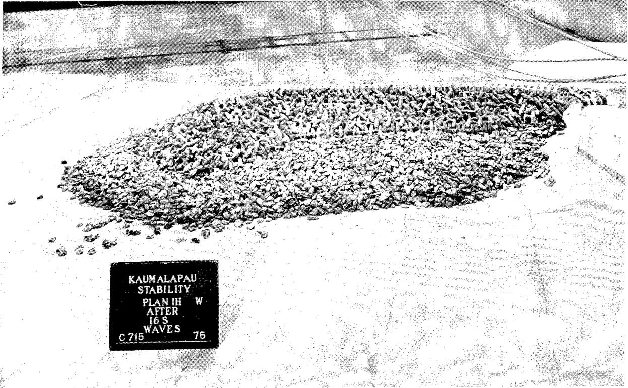
Photo B69. Leeside view of Plan 4H after 16-sec, 7.7-m waves from 251-deg direction
