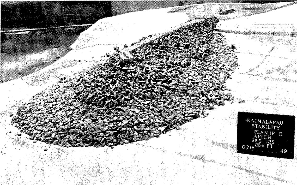
Photo B43. Plan 4F, breakwater head after maximum 9.8-and 12-sec waves
