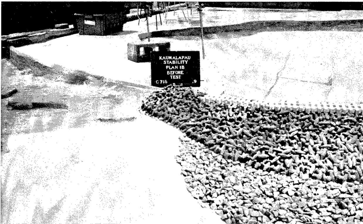
Photo B8. Sea-side shoreward end view of Plan 4B, before experiments
