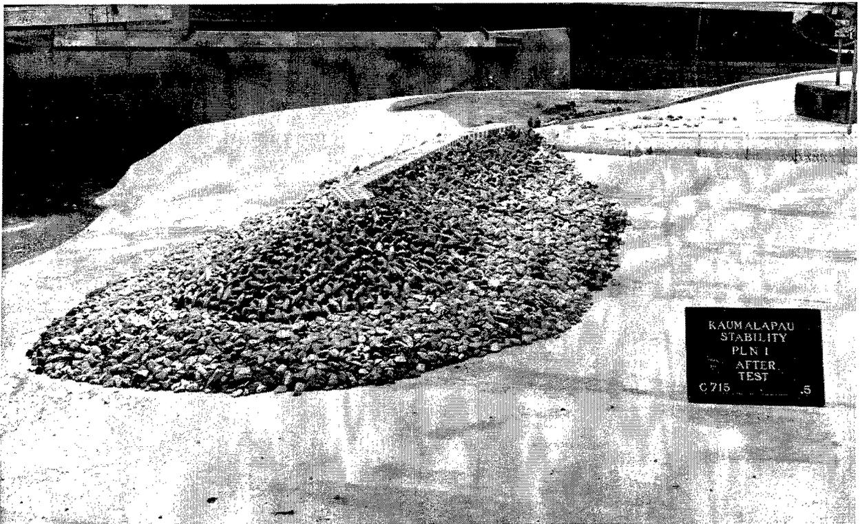
Photo B6. Head view of Plan 4 after 9.8-sec, 7.5-m waves
