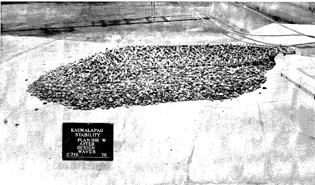
Photo B72. Leeside view of Plan 4H after 9.8- and 12-sec waves at design height and 16-sec waves up to  $H_o = 6.6$  m from 251-deg direction, repeat test
