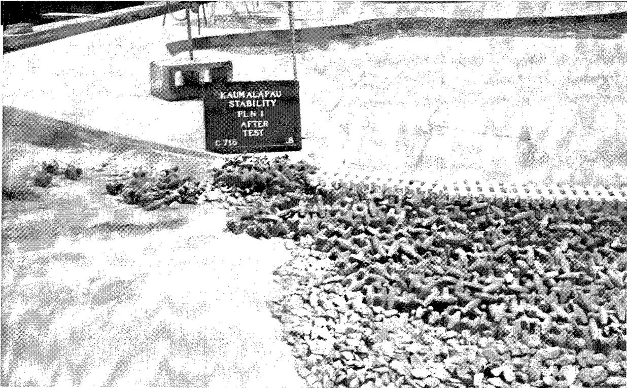
Photo B7. Sea-side shoreward end view of Plan 4A after 9.8-sec, 6.4-m waves
