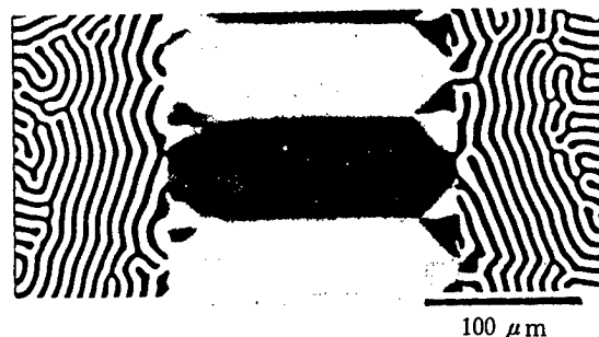
Figure 6. Magnetic Domain Pattern When Changing the Magnetization Direction Garnet Film by Laser Annealing
