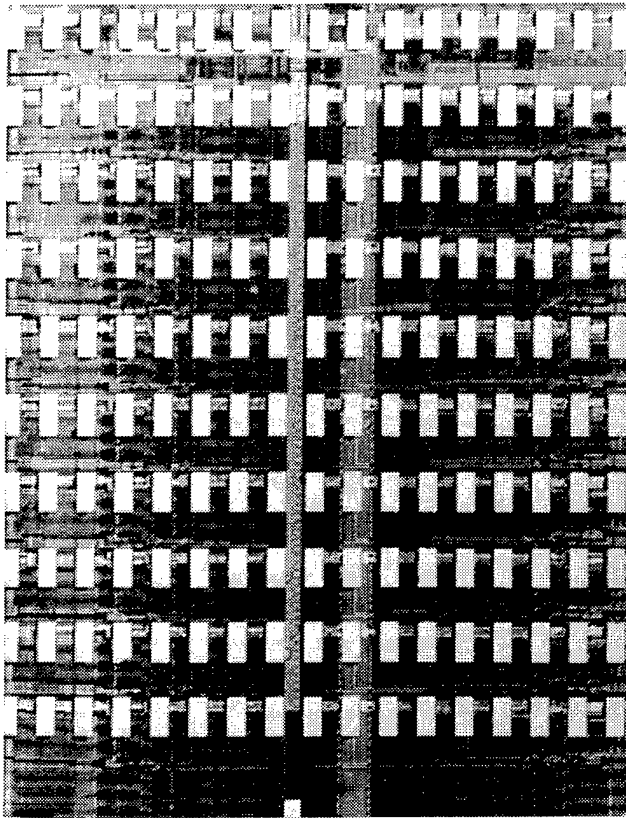
Figure 1: Microphotograph of the 0.8μm, CMOS/MQW-modulator, Static-RAM integrated-circuit, showing a portion of the 10 x 20 array of diodes after bonding and substrate removal [11]. MQW modulators are 20μm x 50μm with 62.5μm / 125μm separations.
