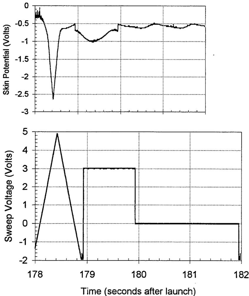
Figure 3. DFF Vehicle Potential Influenced by the Langmuir Probe. Upper frame shows the DFF skin potential measured with respect to a spherical floating probe deployed on an insulating boom. Bottom frame illustrates the Langmuir probe grid bias with respect to the DFF skin.
