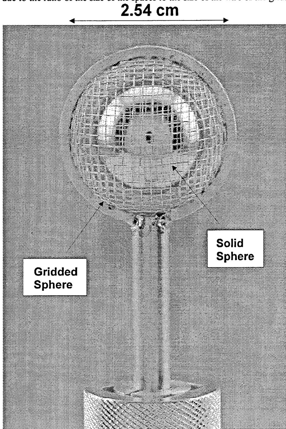
Figure 2. Langmuir Probe Gridded Sphere and Dimensions.
