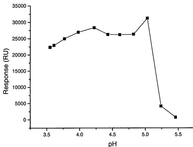
Figure 3: Effect of the pH on the amount of anti-SEB antibodies sorbed into the dextran matrix.
