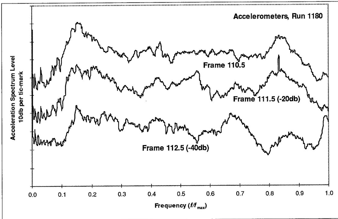
**Figure 53 High frequency accelerometer data, Run 1180**
