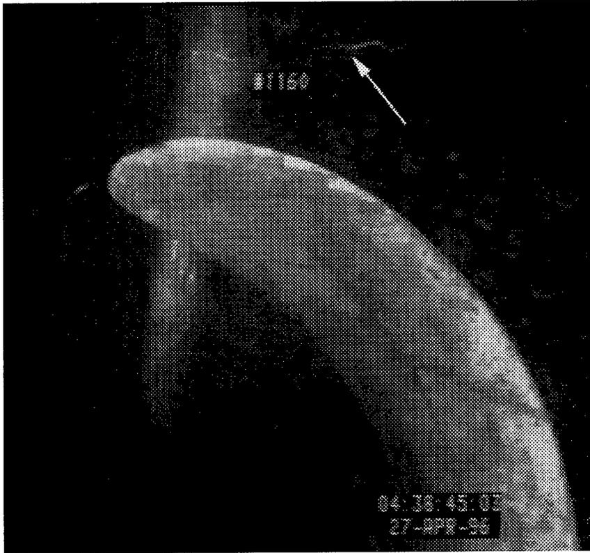
**Figure 37 Propeller cavitation, looking aft, Run 1160**
