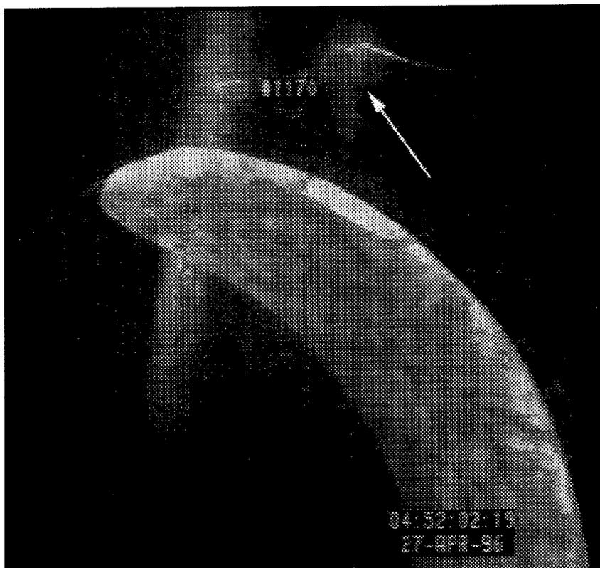
**Figure 43 Propeller cavitation, looking aft, Run 1170**
