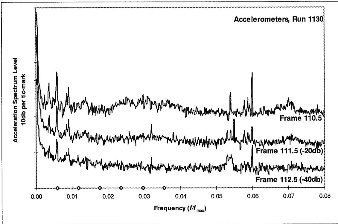
Figure 21 Low frequency accelerometer data, Run 1130
