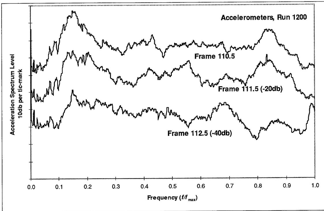
Figure 65 High frequency accelerometer data, Run 1200
