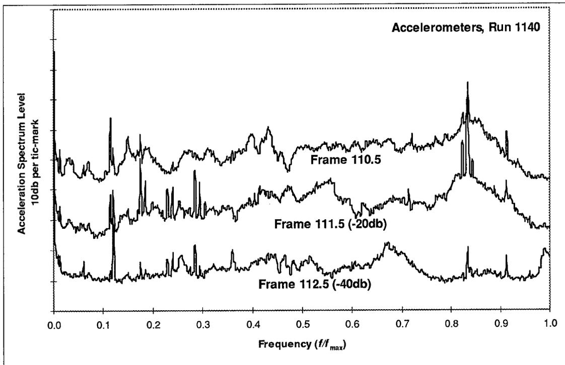
**Figure 29 High frequency accelerometer data, Run 1140**
