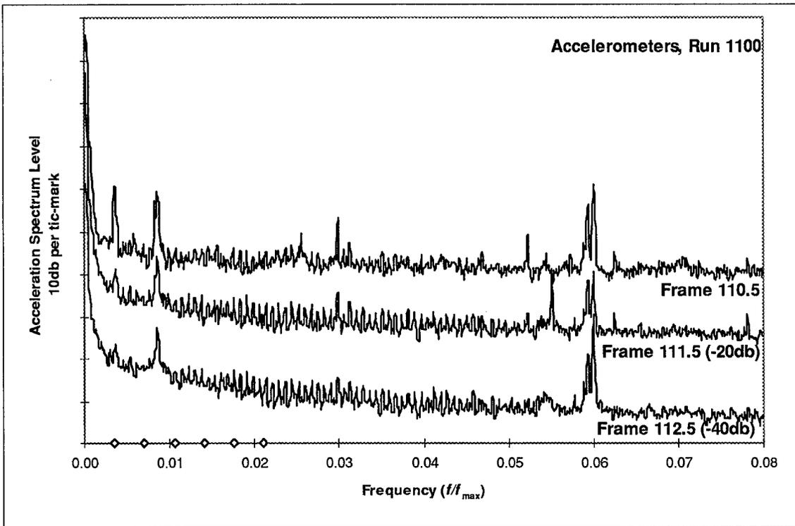
**Figure 4 Low frequency accelerometer data, Run 1100**
