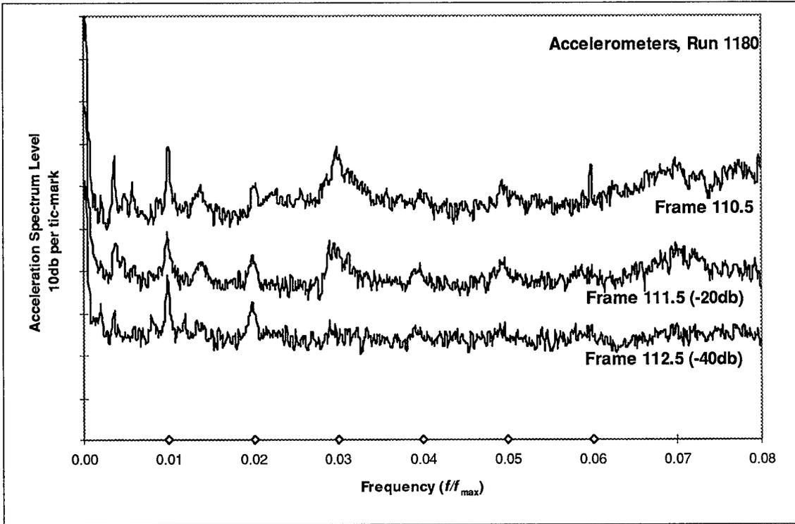
Figure 51 Low frequency accelerometer data, Run 1180
