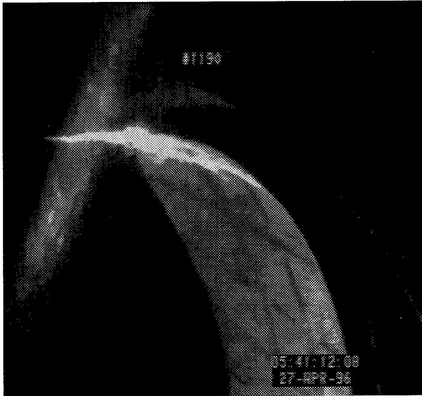
Figure 55 Propeller cavitation, looking aft, Run 1190
