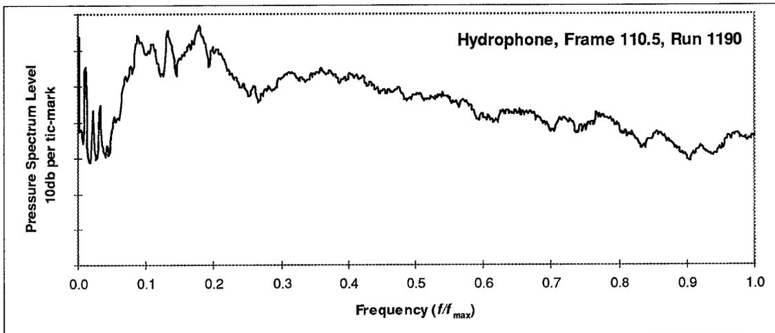
**Figure 60 High frequency hydrophone data, Run 1190**
