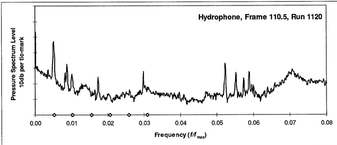
Figure 16 Low frequency hydrophone data, Run 1120
