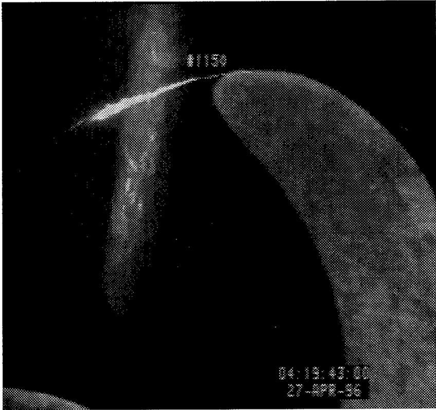
Figure 31 Propeller cavitation, looking aft, Run 1150
