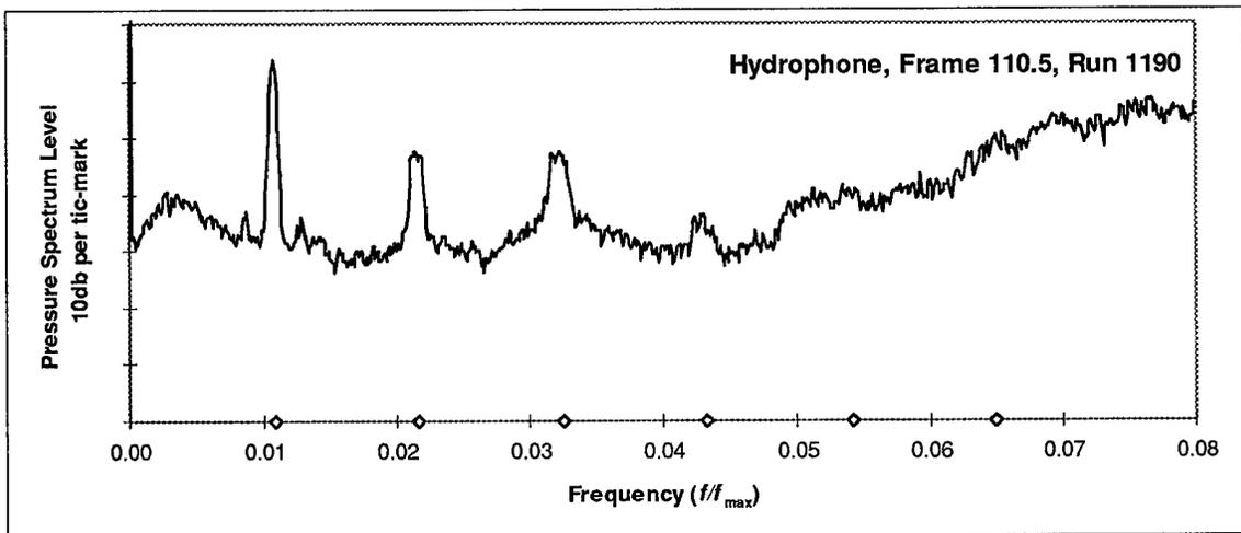
Figure 58 Low frequency hydrophone data, Run 1190
