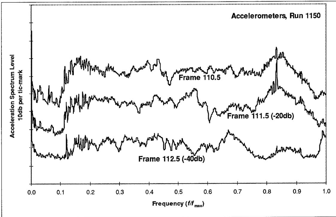
Figure 35 High frequency accelerometer data, Run 1150
