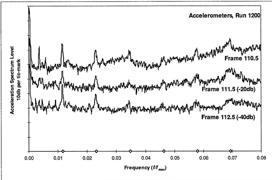
**Figure 63 Low frequency accelerometer data, Run 1200**
