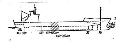
Location of cylindrical insert (shaded). 1--design waterline
