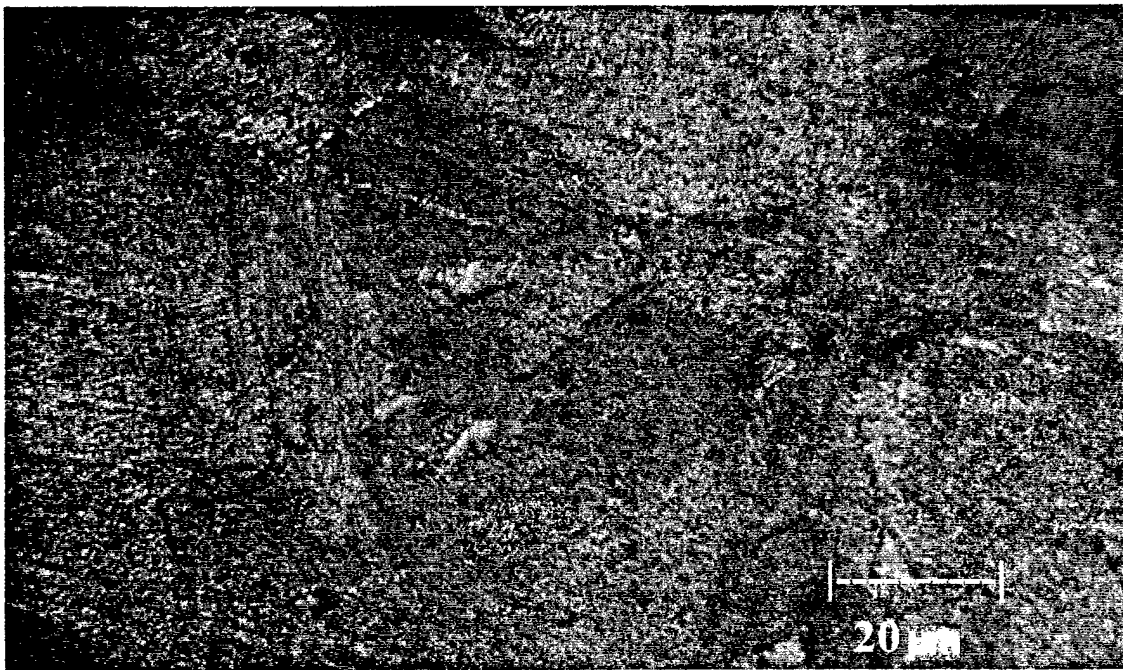
Figure IV.3: Micrograph of OFHC Cu annealed at 600°C for four hours. The micron bar corresponds to 20 \mu\text{m} and a magnification of 100 x.
