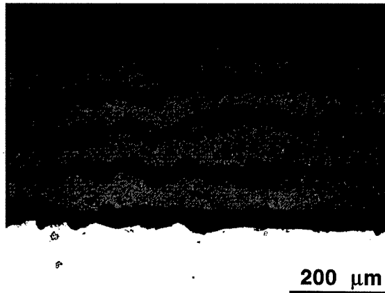
Fig. 6(a) Microstructure of PS AZ4 coating in the as-sprayed condition
