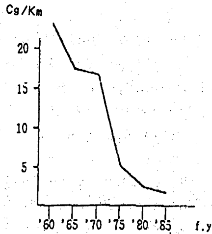
Fig.9-5 The CO emissions from automobiles per unit running kilometer (including trucks)
