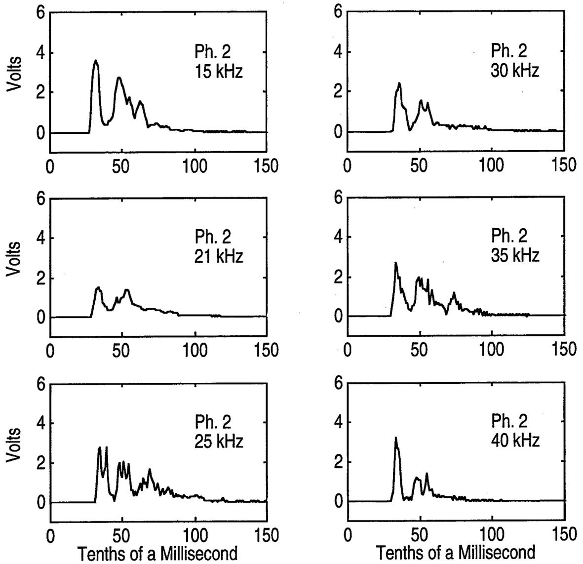
Figure B2. Phone 2 mean envelopes of 0.5 ms pulses.
