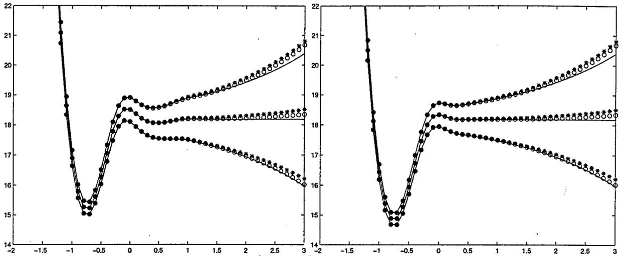
FIGURE 5. Apparent Resistivity (Ohm-m) *vs.* Logarithm of Frequency (Hz): a comparison of theory and simulations. The mean and mean  $\pm$  one standard deviation are plotted for (a) the thin resistive layer present and (b) the layer absent. The solid lines represent the theory. The circles and stars represent the two random layering models used in the simulations.
