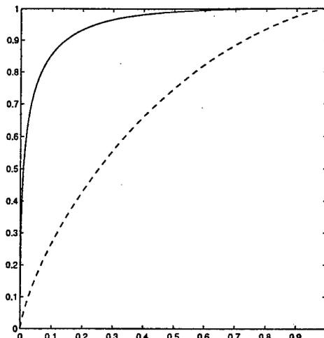
FIGURE 13. The Importance of Using Correct Covariance Information: the case of detecting a 50 m thick resistive layer in the presence of  $\nu^2 = 10^{-11}$  added noise is considered. The solid curve is the ROC curve using correct covariance information while the dashed curve represents the case where these covariance weights have been replaced by the identity matrix.
