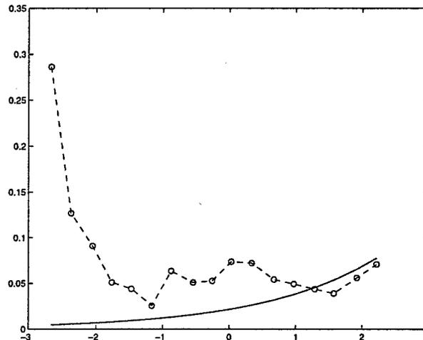
FIGURE 3. Comparison of Uncertainty Levels: Apparent Resistivity Uncertainty *vs.* Logarithm of Frequency (Hz). The solid curve represents uncertainty due to resistivity microstructure. The circles are uncertainty levels reported by Parker [12].
