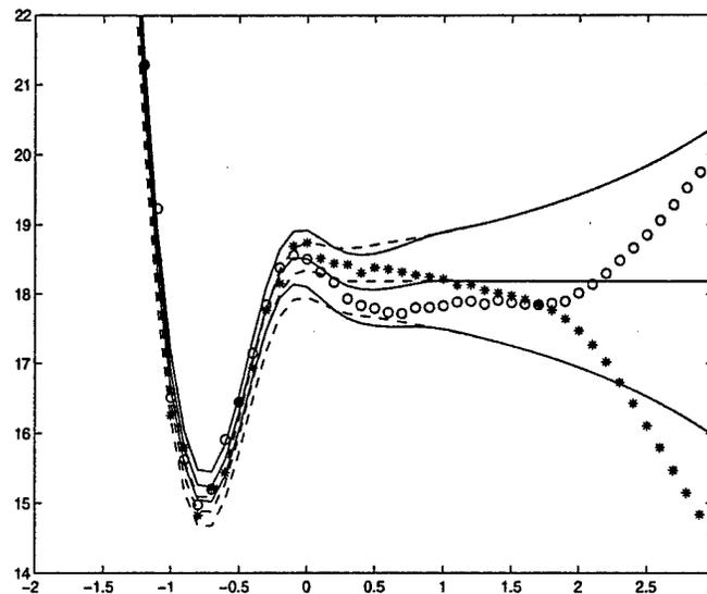
FIGURE 9. The Detection Problem: Apparent Resistivity (Ohm-m) *vs.* Logarithm of Frequency (Hz). The solid and dashed curves are predictions of the theory for the resistive layer being present and absent, respectively. The mean and mean  $\pm$  one standard deviation are shown for each case. The circles and stars are two different realizations, *i.e.* two different sets of random microstructure, both for the case where the layer is present.
