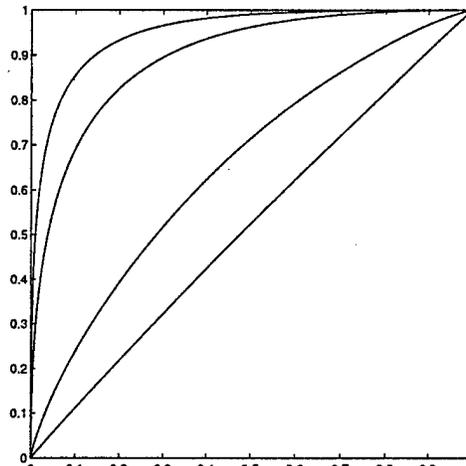
FIGURE 12. The Effect of Added Noise upon Detection: ROC curves are plotted for a resistive layer thickness of 50 m and added noise levels of  $\nu^2 = 10^{-11}, 10^{-9}, 10^{-7},$  and  $10^{-5}$ . The curves decrease monotonically as the noise level is increased.
