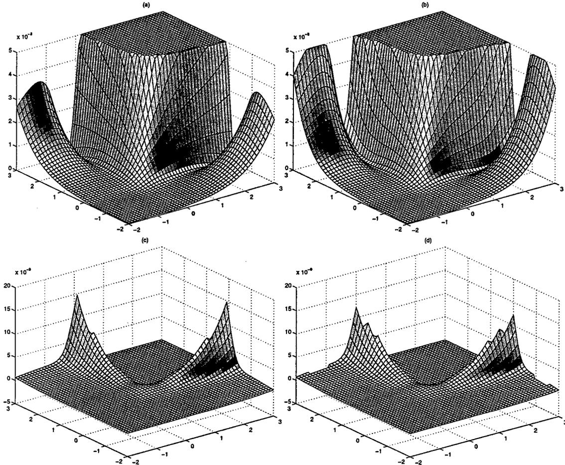
FIGURE 8. Real-Real Covariance Submatrix *vs.* Logarithmic Frequency. The first two figures show the fine scale structure of  $C^{RR}$ , as computed by (a) theory and (b) simulations. The latter two figures show the effect of the thin resistive layer upon the covariance submatrix, *i.e.*  $C_1^{RR} - C_0^{RR}$ , as computed by theory in (c) and simulations in (d).
