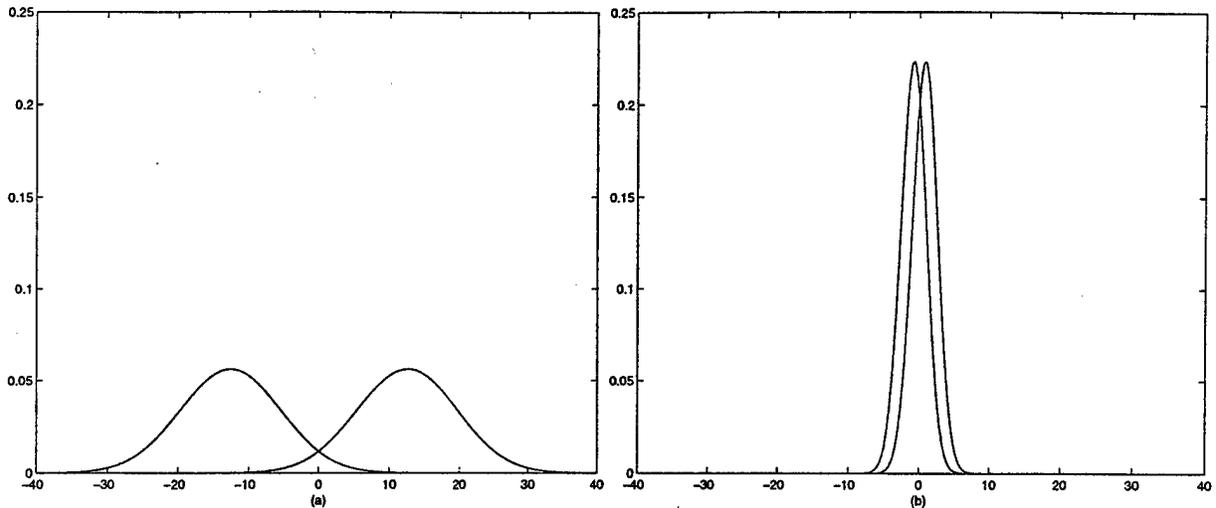
FIGURE 10. Probability Density Functions for the Detection Problem: Density functions  $q_0$  and  $q_1$  for a (a) 100 m thick resistive layer and (b) 25 m layer. In each case, the density function  $q_0(Q)$ , corresponding to the layer absent, appears on the left while the density function  $q_1(Q)$ , corresponding to the layer present, appears on the right.
