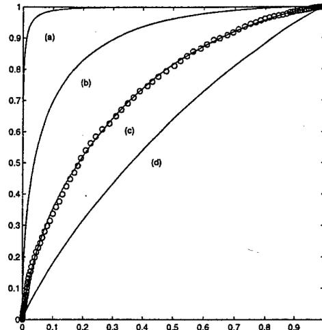
FIGURE 11. ROC Curves: Probability of Detection *vs.* False Positive Rate for a resistive layer thickness of (a) 100 m, (b) 50 m, (c) 25 m, (d) 10 m, constructed using the theory. The circles represent a corresponding curve created using the simulations.
