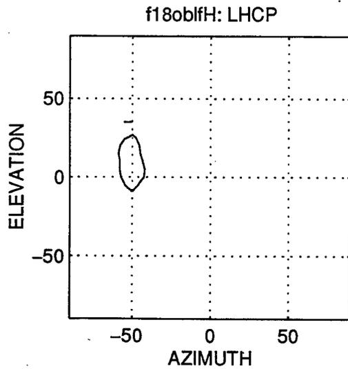
Figure 30: CATM outboard, high frequency, outboard microstrip antenna pattern (mode 2).
