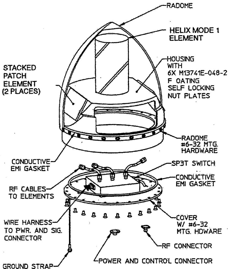
Figure 8: JSOW antenna assembly (From [8]).
