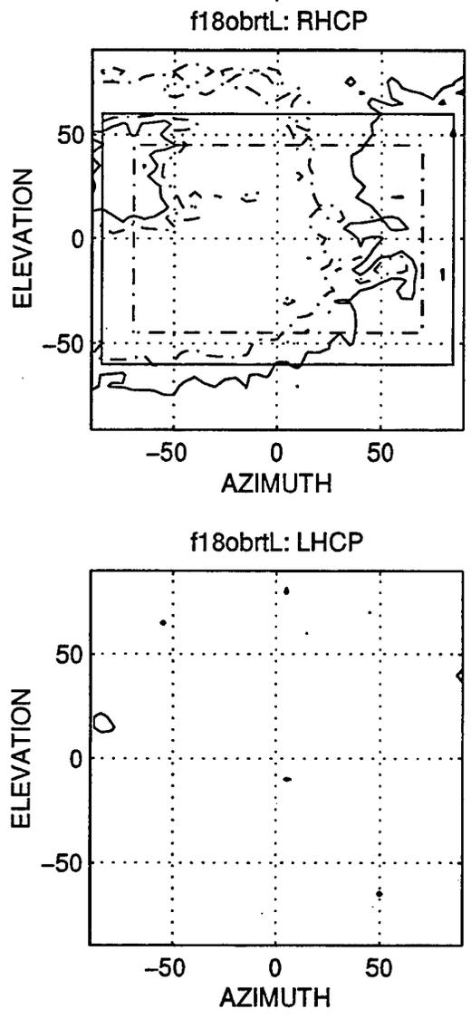
Figure 31: CATM outboard, low frequency, inboard microstrip antenna pattern (mode 2).
