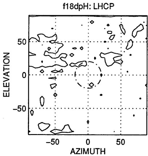
Figure 27: CATM outboard, with drop tank, high frequency, helix antenna (mode 1).
