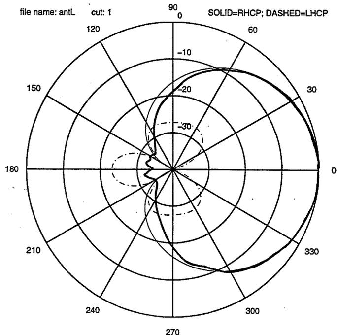
Figure 11: Comparison of measured and calculated helix azimuth pattern at  $f_L$ ,  $EL=0$ . (Heavy line: measured; thin line calculated.)
