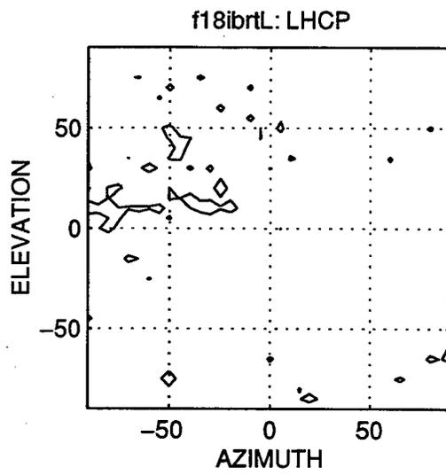
Figure 36: CATM inboard, low frequency, inboard microstrip antenna pattern (mode 2).
