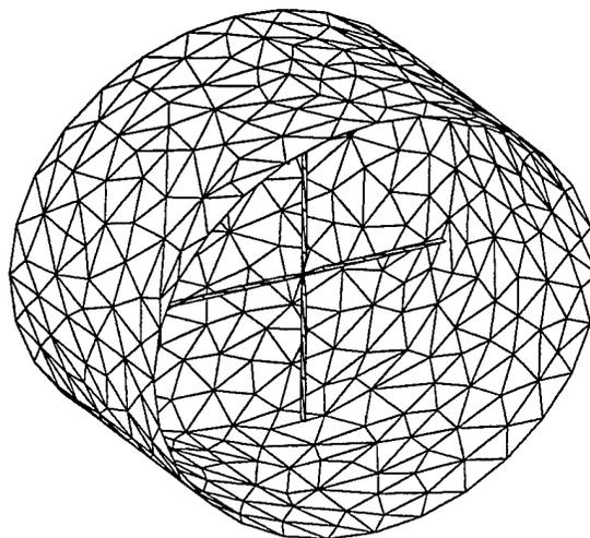
Figure 10: PATCH model used to generate the antenna patterns.
