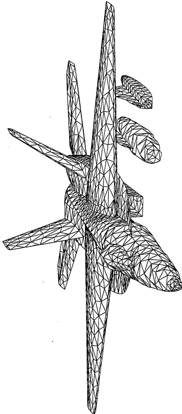
Figure 7: F-18, drop tank, and CATM facet model built with ACAD.
