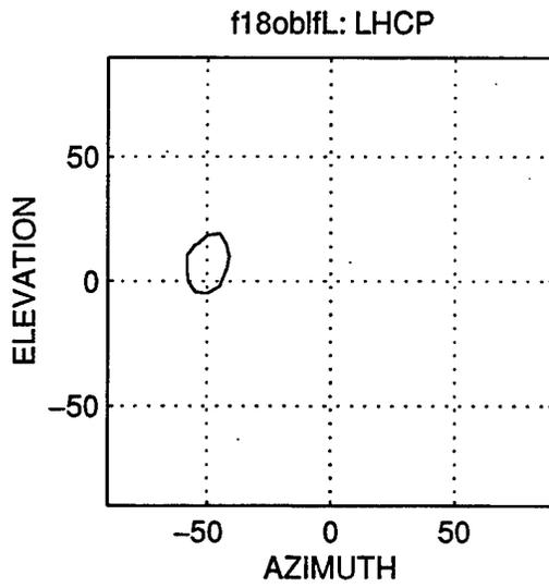
Figure 29: CATM outboard, low frequency, outboard microstrip antenna pattern (mode 2).
