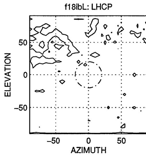
Figure 22: CATM inboard, low frequency, helix antenna (mode 1).
