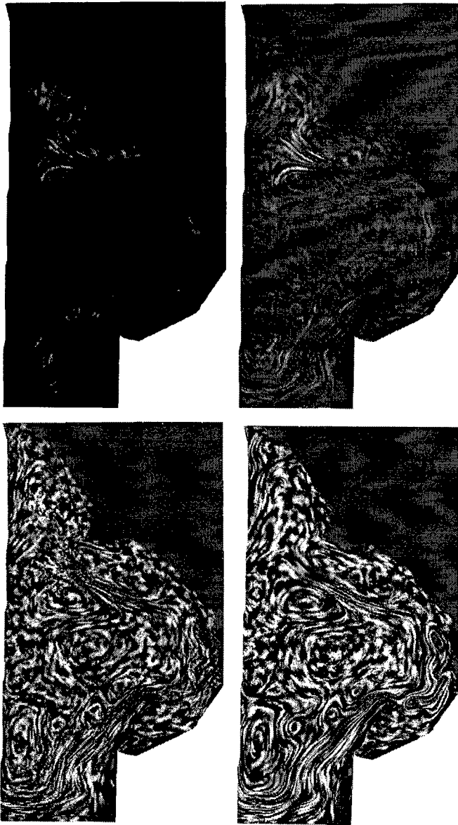
Fig. 8. Slice from the bay of Gdansk data set visualized with different methods: colour (see also Appendix), spot intensity scaling, velocity perturbation and texture blurring.
