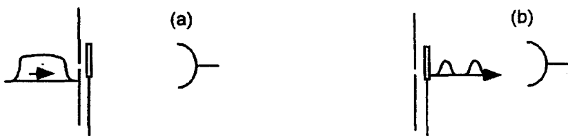
Fig. 1. (a) A quasi-monochromatic wave packet is incident onto a chopper which is opened for two short periods. (b) For matter waves the spreading of the two wave packets may lead to interferences in the signal recorded by the detector. This is not possible for light waves propagating in a non dispersive medium.
