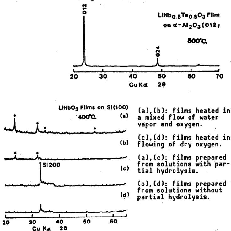
Figure 3. XRD Profiles of  $\text{Li}(\text{Nb},\text{Ta})\text{O}_3$  Films
