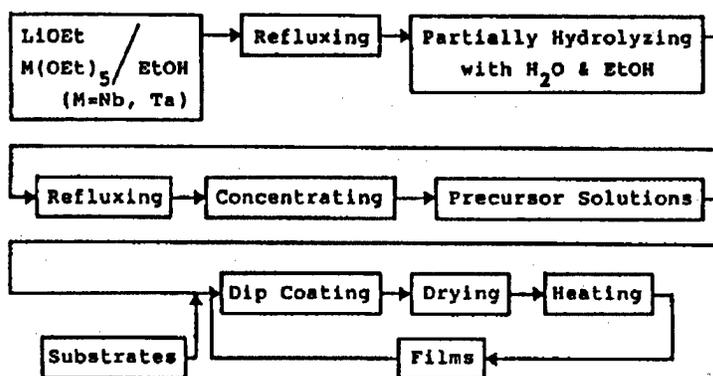
Figure 2. Preparation of  $\text{Li}(\text{Nb},\text{Ta})\text{O}_3$  Film
