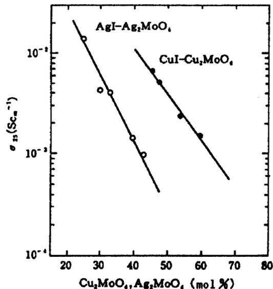
Figure 11. Compositional Dependence of Ion Conductivity (25°C) in CuI-Cu<sub>2</sub>MoO<sub>4</sub>-System Glass and Ag<sub>2</sub>MoO<sub>4</sub>-System Glass (Cited from Ref. 16 material)
