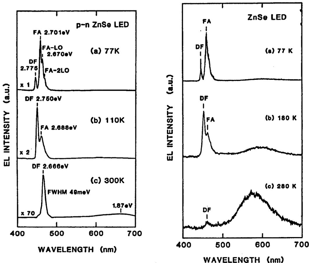
Figure 10. Luminescence Spectra for pn-Junction LEDs
