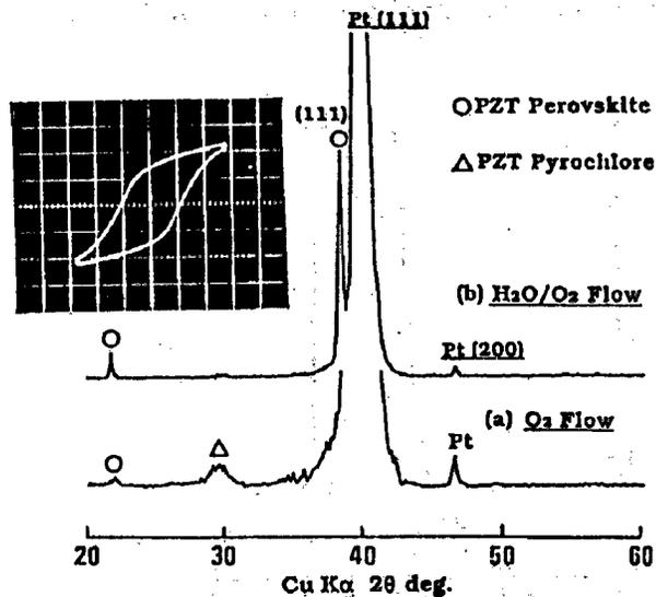
Figure 6. XRD Profiles of PZT (Zr:Ti = 53.47) Thin Films on Substrate (Pt/Ti/SiO<sub>2</sub>/Si) Fired at 600°C for 2h. Condition of calcination: (a) O<sub>2</sub> flow; (b) H<sub>2</sub>O/O<sub>2</sub> flow
