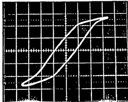
Figure 4. D-E Hysteresis Loop of  $\text{LiNbO}_3$  Thin Film on  $\text{Si}(111)$  Substrate at  $550^\circ\text{C}$ .
