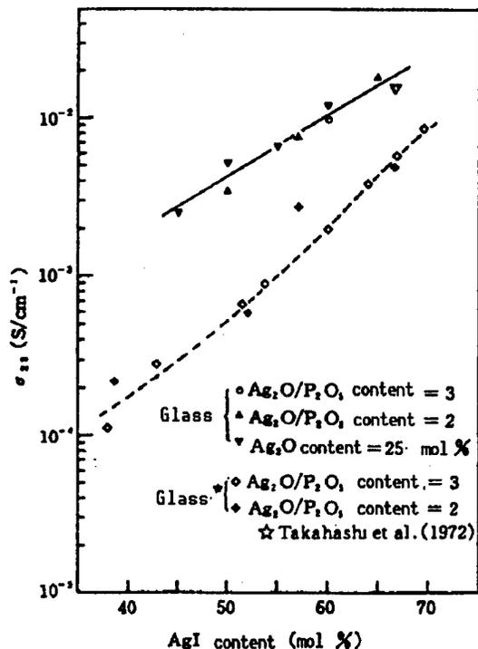
Figure 1. Comparison of Ion Conductivity Between AgI-Ag<sub>2</sub>O-P<sub>2</sub>O<sub>5</sub>-System Crystals and Same-System Glass at 25°C (Cited from Ref. 3 material)
