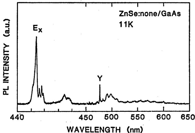
Figure 2. Low-Temperature PL Spectrum in No-Additive-Containing ZnSe
