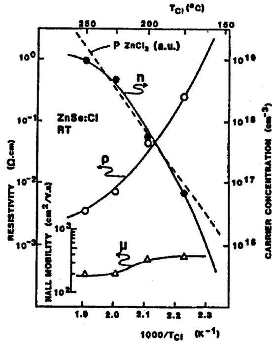
Figure 3. Electric Characteristics in Cl-Doped n-Type ZnSe (Effect of  $\text{ZnCl}_2$  cell temperature)
