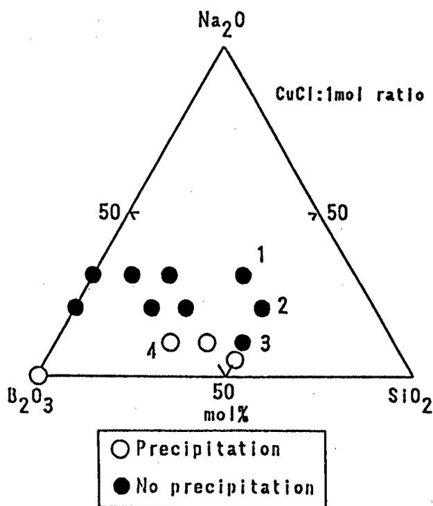
Figure 4. CuCl Precipitated Glass Composition
