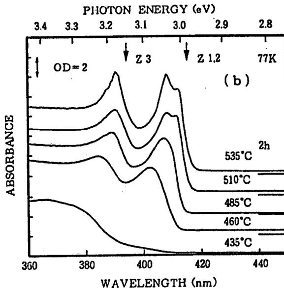
Figure 9. Absorption Spectra in Fine-Particle-Scattered Glass
