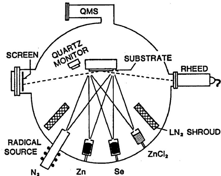
Figure 1. Schematic Representation of MBE Apparatus Reaction Chamber
