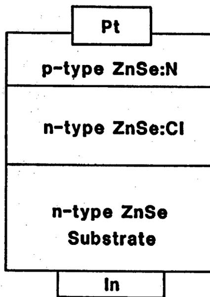
Figure 8. Construction in Fabricated pn-Junction LEDs
