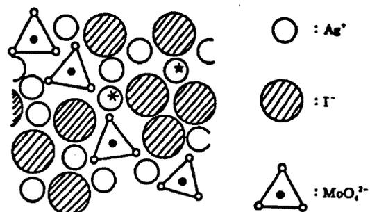
Figure 10. Structure Model of AgI-Ag<sub>2</sub>MoO<sub>4</sub>-System Glass
