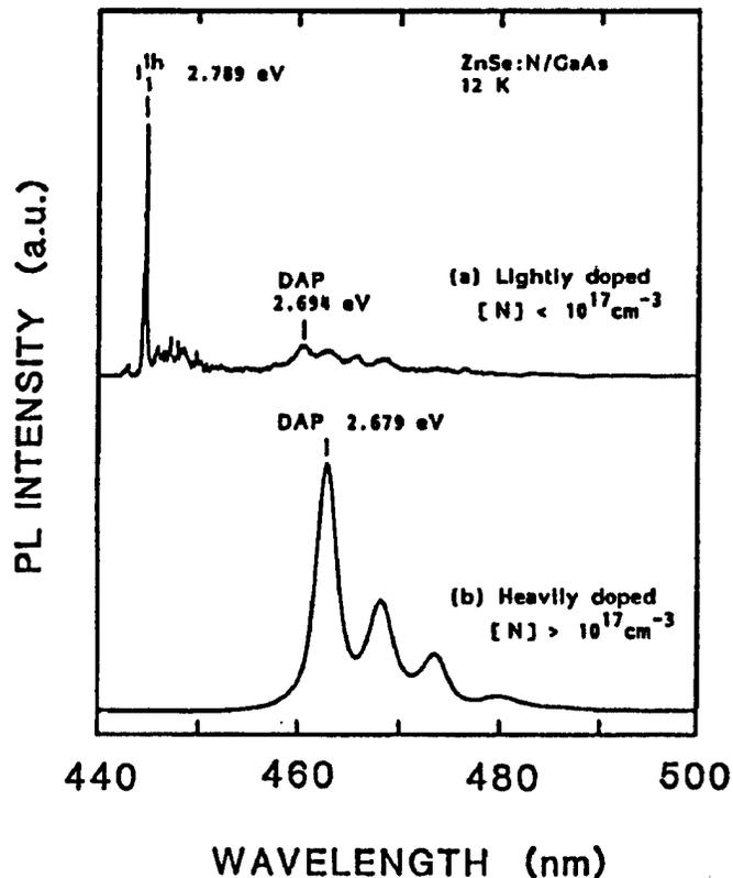
Figure 5. Low-Temperature PL Spectra for Activated N-Doped ZnSe
