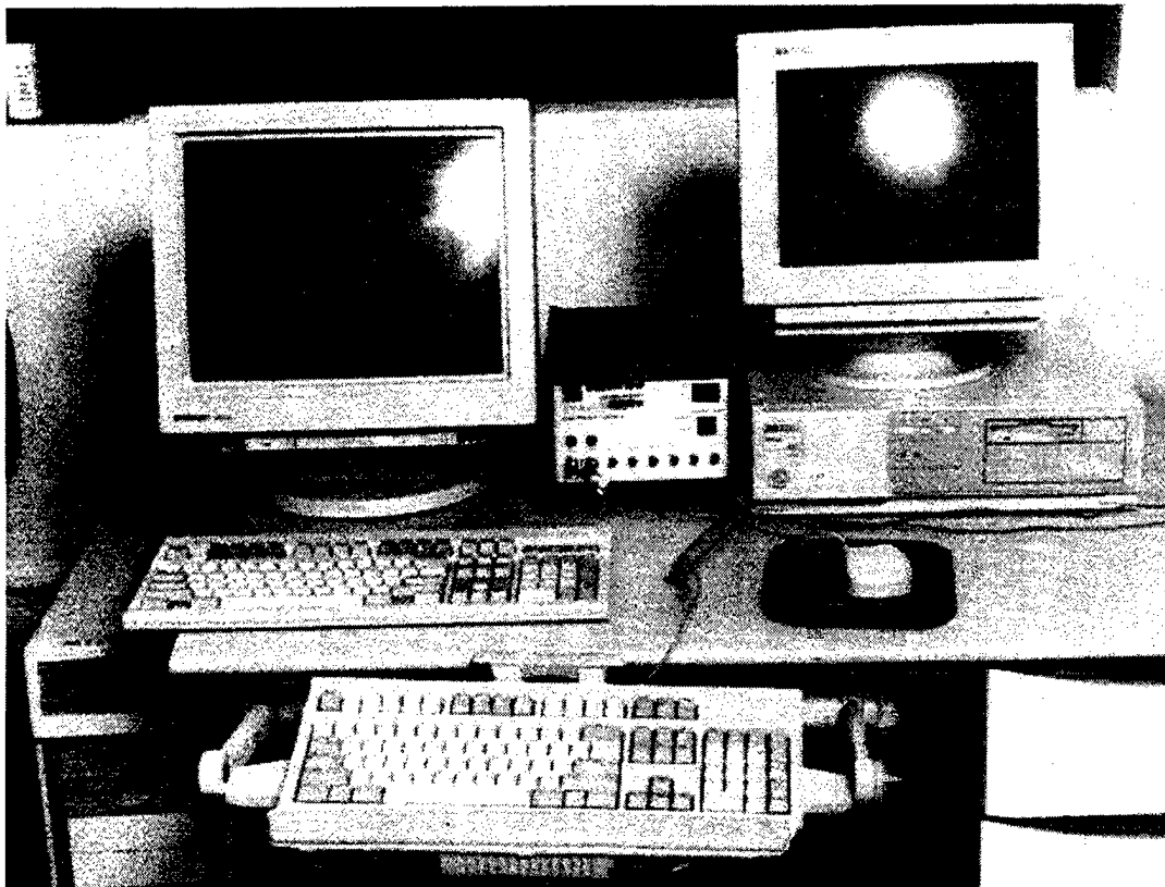
Figure E.1 ECA, ECA sensor interface, and SF-901 Dynamometer computer.
