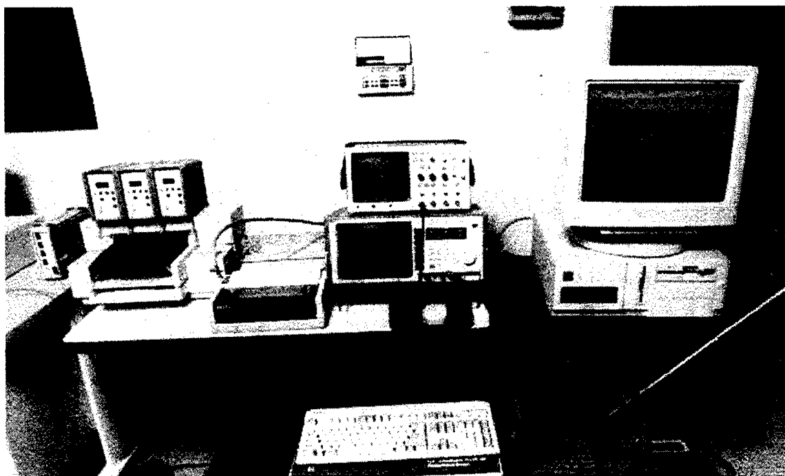
Figure D.1 MDA and high speed data acquisition computer. An oscilloscope sets on top of the MDA.
