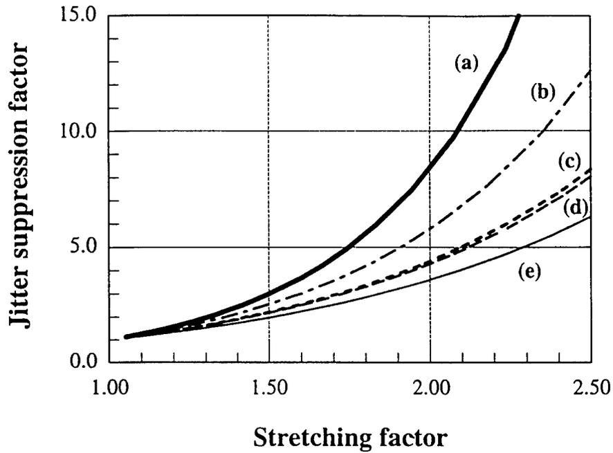
Fig.5b: JSF vs stretching factor (when either  $L_1$  or  $L_2$  equals  $4L_{amp}$ )
