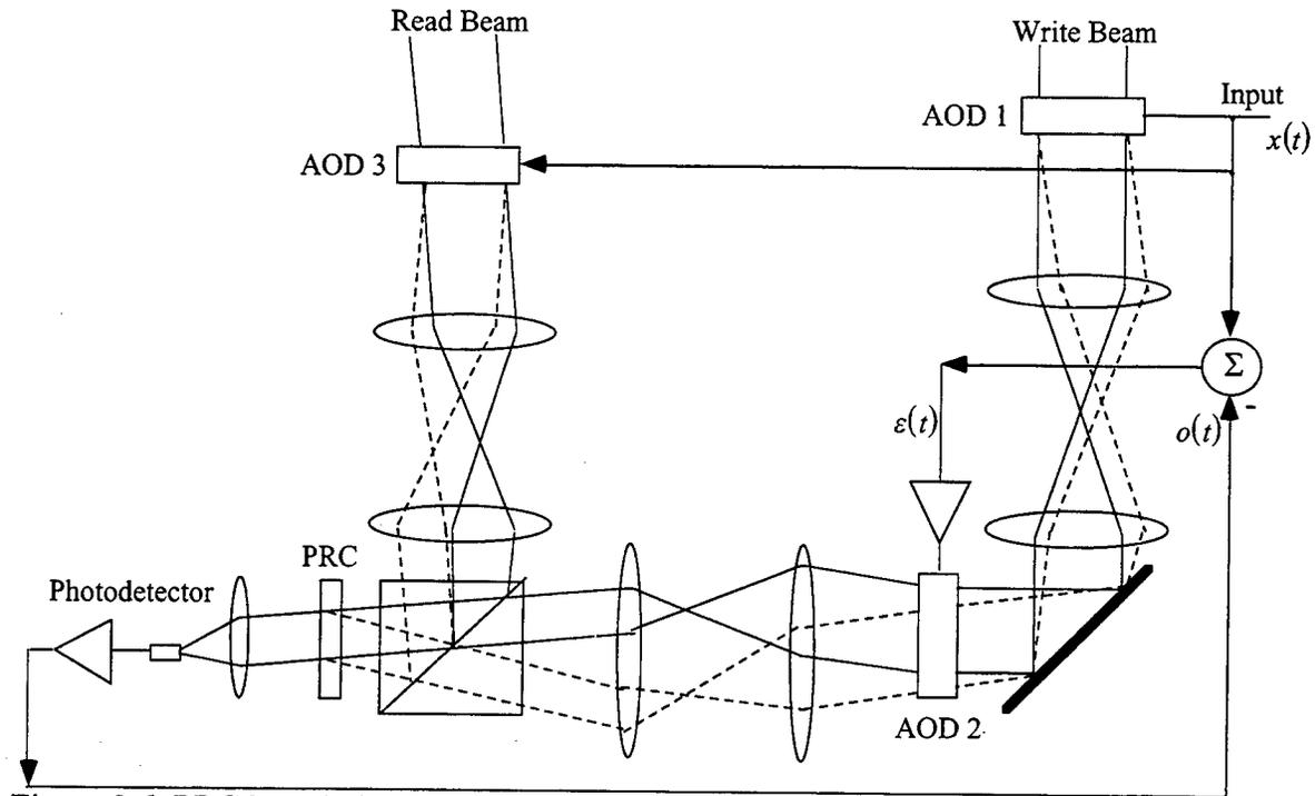
Figure 3.6. PRC based, time-integrating adaptive filter.
