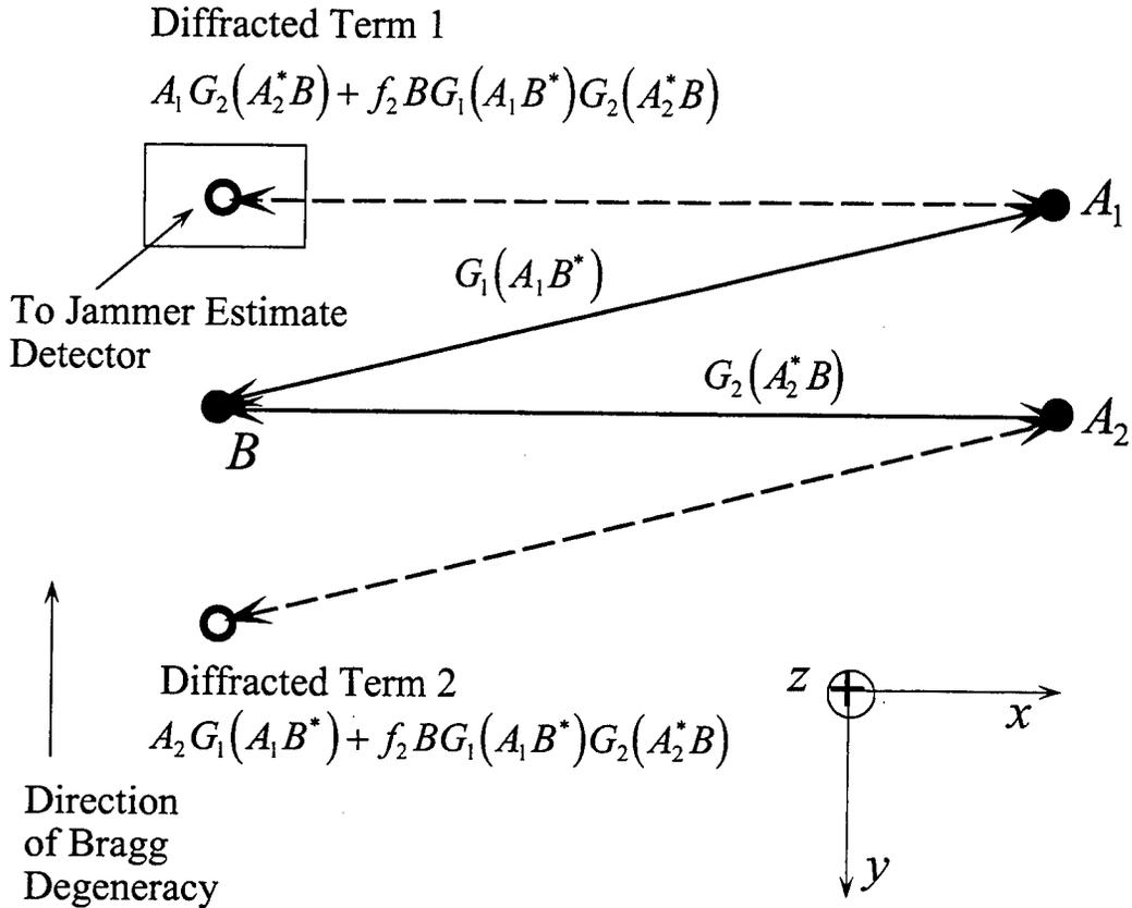
Figure 5.4. Planar representation of angle multiplexing using Bragg degeneracy technique. Write beams  $B$ ,  $A_1$ , and  $A_2$  propagate in the nominal  $z$  direction (into the page) and produce gratings  $G_1(A_1 B^*)$  and  $G_2(A_2^* B)$ .  $A_1$  and  $A_2$  diffract off these gratings to produce the spatially and angularly separable diffracted beams at the left of the figure.
