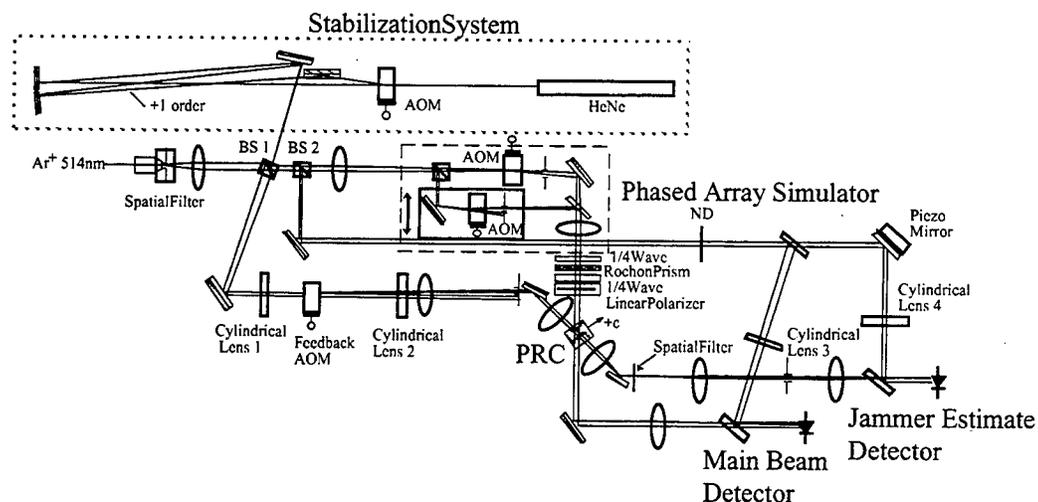
Figure 7.19. Optical component layout of jammer nulling processor using Bragg degeneracy for write/read separation.
