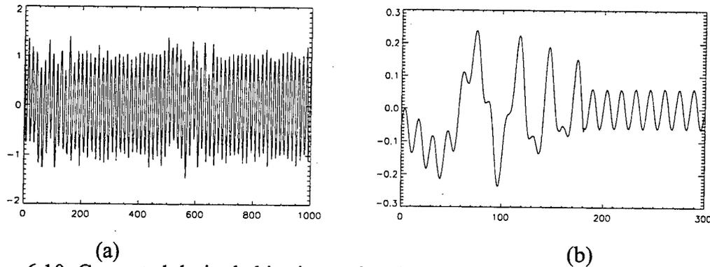
Figure 6.10. Corrupted desired chirp input signal shown in (a), and recovered desired signal in (b) demonstrating an SINR improvement of approximately 24 dB in the presence of a strong jammer.
