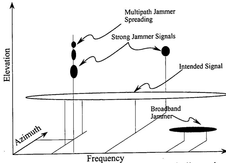
Figure 1.1. Received signal environment shown as 3-dimensional space, two dimensions of angle-of-arrival and one of temporal frequency.
