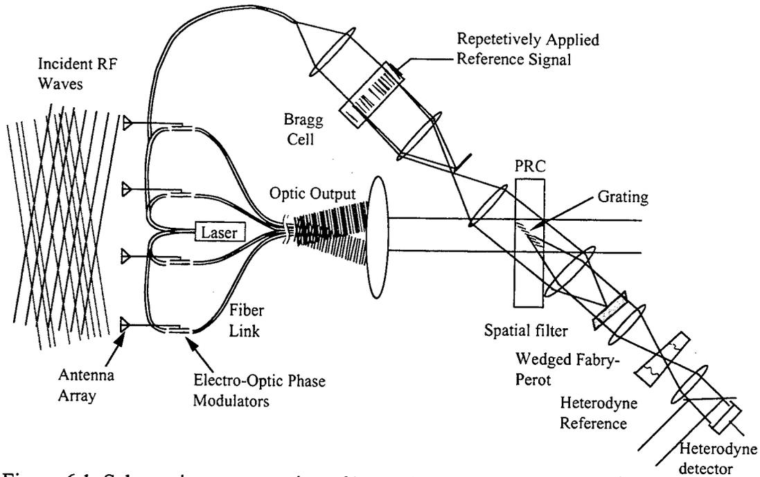
Figure 6.1. Schematic representation of beam-forming phased-array radar processor
