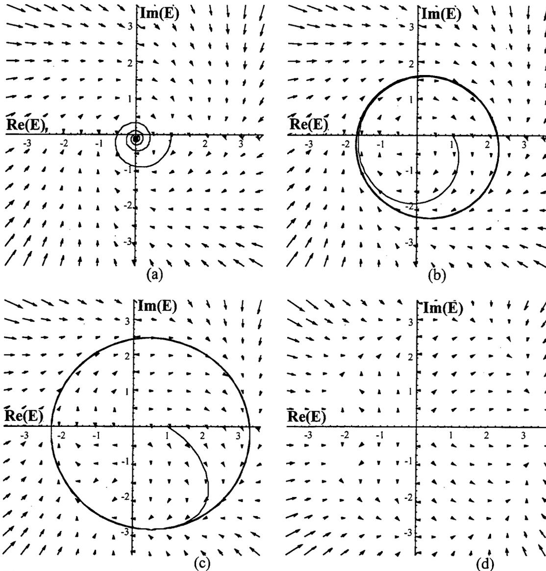
Figure 7.9. Plot of single jammer excision in the complex plane, superimposed over a vector-velocity-field (time interval of 3 seconds). The phase difference increases from  $\pi/2$  to  $\pi$  by  $\pi/6$  for each plot in the sequence. The simulation parameters are the same as those for figure 7.7.
