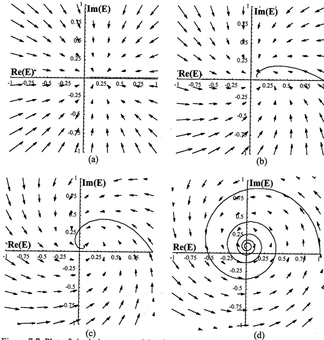
Figure 7.7. Plot of single jammer excision in the complex plane, superimposed over a vector-velocity-field (time interval of 3 seconds), for  $a = 1$ ,  $b = 20$ . The phase difference increases from 0 to  $\pi/2$  by  $\pi/6$  for each plot in the sequence.
