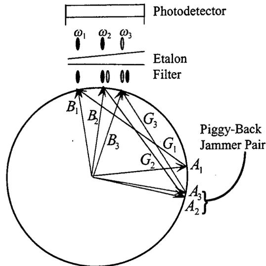
Figure 7.2. Jammers  $A_2$  and  $A_3$  have narrowly separated optical AOAs and hence diffract off of each gratings. This piggy-back diffraction of  $A_2$  off of the grating written by  $A_3$ , and  $A_3$  off of the grating written by  $A_2$  produces spurious frequency terms, which are consequently blocked by the etalon filter before photodetection.
