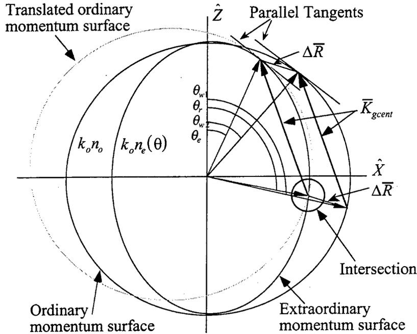
Figure 5.10. Ordinary momentum surface is translated by  $\Delta \bar{R}$  such that points of parallel tangency coincide. Point of intersection (or difference of  $\Delta K \approx \pi/L$ ) between translated ordinary surface and extraordinary surface determines extraordinary plane-wave read-out angle  $\theta_r$ . Ordinary plane-wave write beam angle at  $\theta_{w1}$  is then determined by translation back by  $\Delta \bar{R}$ .
