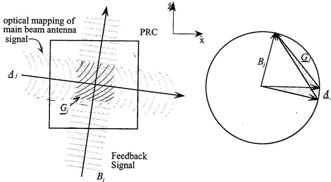
Figure 7.4. Interference at photorefractive crystal between the  $j$ th single frequency jammer  $A_j$  of arbitrary spatial profile and feedback beam  $B_j$  containing frequency content of  $A_j$ . The real space representation is shown at the left of the figure illustrating near field curvature, and the momentum space representation is on the right illustrating two distinct jammers.
