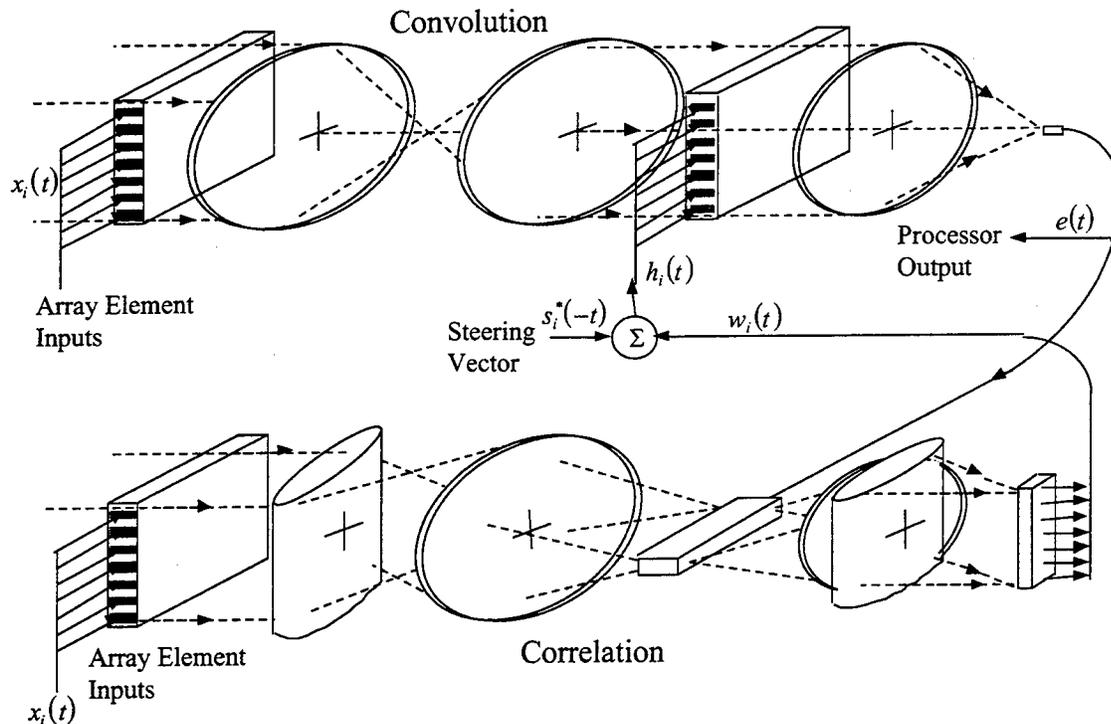
Figure 3.5. Optical implementation of 3-D space-time optical processor
