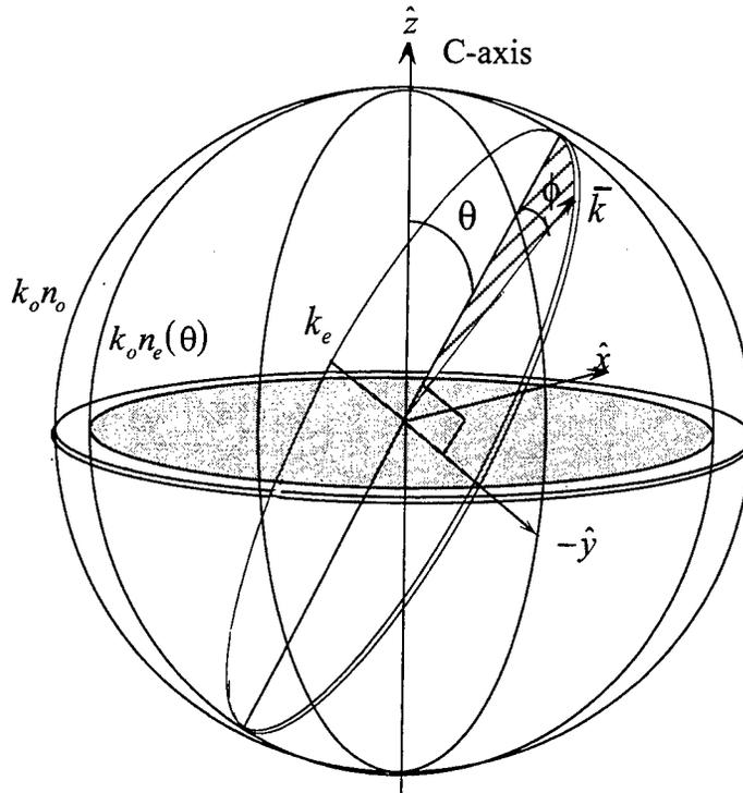
Figure 5.7. Uniaxial crystal 3D momentum surfaces showing ellipse formed between axes  $k_e(\theta)$  and the  $\hat{Y}$  axis. Ellipse is in plane inclined at angle  $\theta$  from C-axis, and angle  $\phi$  moves vector  $\bar{k}$  along elliptical path.
