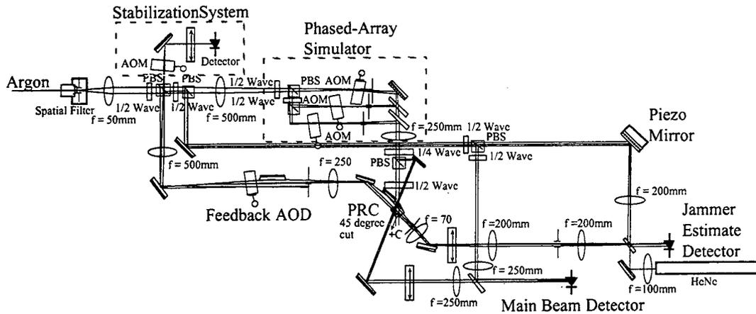
Figure 7.22. Optical component layout of jammer nulling processor using orthogonal polarizations for write/read separation.
