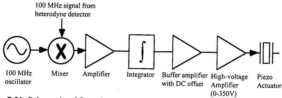
Figure 7.21. Schematic of first piezo actuator driver circuit.
