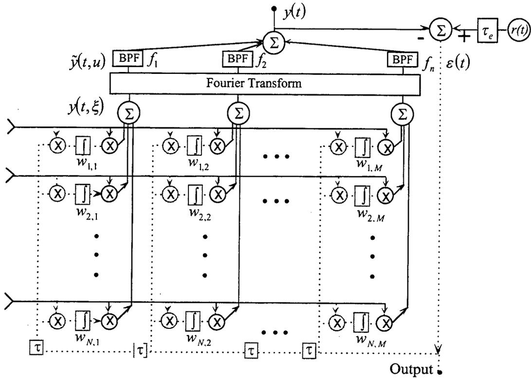
Figure 2.11. Schematic of optically implemented LMS algorithm.
