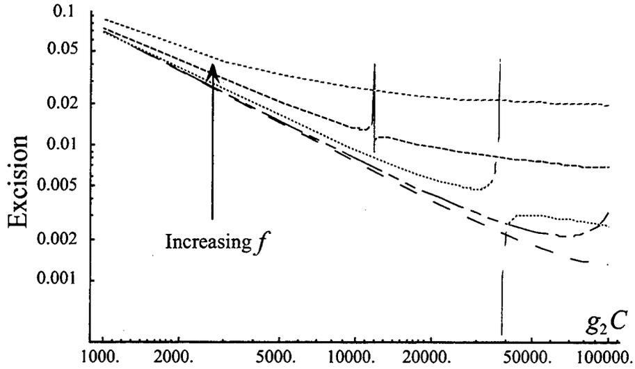
Figure 7.16. Plot of excision versus  $g_2C$ , parameterized in optical feedthrough  $f$ , which is unitless, where  $f = 10^{-3}, 10^{-2.5}, 10^{-2}, 10^{-1.5}, 10^{-1}$ . The simulation parameters were:  $A = 0.1$ ,  $R_{JE} = 0.1$ ,  $R_{MB} = 0.005$ ,  $D = 10^{-3}$ ,  $U = 10^{-5}$  all with units of volts/meter and  $r = 1$ , and  $N_{JE} = N_{MB} = 10^{-5}$ , in units of amps.
