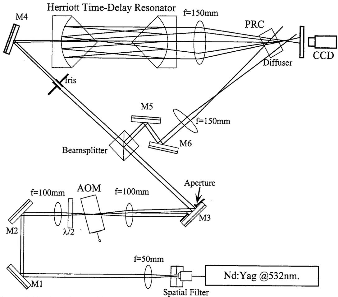
Figure 8.12. Experimental layout of Herriott time-delay resonator experiment.
