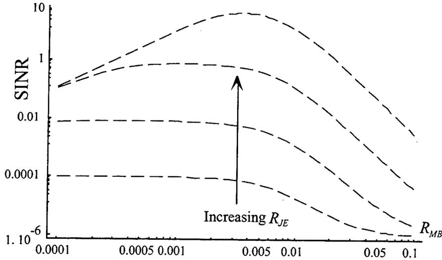
Figure 7.18. SINR versus main-beam heterodyne reference signal  $R_{MB}$ , parameterized in jammer estimate heterodyne reference signal  $R_{JE}$ , where  $R_{JE} = 10^{-4}, 10^{-3}, 10^{-2}, 10^{-1}$ . The simulation parameters were:  $A = 0.1$ ,  $U = 10^{-7}$ , with units of volts/meter,  $N_{JE} = N_{MB} = 10^{-7}$ , with units of amps,  $g_2C = 4 \times 10^4$  with units of volts/meter, and  $f = 0$ , which is unitless.
