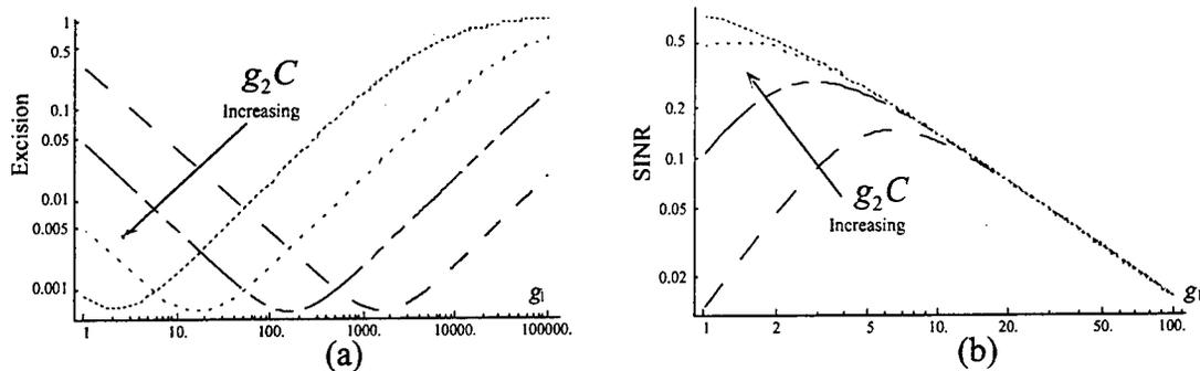
Figure 7.14. Excision versus  $g_1$  parameterized in  $g_2C$ , with units of volts/meter ( $g_2C = 10^1, 10^2, 10^3, 10^4$ ) in (a), and SINR versus  $g_1$  parameterized in  $g_2C$  ( $g_2C = 10^2, 10^{2.5}, 10^3, 10^{3.5}$ ) in (b). The simulation Parameters were:  $A = 0.1$ ,  $R_{JE} = 0.1$ ,  $R_{MB} = 0.005$ ,  $D = 10^{-3}$ ,  $U = 10^{-7}$ , all with units of volts/meter and  $r = 1$ ,  $N_{JE} = N_{MB} = 10^{-5}$  with units of amps, and  $f = 0$ , which is unitless.
