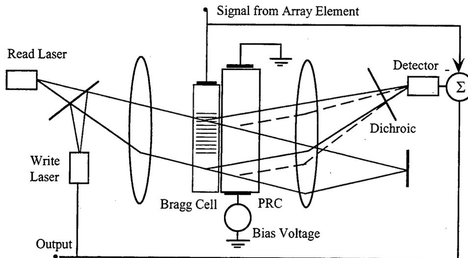
Figure 3.8. Adaptive phased-array processor (single element shown) of Montgomery, et al.<sup>13</sup>
