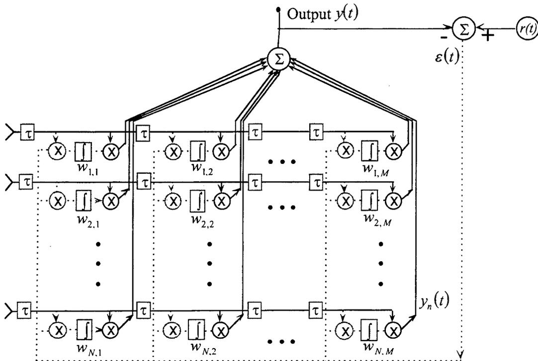
Figure 2.7. Tapped-delay line phased-array implementation of LMS architecture.
