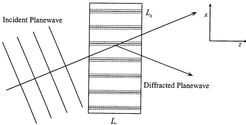
Figure 4.2. Two-dimensional holographic interaction region of dimensions  $L_x$ ,  $L_y$ , and  $L_z$ , with periodic dielectric perturbation in  $x$  direction. Incident readout plane wave produces a diffracted output wave.
