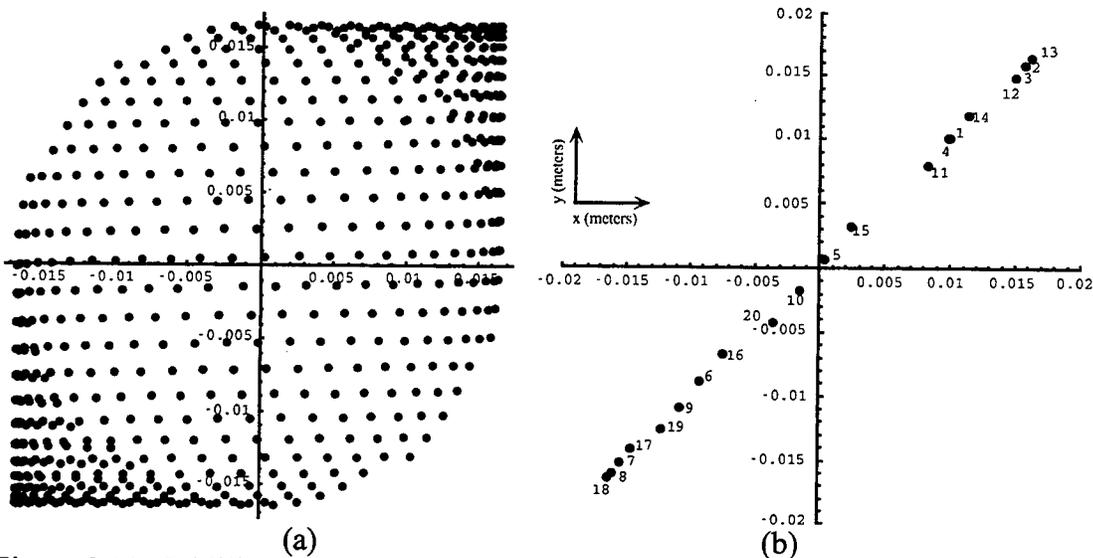
Figure 8.11. Grid-like resonator output spot pattern consisting of 650 spots in (a), and the first 20 output spots of the pattern in (b). Input parameters were  $\{d = .353, f_x = 3.72, f_y = 3.75, x_0 = .01, x' = .01, y_0 = .01, y' = .01\}$
