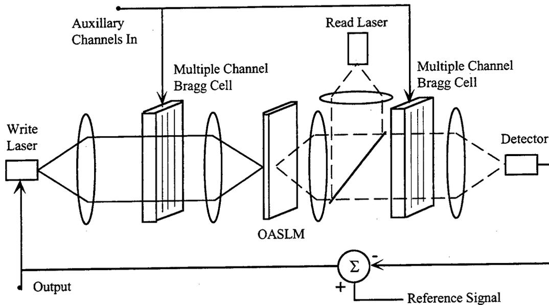
Figure 3.9. Adaptive, optical phased-array radar processor proposed by Penn, et al.<sup>16</sup>
