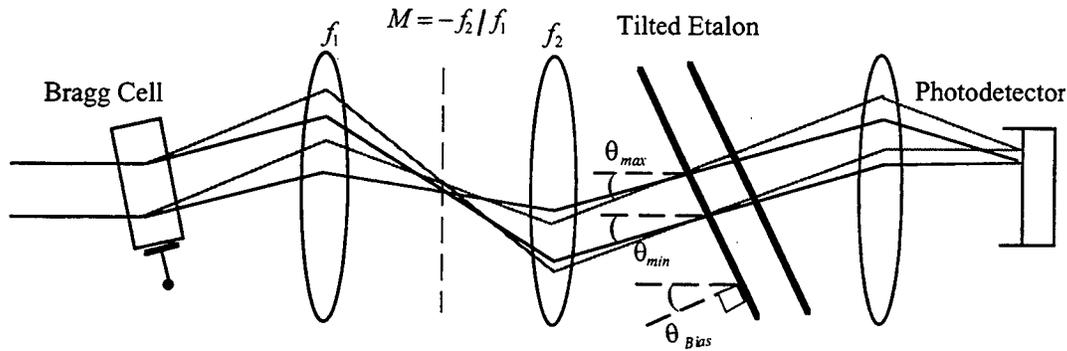
Figure 8.3. Bragg cell shown imaged with magnification  $M$  onto etalon tilted by  $\theta_{Bias}$ . The two diffracted beams from the Bragg cell incident on the etalon at  $\theta_{min}$  and  $\theta_{max}$  correspond to optical frequencies  $\nu_l = \nu_{RFcf} - \Delta f/2$  and  $\nu_u = \nu_{RFcf} + \Delta f/2$  respectively.
