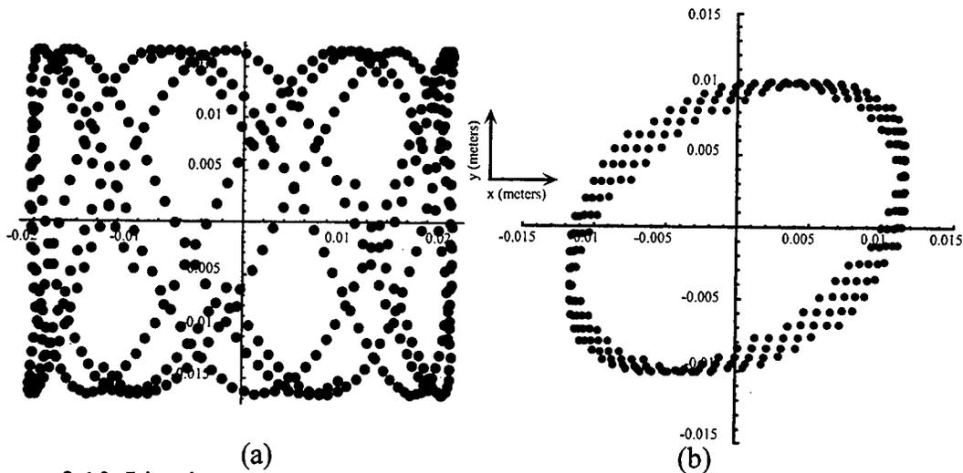
Figure 8.10. Lissajous patterns produced by astigmatic Herriott time-delay resonator. Parameters for (a) were  $\{d = .353, f_x = 3.55, f_y = 3.75, x_0 = .015, x' = .01, y_0 = .01, y' = .01\}$ , and  $\{d = .353, f_x = 3.73, f_y = 3.75, x_0 = .0001, x' = .01, y_0 = .01, y' = 0.0\}$  for (b).
