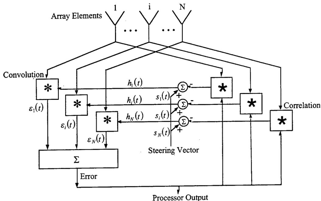
Figure 3.3. Algorithm implemented by 3-D space-time array processor
