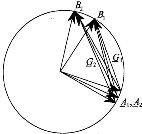
Figure 7.11. Momentum space representation of two multiple spatial mode jammers  $\underline{A}_1$  and  $\underline{A}_2$  of different temporal frequencies which share the same optical angle of arrival.
