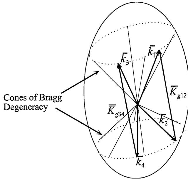
Figure 5.2. Momentum-space representation of Bragg degenerate gratings  $\bar{K}_{g12}$  and  $\bar{K}_{g34}$  formed between two independent sets of input-output  $k$ -vectors  $\bar{k}_1$  and  $\bar{k}_2$ , and  $\bar{k}_3$  and  $\bar{k}_4$ . Infinite number of possible input-output  $k$ -vector pairs map out "cones of Bragg degeneracy".
