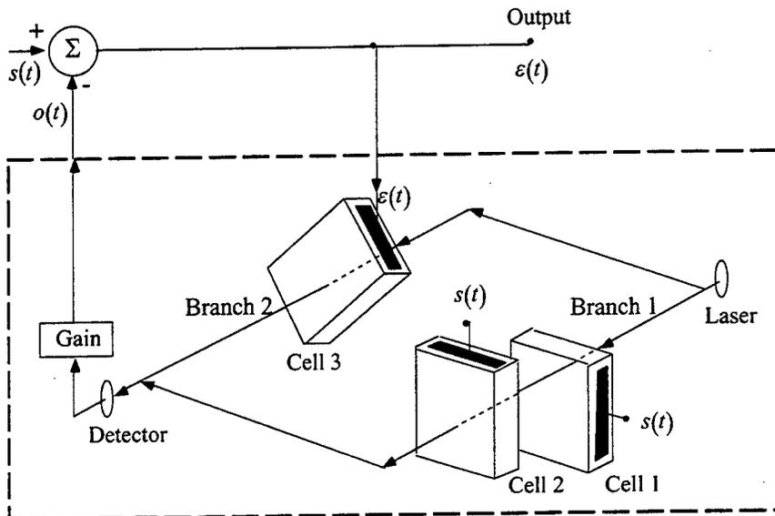
Figure 3.1. Simplified schematic of Fourier domain adaptive filter.
