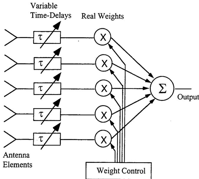
Figure 2.3. Variable time-delay architecture for broadband array processing.
