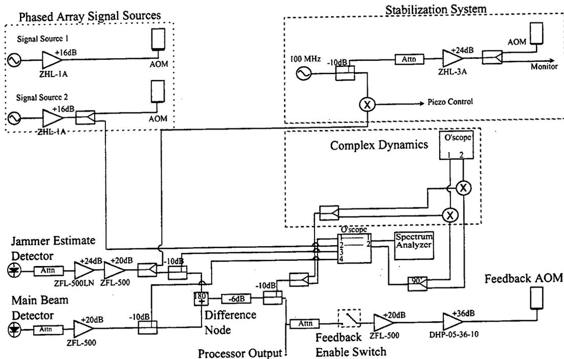
Figure 7.20. RF schematic of phased-array radar jammer-nulling processor.
