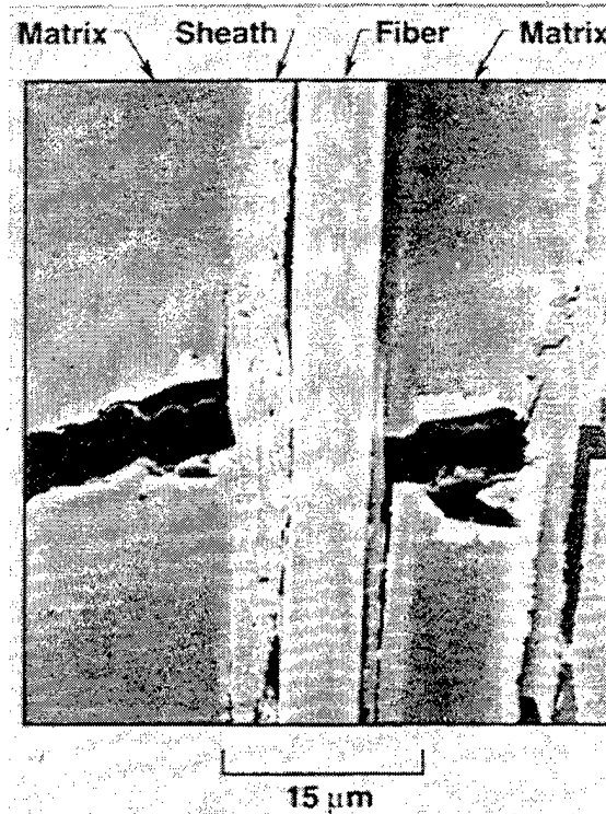
Figure 10. Crack zone showing well-defined regions of non graphitized matrix, graphitized sheath, and fiber in 2400°C heat-treated composite.
