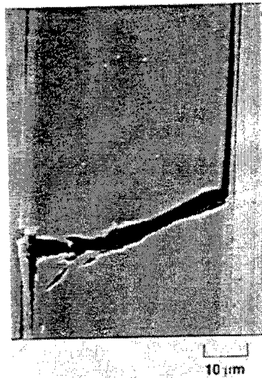
Figure 9. Short-range longitudinal intramatrix splitting in 2400°C heat-treated composite.
