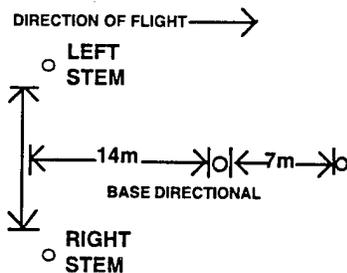
**NOTES:** The aircraft touch down point will be midpoint on the legs of the Y. If more than 1 will land in the same PZ or LZ, add 1 more light for each. For OH-, UH-, and AH-acft, mark each additional landing point with 1 light at the exact point each acft is to land. For CH-acft, mark each additional point with 2 lights placed 10mm apart and aligned in the acft direction of flight.
