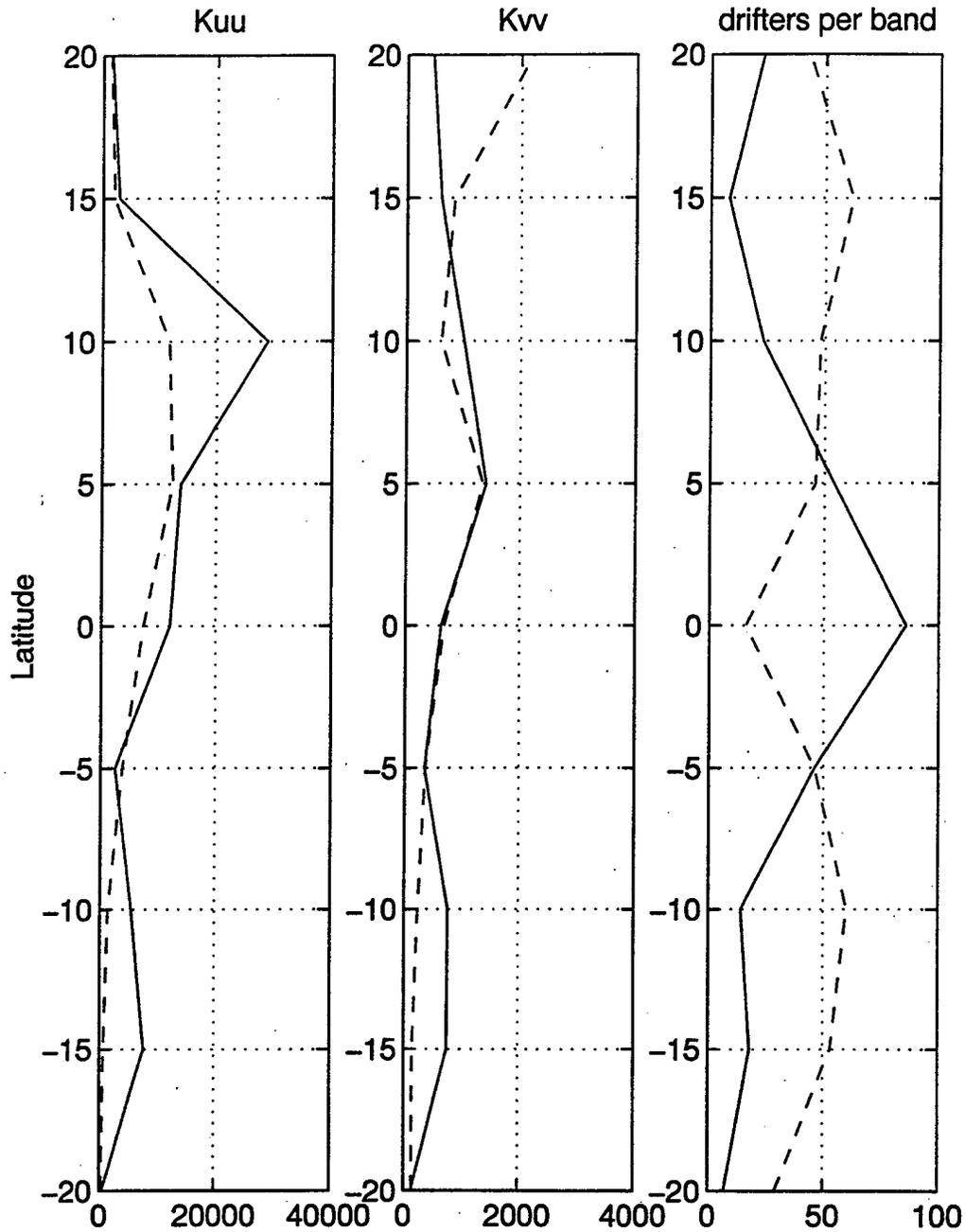
Figure 45. Meridional profiles of zonally averaged uniform (dashed line) and non-uniform (solid line) diffusivity ( $m^2 s^{-1}$ ), and number of drifters per zonal band.
