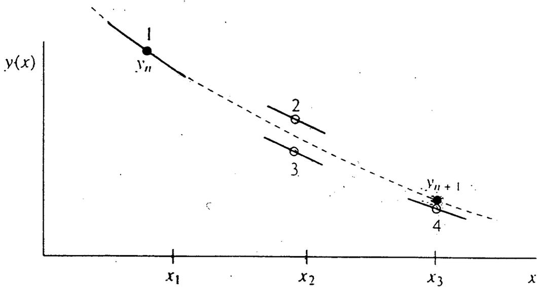
Figure 50. Fourth-order Runge-Kutta method. In each step the derivative is evaluated four times: once at the initial point, twice at trial midpoints, and once at a trial endpoint. From these derivatives the final function value (shown as a filled dot) is calculated. Figure 16.1.3 from Press et al., 1996.
