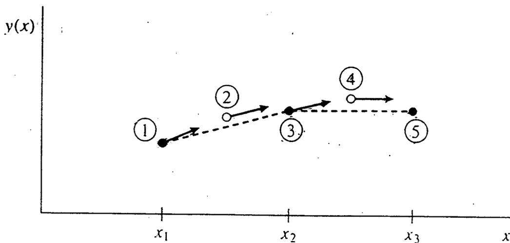
Figure 49. Midpoint method. Second-order accuracy is obtained by using the initial derivative at each step to find a point halfway across the interval, then using the midpoint derivative across the full width of the interval. In the figure, filled dots represent final function values, while open dots represent function values that are discarded once their derivatives have been calculated and used. Figure 16.1.2 from Press et al., 1996.
