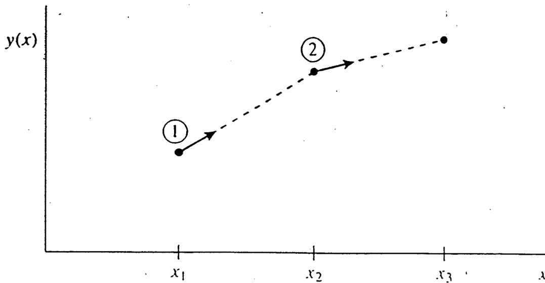
Figure 48. Euler's method. In this simplest (and least accurate) method for integrating an ODE, the derivative at the starting point of each interval is extrapolated to the next function value. The method has first-order accuracy. Figure 16.1.1 from Press et al., 1996.
