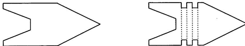
Figure 3.7 Solid armature geometry with and without grooving
