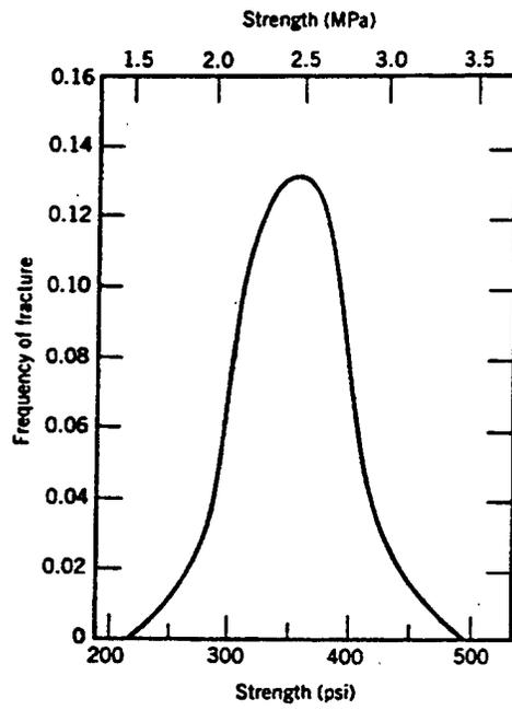
Figure 2.3 The frequency distribution of observed fracture strengths for a typical portland cement (from Ref. 5).
