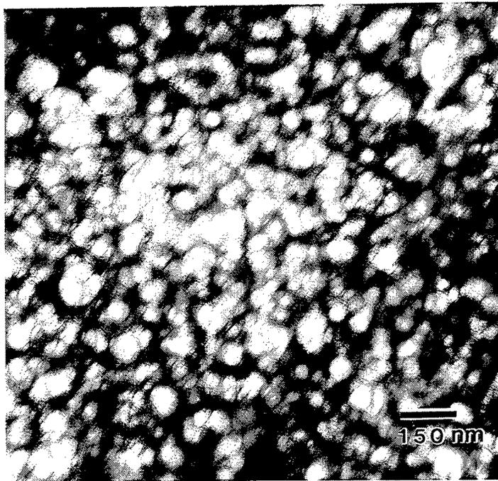
Figure 4.8 Bright-field TEM image of the C-S-H gel, showing the outer product area.
