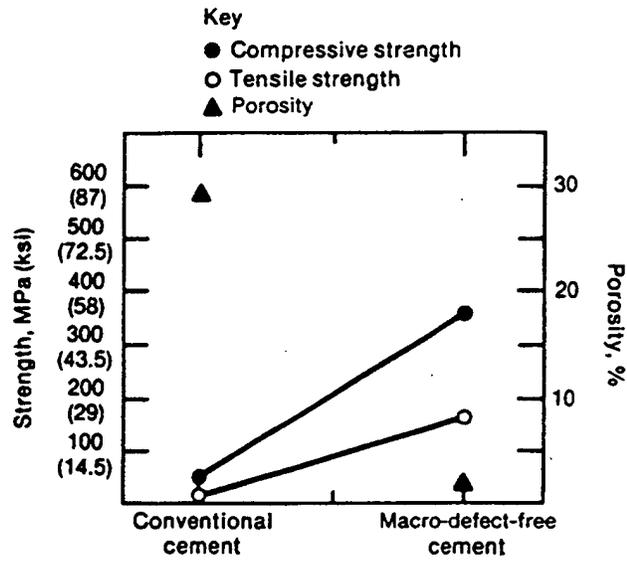
Figure 2.5 Increases in strength and decreases in porosity achieved with advanced macro-defect-free (MDF) cements (from Ref. 13).
