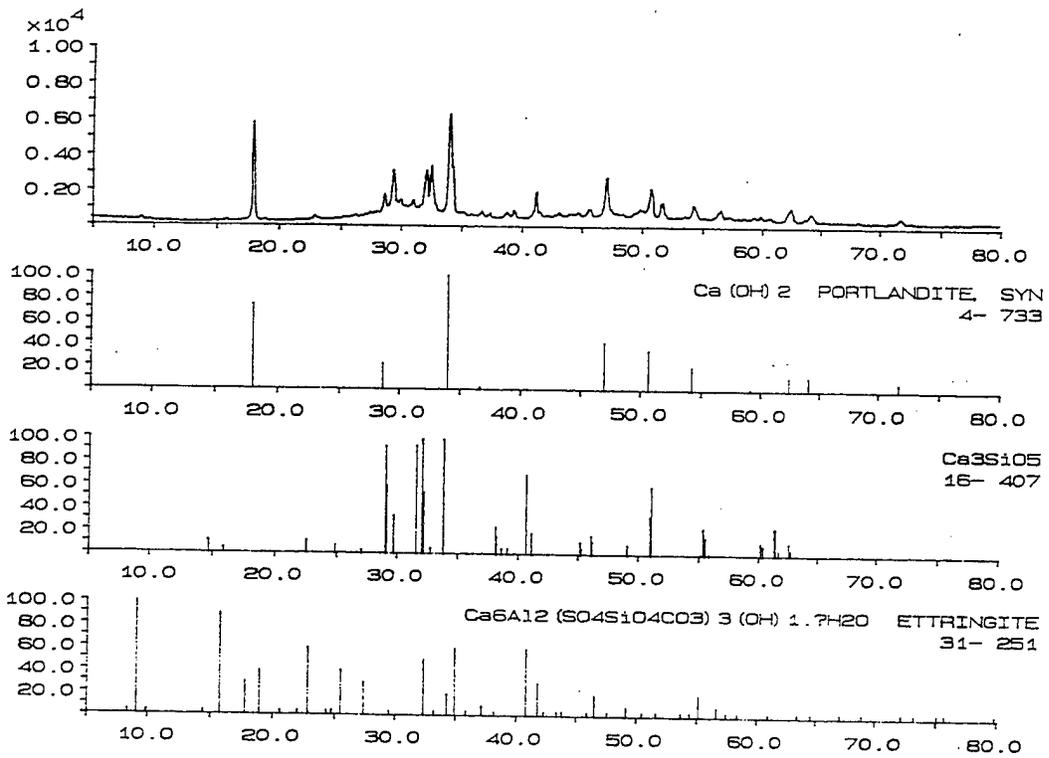
Figure 4.3 XRD line patterns of phases present in the as-received and hydrated powder sample.
