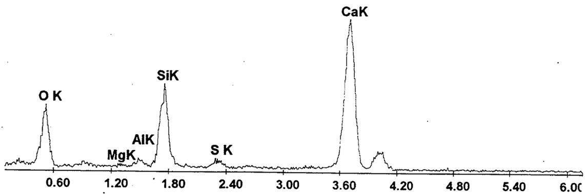
Figure 4.9 EDX spectra for the outer product C-S-H (shown in Figure 4.8) showing an average Ca:Si ratio of 1.76.
