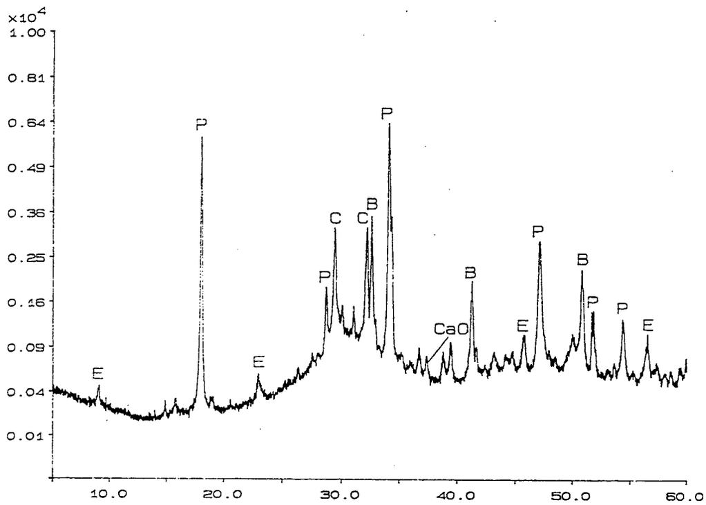
Figure 4.1 XRD Pattern of the as-received and hydrated powder sample showing crystalline phases E=Ettringite, P=Portlandite, C=C<sub>3</sub>S, B=β-C<sub>2</sub>S, and CaO.
