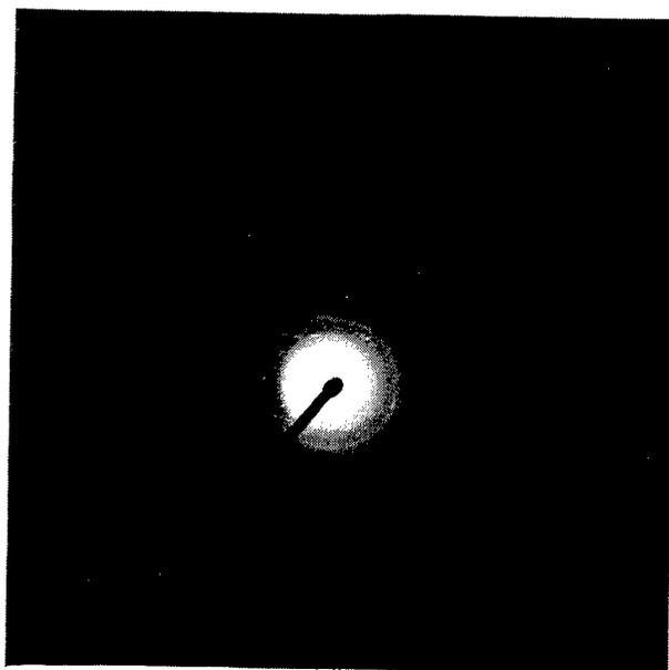
Figure 4.17 SAED pattern taken from a randomly selected region within the C-S-H gel. The pattern clearly indicates the presence of diffuse rings.
