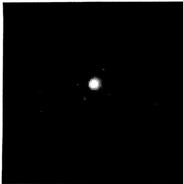
Figure 4.10 SAED pattern of the outer C-S-H gel region (shown in Figure 4.8) showing the presence of nanocrystallites regions coexisting with the C-S-H phase.
