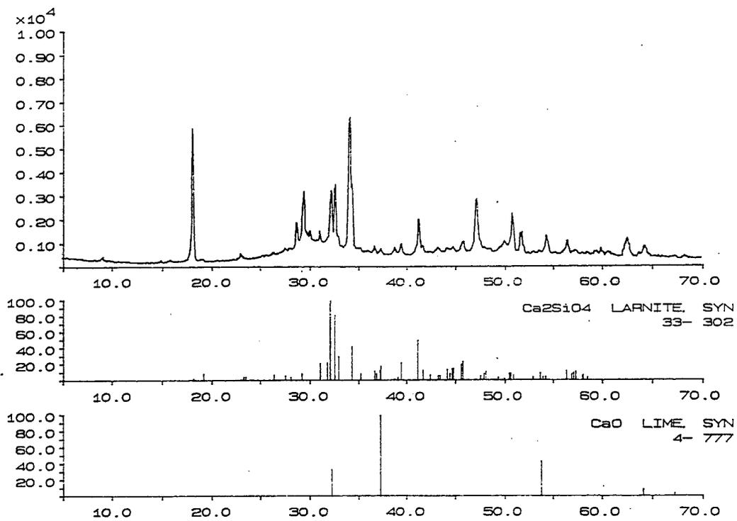
Figure 4.4 XRD line patterns of phases present in the as-received and hydrated powder sample.
