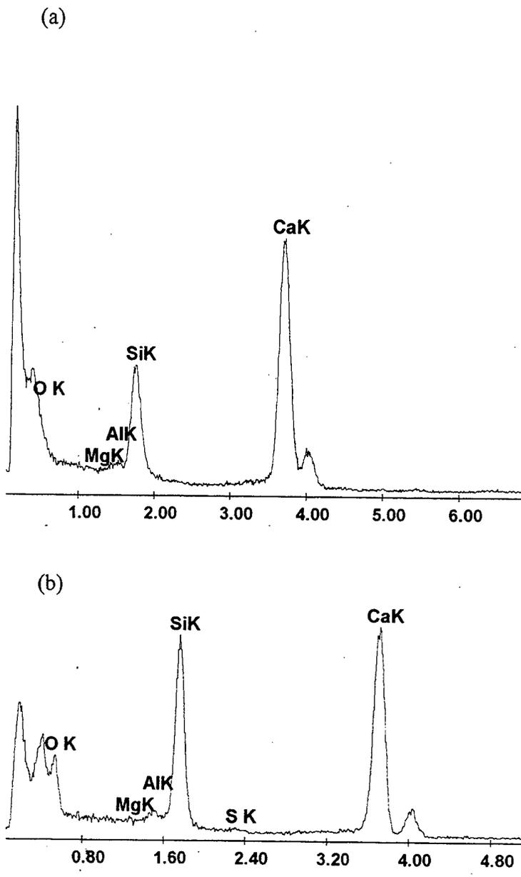
Figure 4.15 (a) EDX spectra for the unhydrated  $\beta$ -C<sub>2</sub>S and (b) EDX spectra for the C-S-H phase (shown in Figure 4.14).
