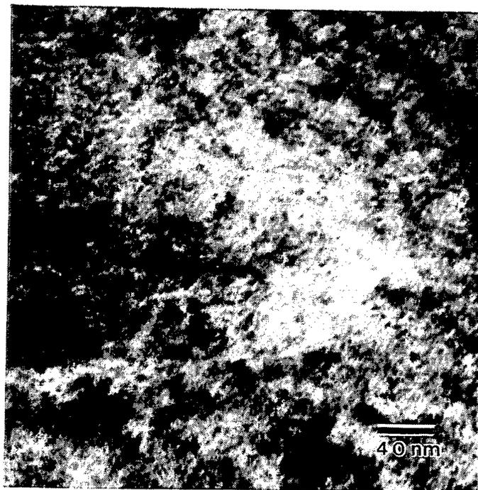
Figure 4.11 Bright-field TEM image of the inner product region of the C-S-H gel.
