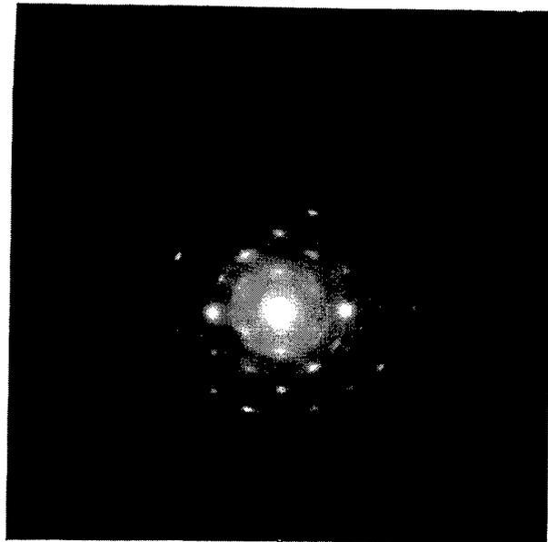
Figure 4.20 SAED for the CH region (shown in Figure 4.18). The electron beam direction is  $[110]$ .
