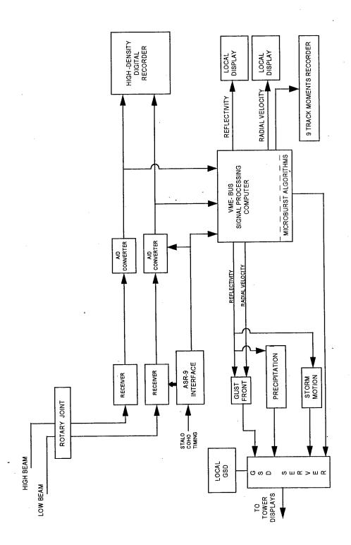
FIGURE 3.1-2. TRDF PROTOTYPE WSP - PHASE I DEMVAL
