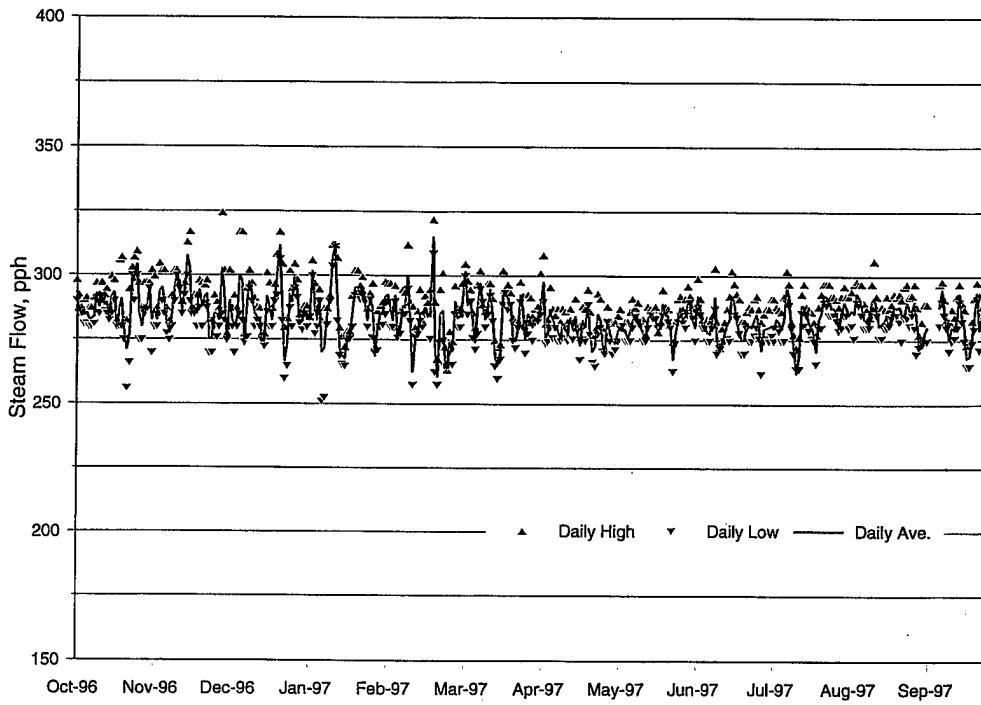
FIGURE 3. Well 4H-4 Steam Flow, October 1996 through September 1997.
