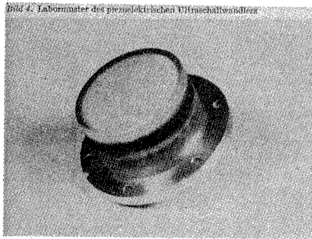
Figure 4. Laboratory model of the piezoelectric ultrasonic transducer
