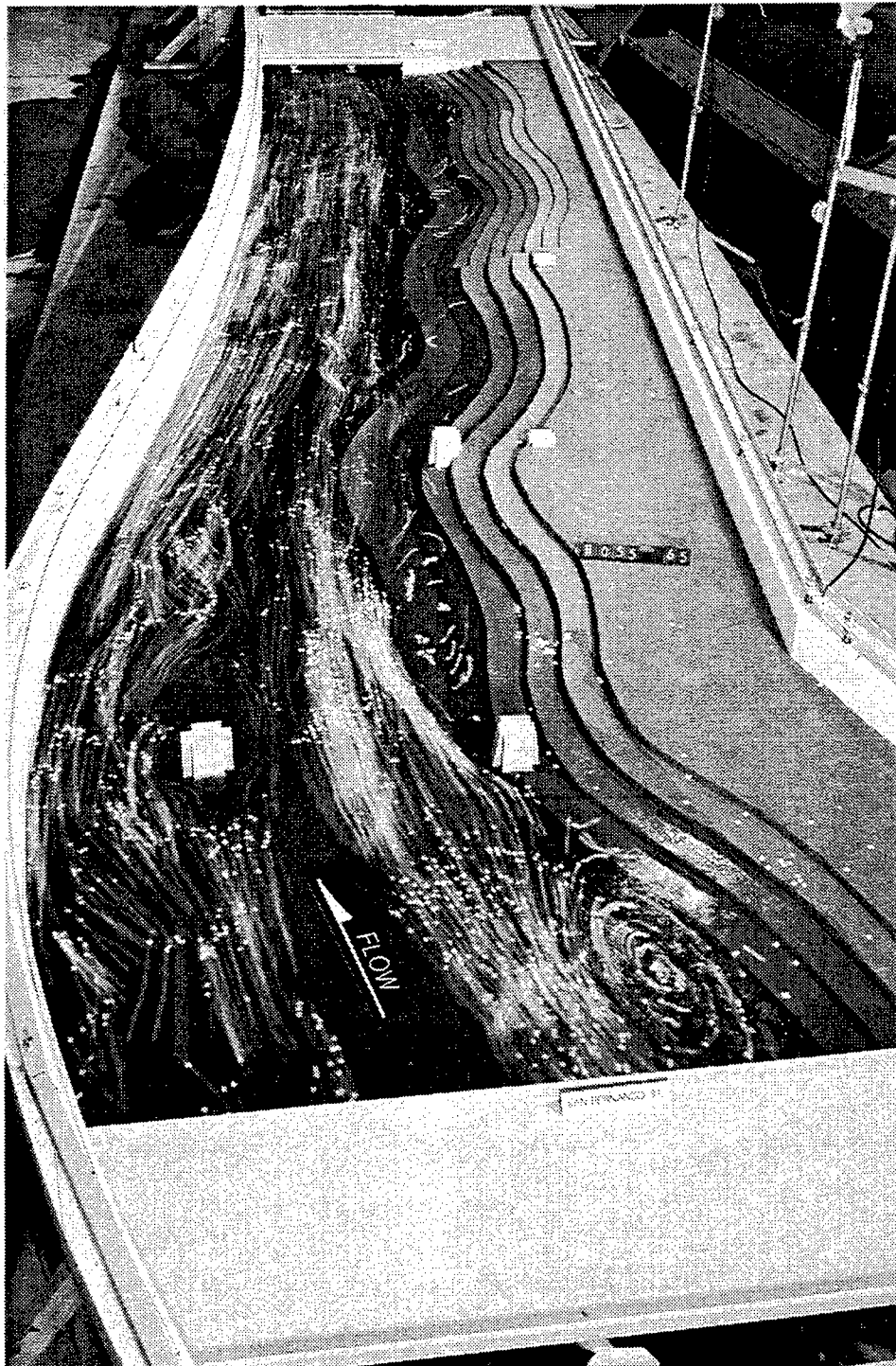
Photo 15. Looking downstream from sta 163+00 at flow conditions in the Guadalupe River with the type 1 design, existing conditions, and a discharge of 9,100 cfs and confetti placed on the surface to highlight surface patterns
