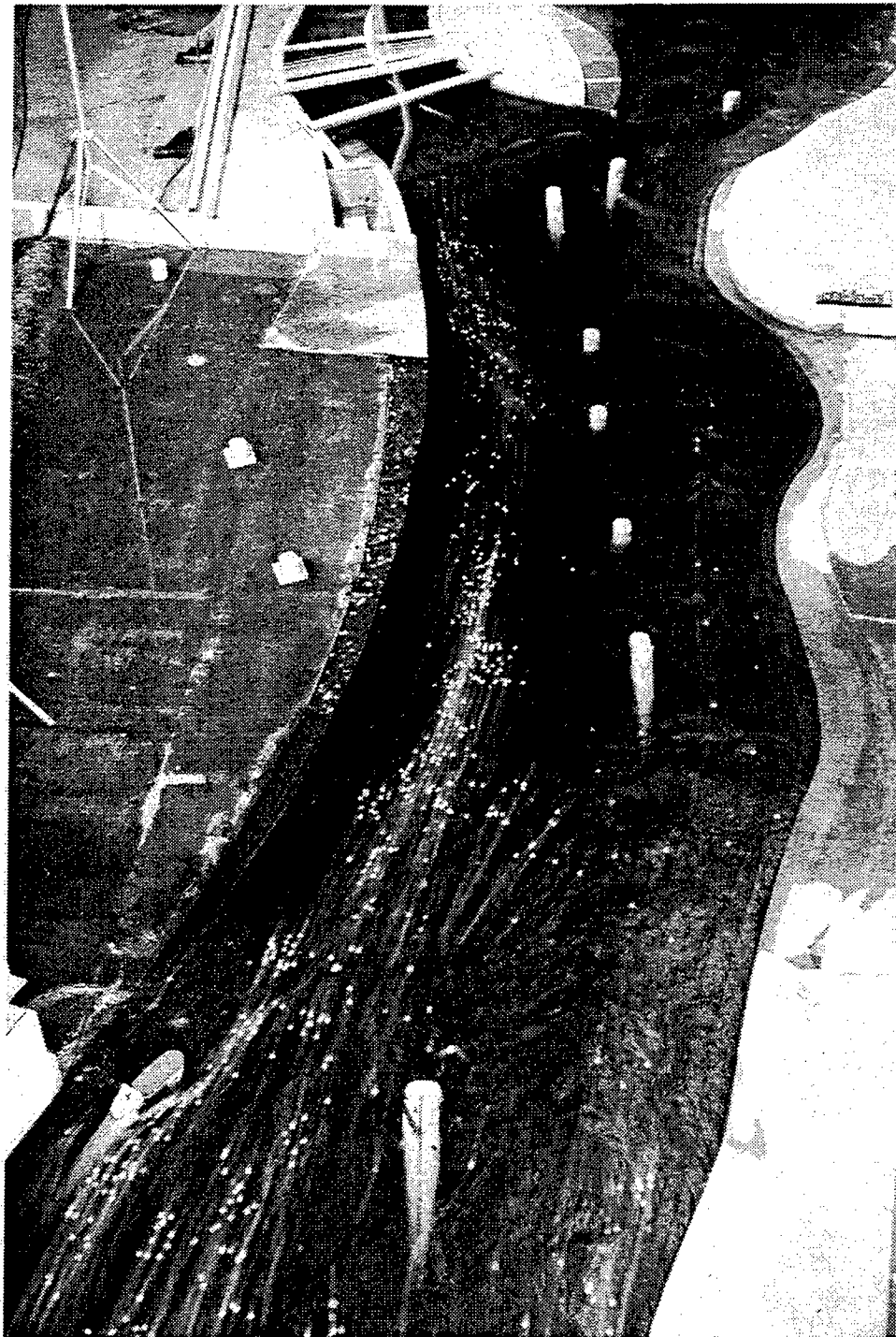
Photo 22. Looking downstream at flow conditions in the upstream channel between sta 199+00 and the entrance to the bypass culvert with the type 19 upstream channel, type 16 bypass entrance, and type 8 pier extensions with future conditions and a discharge of 14,600 cfs
