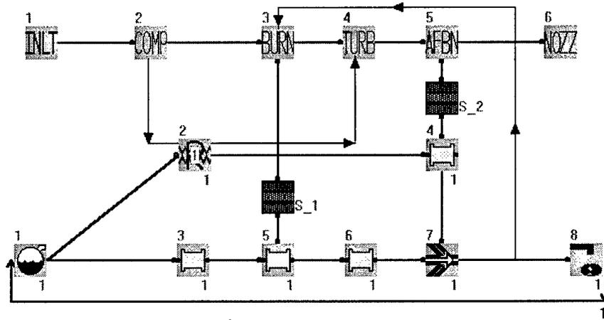
Figure 8. VITMAC Generic Turbojet Engine Cooling Network
