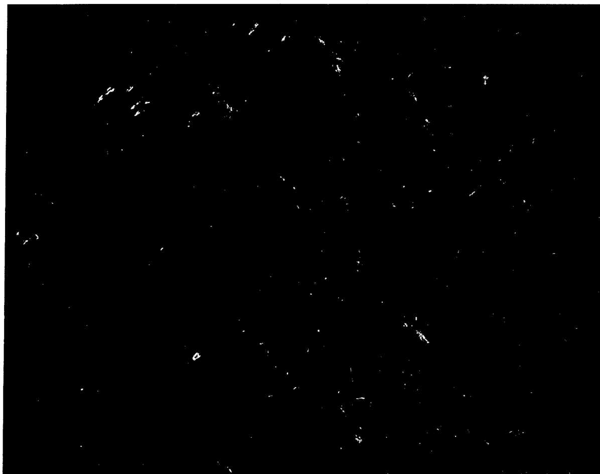
Fig. 1. Photograph of a Quartz Substrate Before Cleaning as Observed Through a Dark-Field Microscope at 400X Magnification. The field of view is 0.5 mm.
