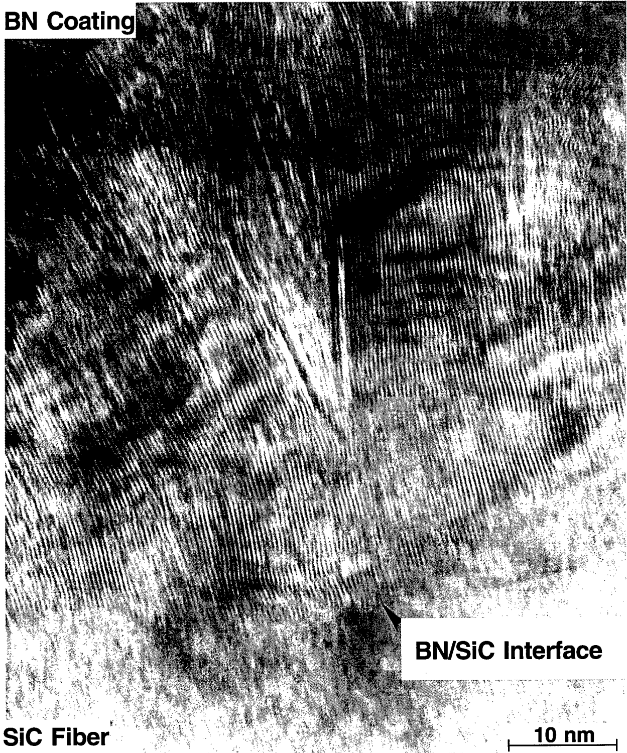
Figure 40. HRTEM micrograph showing the BN coating/SiC fiber interface and the lattice planes of the BN coating. The BN basal planes grow with an orientation that is mostly perpendicular to the long axis of the SiC fiber.
