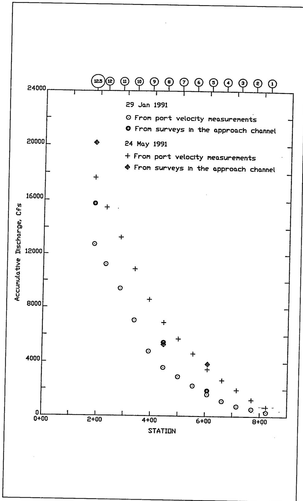
Figure 14. Accumulative discharge through the guard wall ports
