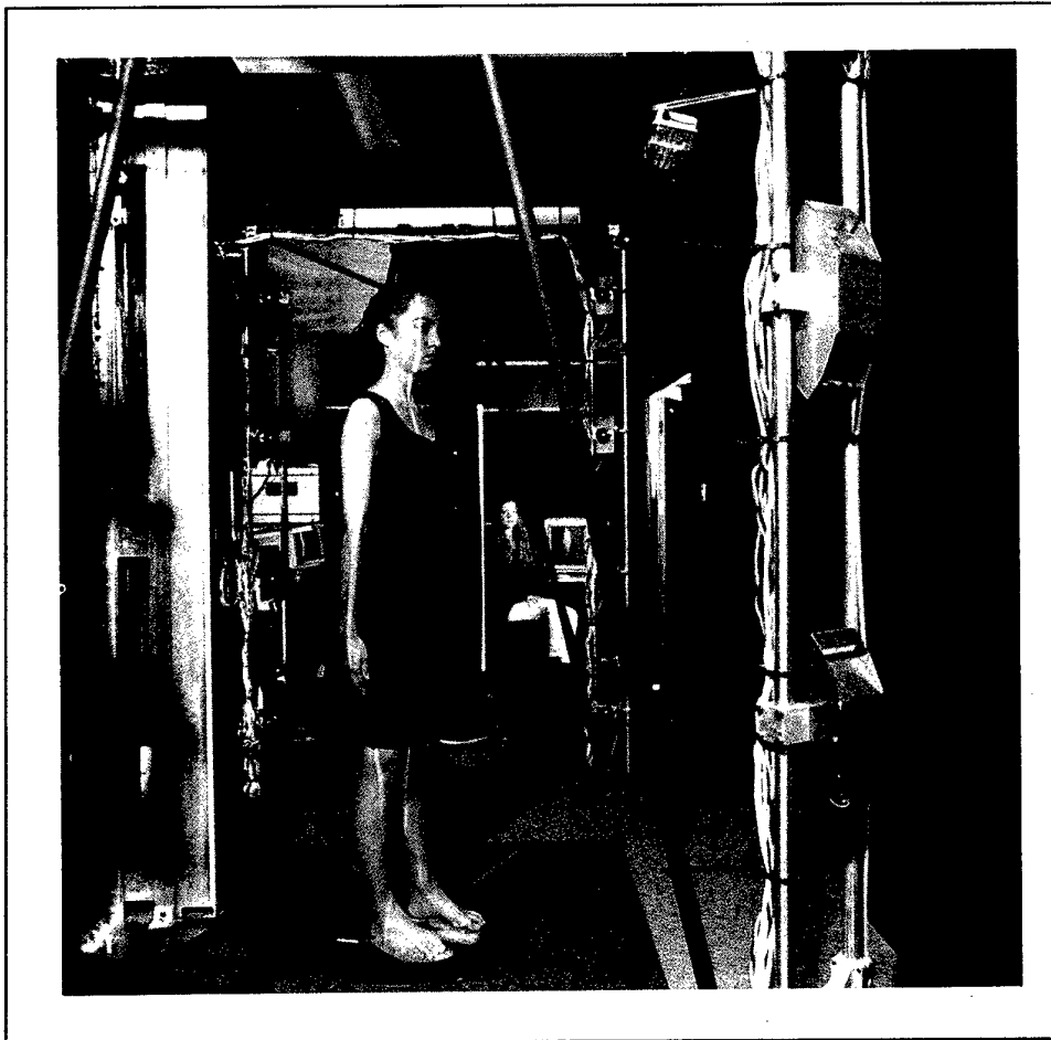
Figure 2-1. A subject being scanned in the LASS experimental rig. The narrow vertical slits of the projector light are falling on the body contours.
