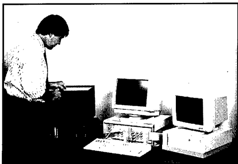
■ A Surface/Interface employee placing a sample in the company's BEESBox™, a commercially available BEEM system manufactured through a license from JPL.
