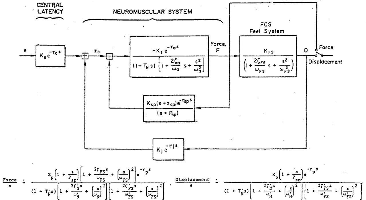
Fig.1.14. Pilot Closed-Loop Limb-Actuation With Feel System Dynamics
