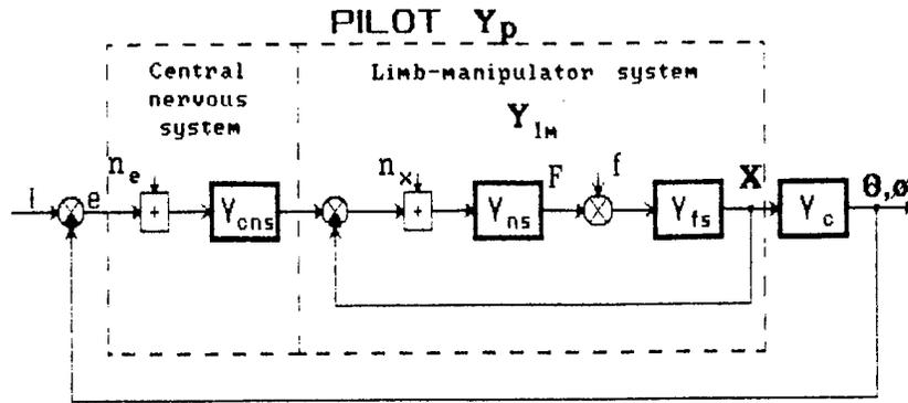
Fig.1.13 Diagram of pilot-aircraft system including closed loop limb-manipulator system.
