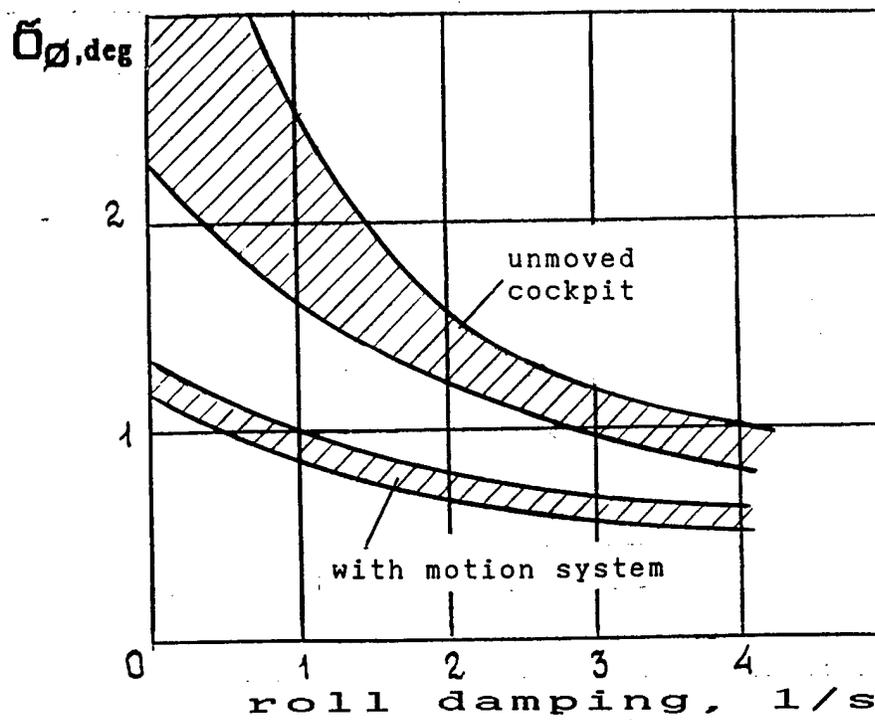
Fig.1.9. Motion Cues Influence on Roll Stabilization Precision
