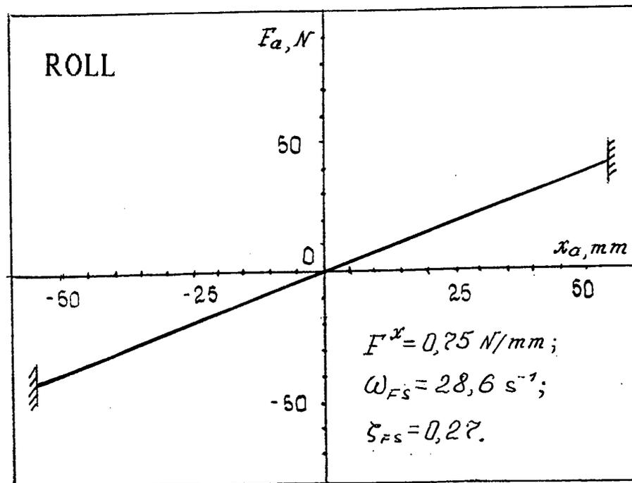
Fig.1.6. Side Stick Feel System Characteristics
