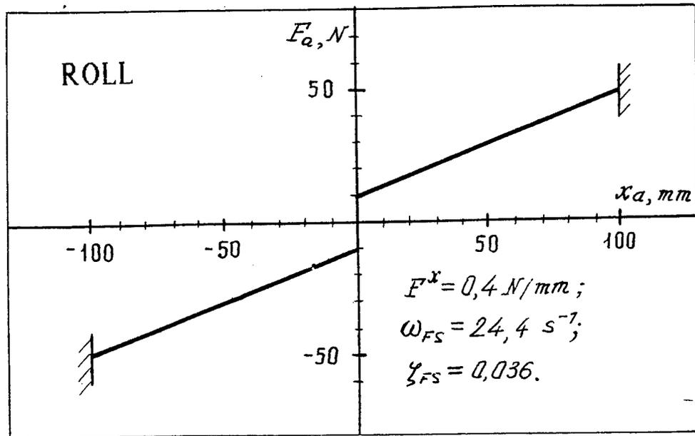
Fig.1.5. Central Stick Feel System Characteristics
