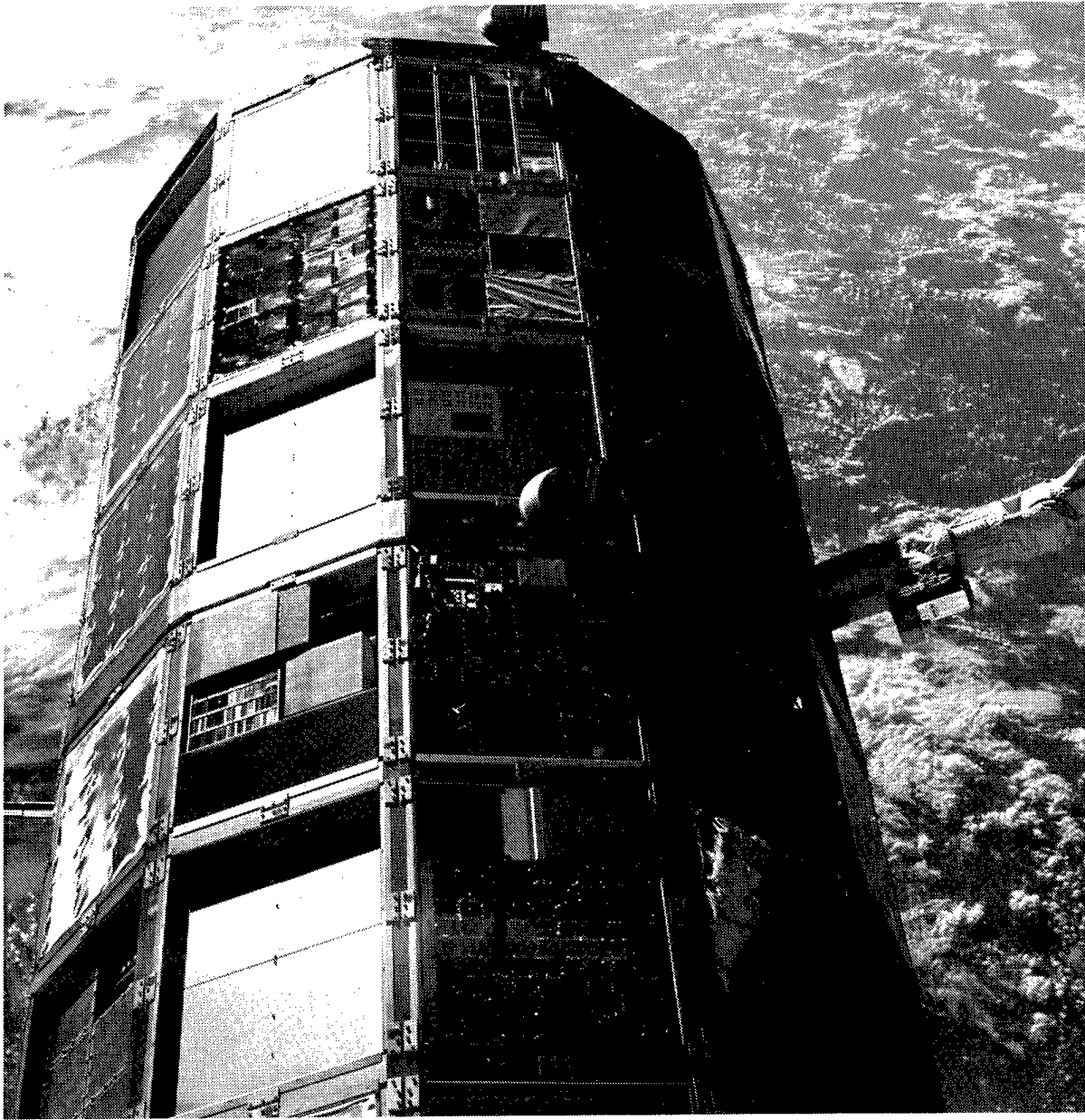
Figure 2.1-3. Photograph Taken During LDEF Retrieval Showing Trays/Experiments Mounted to LDEF
