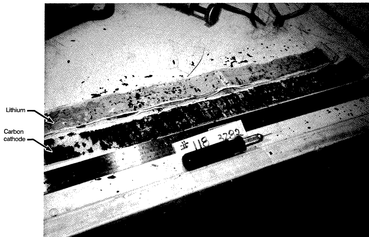
Figure 4.2.3.1-7. \text{LiSO}_2 Cell Components—Flight Battery With a 35% State of Charge
