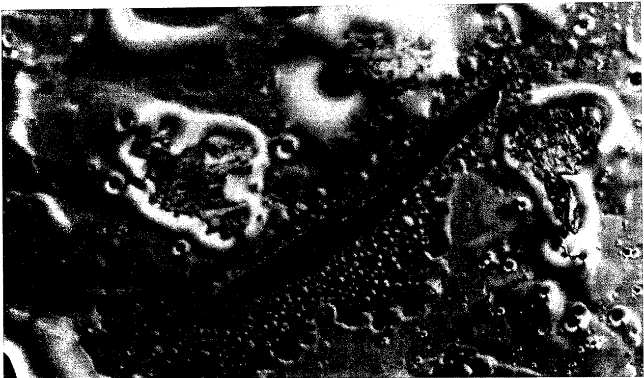
Figure 4.4.2.2-2. Contamination on Laser Mirror Photographed at SAEF-2 at the Nomarski Microscope Workstation. (Courtesy of E. R. Crutcher)
