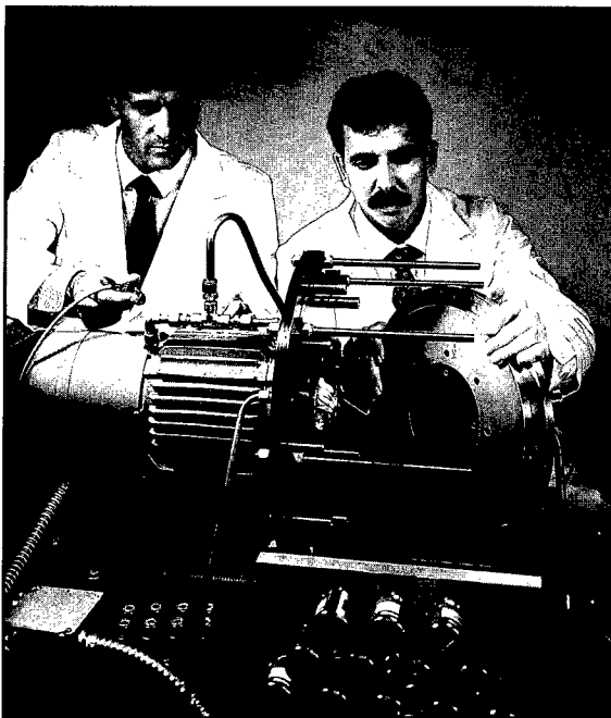
Two researchers from Mainstream Engineering Corporation assembling their high-speed compressor, which could replace compressors in any refrigerator or air conditioner on the market. Mainstream is developing the compressor under an SDI SBIR Phase II contract.
