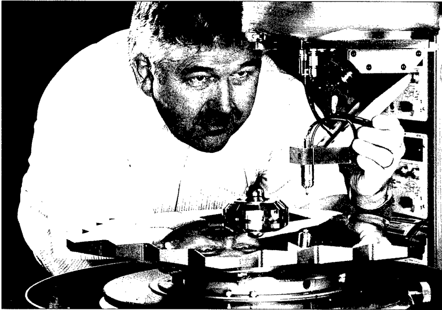
A researcher working on the large optics diamond turning machine. Originally built at Lawrence Livermore National Laboratory to produce the high-power optics for SDI's Alpha laser, the diamond turning machine also has been used to produce high-precision optics for telescopes.
