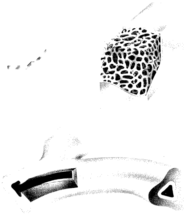
An artist's conception of Ultramet's carbon foams. The top drawing shows the entire foam structure, while the bottom drawing shows an individual fiber.
