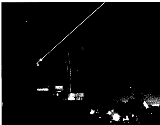
A laser beacon used in adaptive optics. Lasers are fired 90 kilometers into the earth's atmosphere to produce an artificial reference star. By measuring the distortion when atmospheric particles reflect the light back to the earth, researchers can compensate for distortion in images from space.
