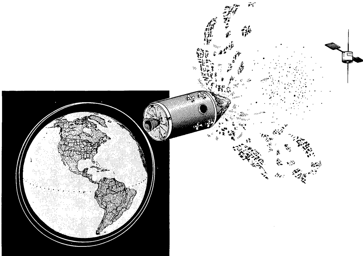
Figure 6.10. CIS Co-Orbital ASAT Flight Profile and Engagement.
