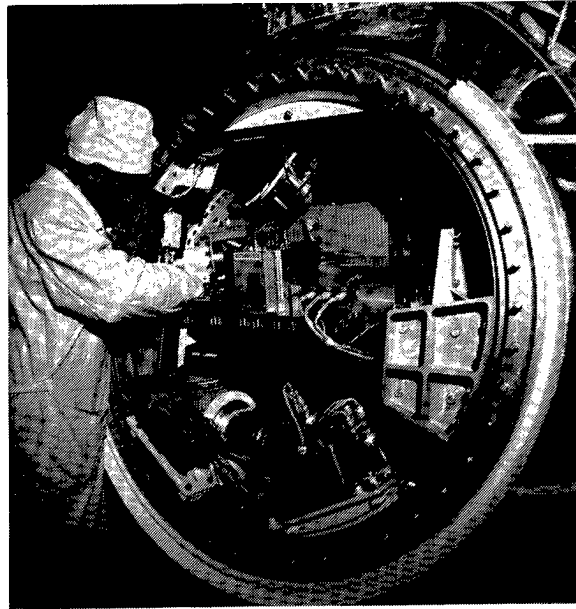
Figure 4.88. Installing Microgravity Experiments in Resurs-F1 Return Capsule.
