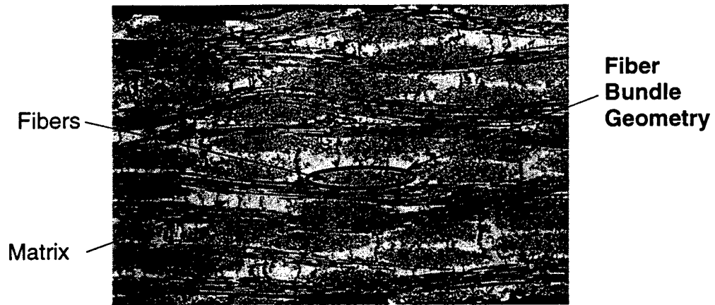
Figure 8. Micrograph of a planar weave composite.
