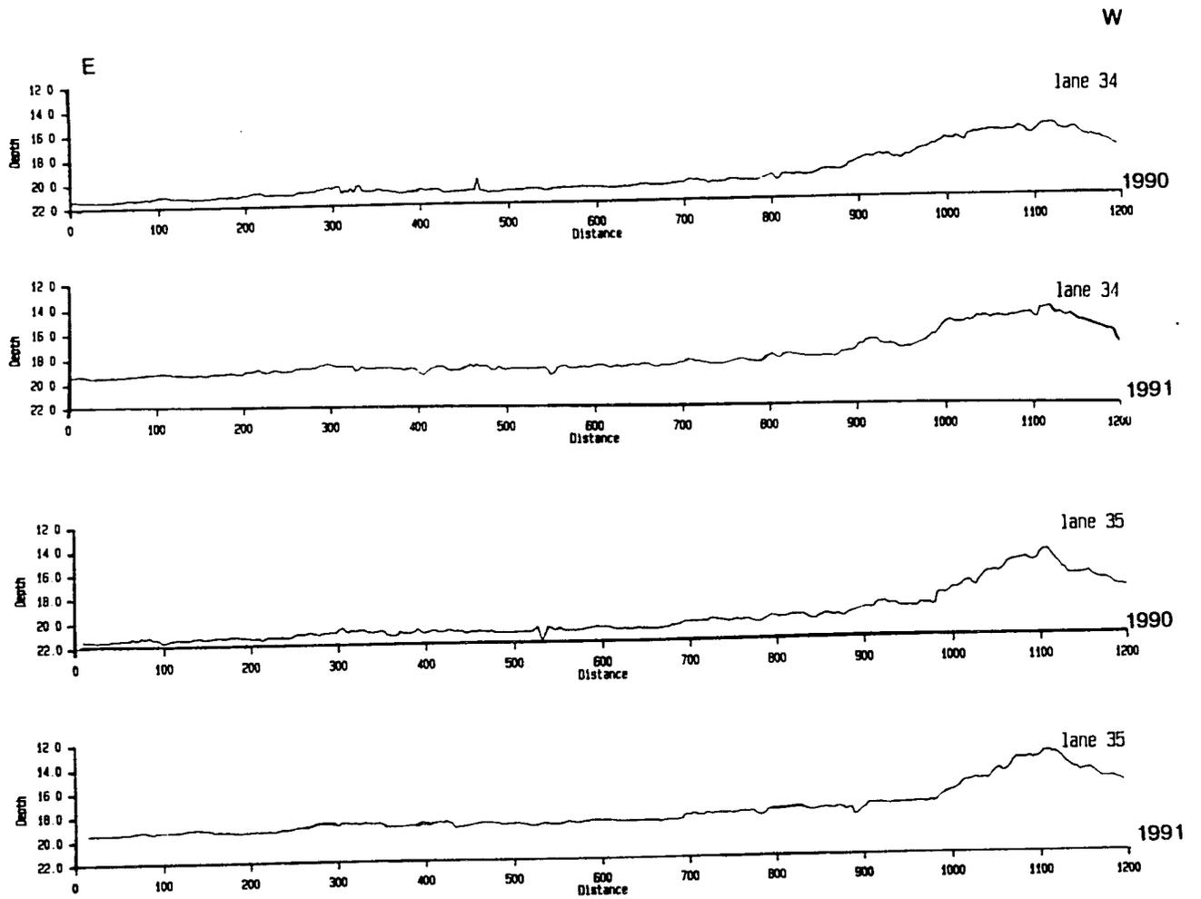
Figure 3-4. Profile plot of survey lanes 34 and 35, CLIS bathymetric surveys, 1990 and 1991
