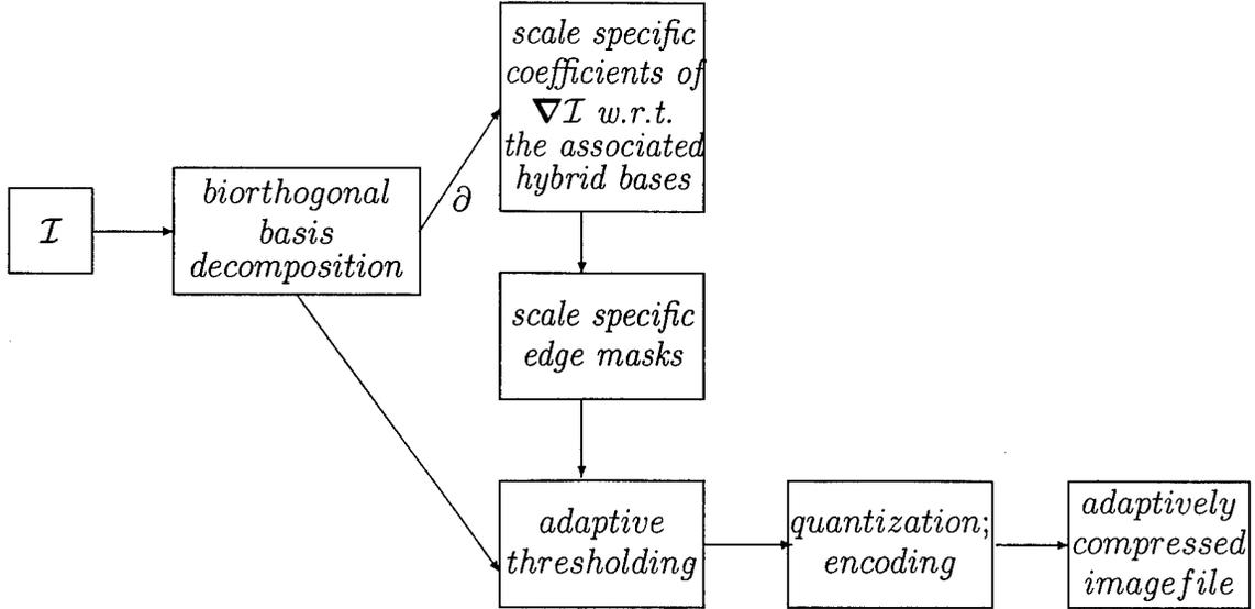
**Fig.4:** Schematic diagram of the modified adaptive compression scheme, using a smooth, compactly supported biorthogonal wavelet decomposition of the image  $\mathcal{I}$ .  $\partial$  is the set of almost-diagonal linear transformations in Fig. 3, applied at selected scales to compute the gradient wavelet coefficients.
