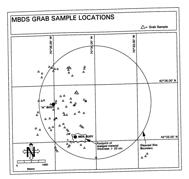
Figure 1-2. Location of grab samples taken at MBDS, June 1989. MDA buoy is the active disposal point; "A" buoy was an historic disposal location. Dredged material footprint from bathymetric survey of 1990 (Germano et al. 1994).
