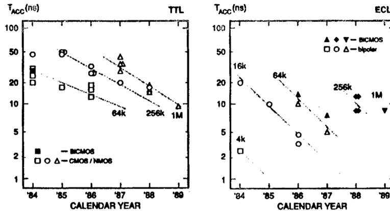
Figure 1. Transition of Access Time of High-Speed SRAM
