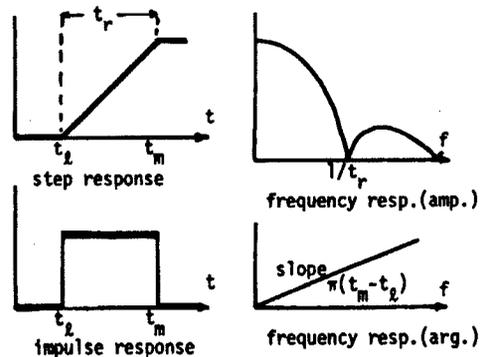
Figure 2. Frequency Characteristics and Time Response of Traveling-Wave-Type Modulator
