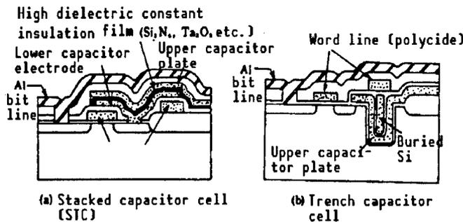
Figure 4. High Integration Density Memory Cells Built Using Three-Dimensional Cell Structures
