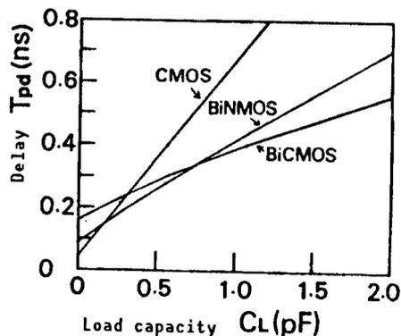
Figure 4. Relationship Between Gate Delay Time and Load Capacities of Three Types of Invertors (CMOS, Bi-nMOS, BiCMOS) (calculated result)
