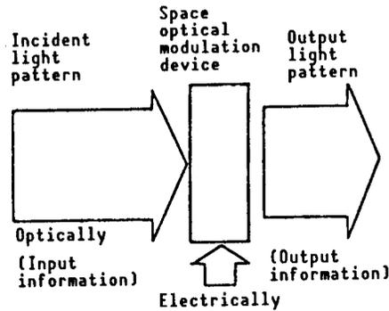
Figure 1. Operation Concept of Space Optical Modulation Device
