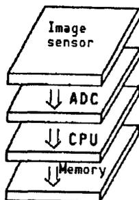
Figure 5. Simplified Construction of a Parallel Image Processor
