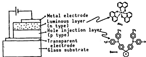
Figure 1. Basic Sectional Structure of Organic Thin Film EL Device
