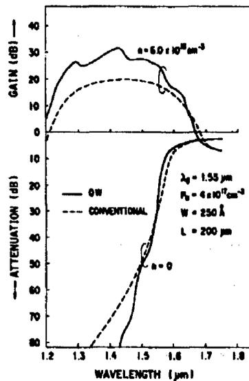
Figure 3. Characteristics of Isolation Wavelength of LD Optical SW Which Can Be Operated in Wide Wavelength Regions<sup>4</sup>
