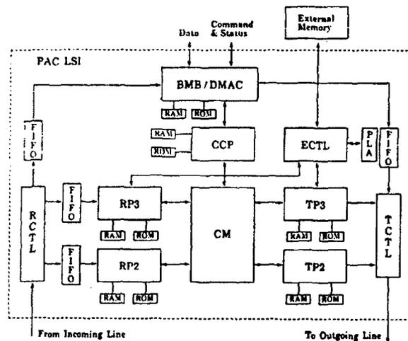
Figure 6. Block Diagram of VLSI for High-Speed Packet Communication Control
