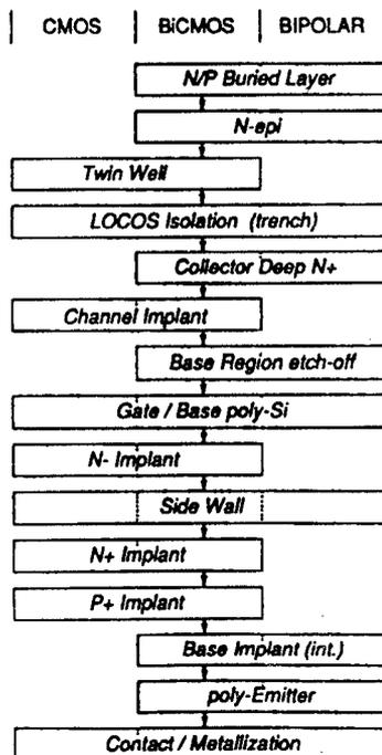
Figure 1. Flowchart of 0.8- $\mu\text{m}$  Level Double Polysilicon BiCMOS Process
