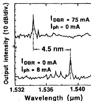
Figure 8. Example of Output Wavelength Spectra
