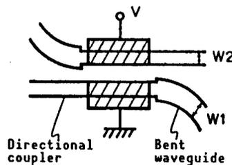
Figure 7. Bent Waveguide Structure
