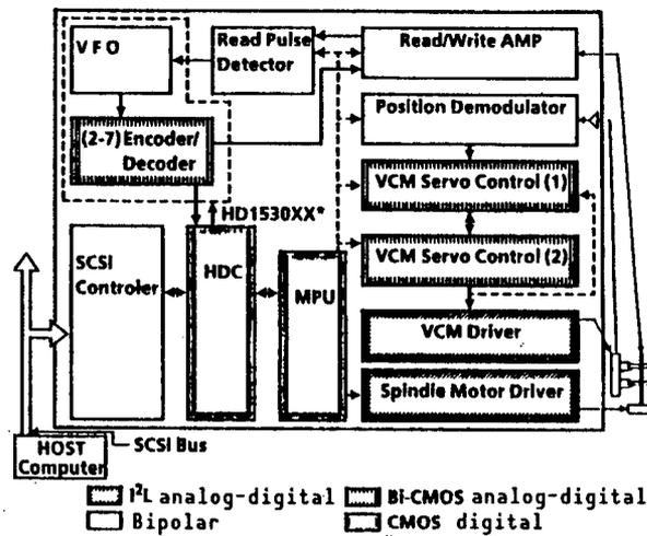
Figure 6. LSI Configuration of a Hard Disk Drive System
