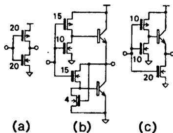
Figure 3. Three Types of Invertor Configurations
