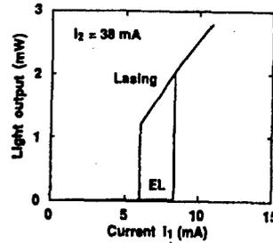
Figure 2. Example of Current-Optical Output Characteristics
