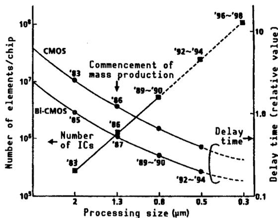
Figure 1. Trend in Number of Integrated Elements and Delay Time
