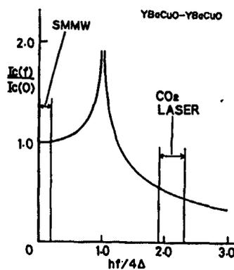
Figure 2. Frequency Dependency of Josephson Current in an Nb-YBaCuO Junction
