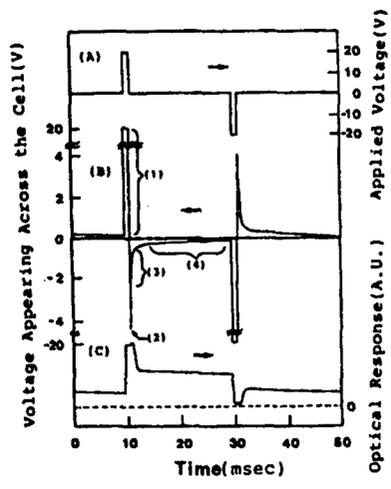
Figure 7. Observation of SSFLCD Both Cell Ends Voltage
