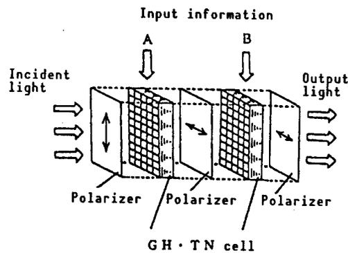
Figure 3. Parallel Optical Operation by GH·TN Liquid Crystal
