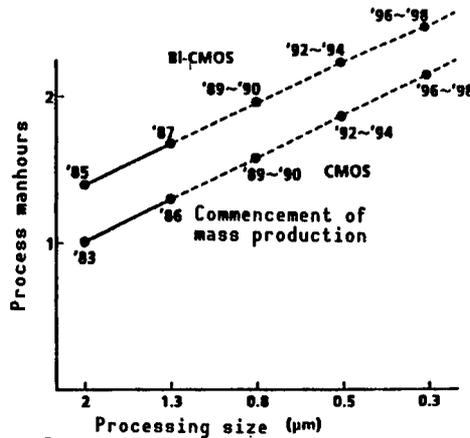
Figure 9. Trend of Process Manhours With Processing Size
