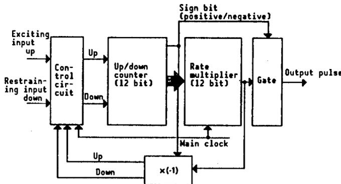
Figure 3. Circuit Construction of Hardware Representing a Neural Cell Body
