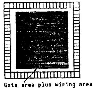
Figure 7. Channelless Gate Array
