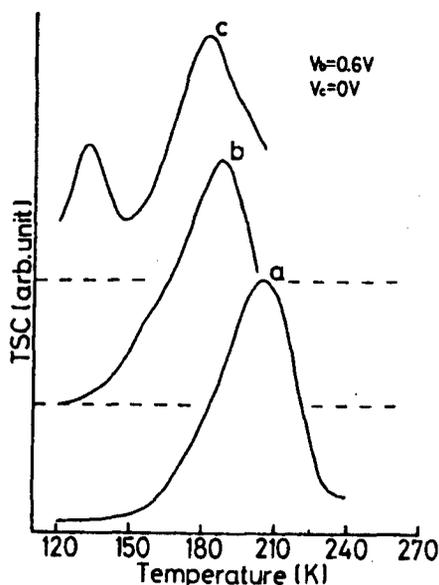
Figure 3. TSC of TCNQ Doped Sample
