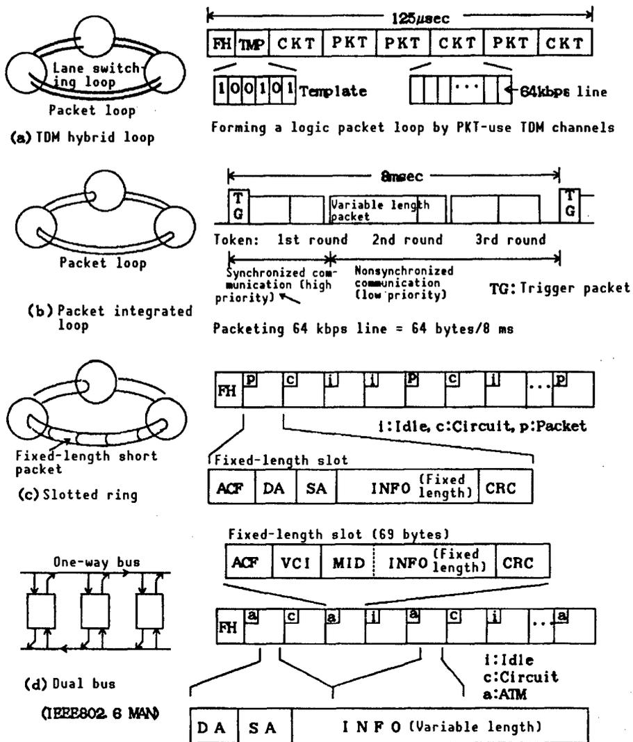
Figure 2. Integrated Trunk LAN/MAN Access System
