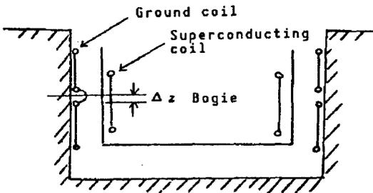
Figure 2. Arrangement Method of Coil to Side Wall
