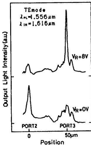
Figure 11. Change in Near Field Patterns Against Electric Field Impression<sup>7</sup>
