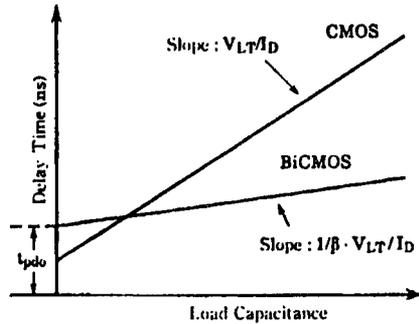
$$t_{pd} = t_o + \frac{1}{\beta} \cdot \frac{V_{LT}}{I_D} \cdot C_L; \quad \beta = \frac{f_T(I_C)}{f}$$
