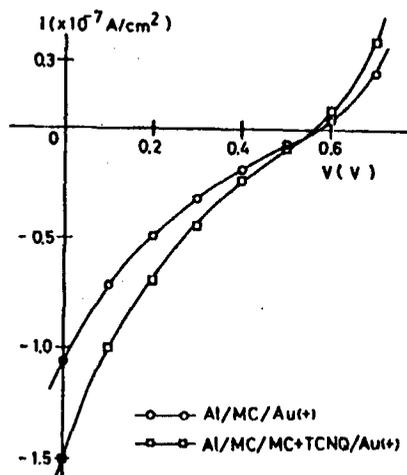
Figure 5. Current-Voltage (I-V) Characteristic Under Light Irradiation
