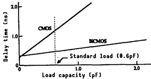
Figure 6. Delay Time Property of BiCMOS Gate
