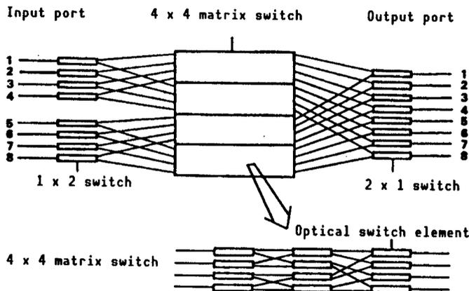
Figure 5. Configuration of  $\text{LiNbO}_3$  8 x 8 Matrix Optical Switch Not Dependent on Light Polarization
