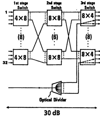
Figure 1. 3-Stage 32-Line Spatial Division Optical Exchanger (Including distribution mode circuits)
