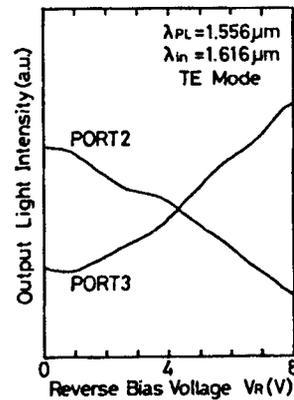
Figure 12. Change in Optical Output of Each Port by Electric Field Impression<sup>7</sup>
