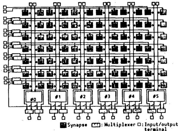
Figure 4. Circuit Construction of a Digital Neurochip
