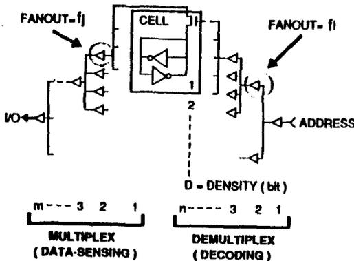
Figure 5. Access Time Critical Path of SRAM
