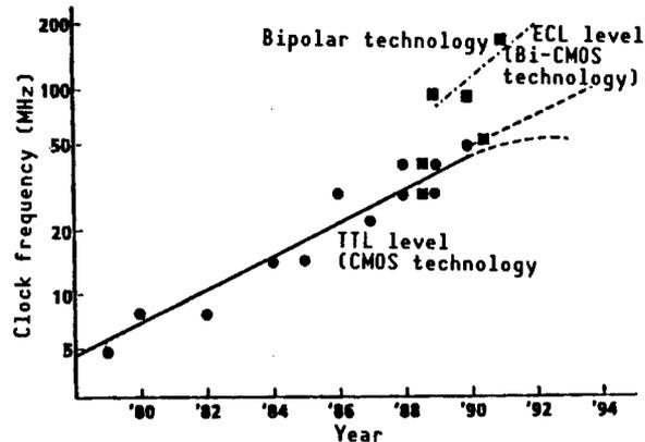
Figure 3. Improved Operating Frequency of Microprocessors
