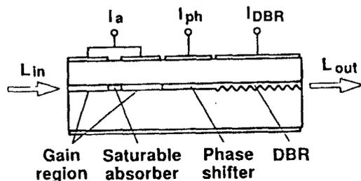
Figure 7. Basic Structure of Wavelength Converting Element
