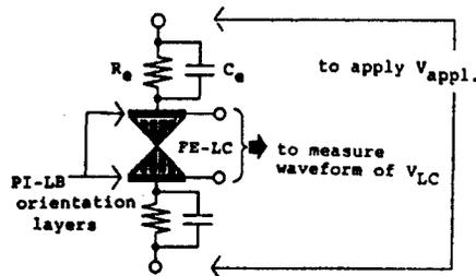
Figure 6. Measuring Circuit Composition
