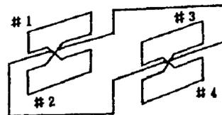
Figure 3. Connection of Ground Coils Serving for Both Levitation and Guidance
