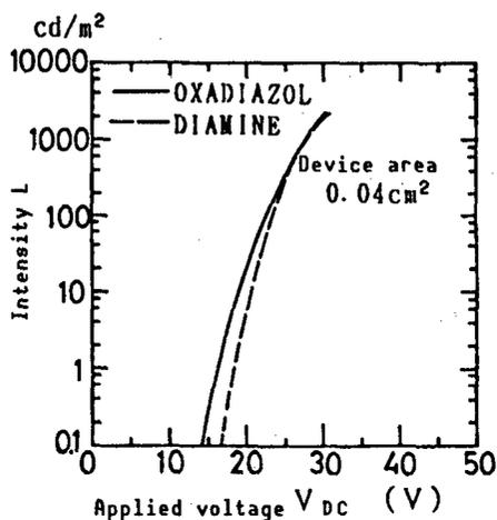
Figure 2. Intensity and Voltage Characteristics of Organic Thin Film EL Device
