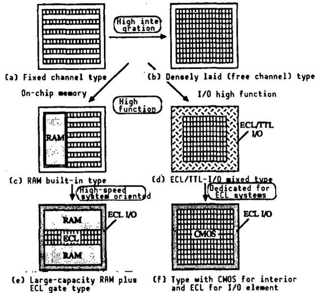
Figure 3. Examples of Representative Master Constructions
