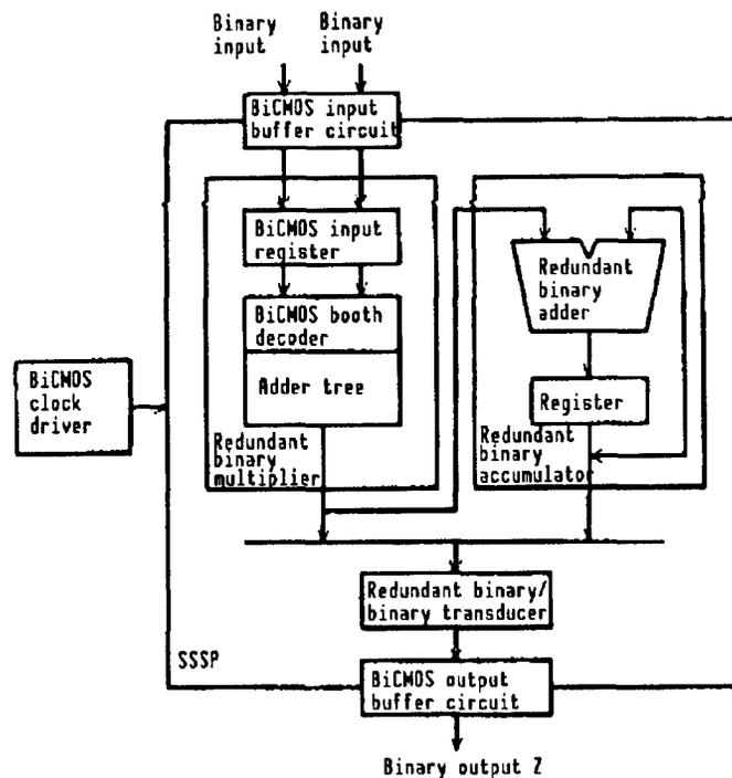
Figure 10. SSSP-LSI Configuration and BiCMOS Circuit-Applied Portions
