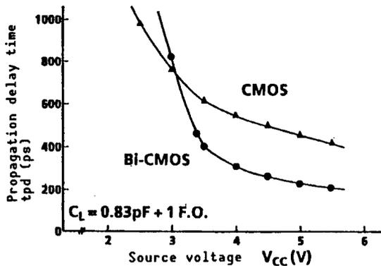
Figure 7. Source Voltage Dependency of Propagation Delay Time
