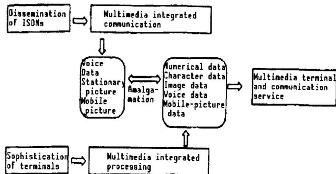
Figure 1. Amalgamation of Multimedia Integrated Communication and Multimedia Integrated Processing
