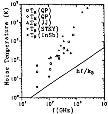
Figure 3. Current State of Performance of Superconductor Mixers
