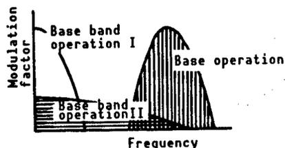
Figure 5. Base Band Modulation and Band Modulation
