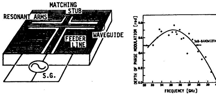
Figure 6. Band Modulator Using Resonant Electrodes<sup>9</sup>
