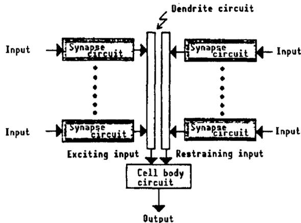
Figure 1. Circuit Construction of Hardware Representing a Nerve Cell
