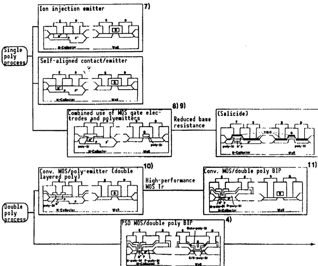
Figure 4. Transition of BiCMOS Device Structure
