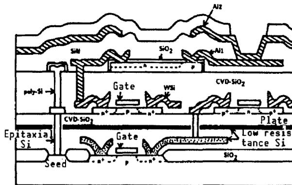
Figure 6. Cross Section of a Parallel Image Processor
