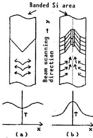
Figure 1. Temperature Distribution Patterns in Laser Beam Recrystallization
