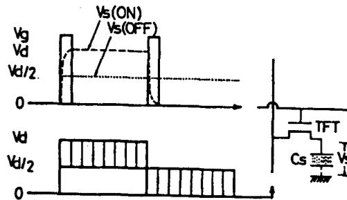
Figure 3. Principle of Active Matrix Drive
