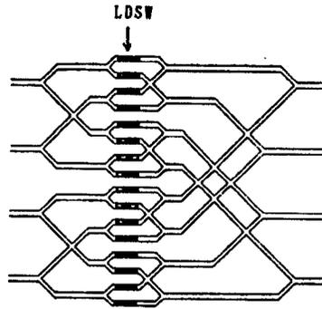
Figure 13. Example of Configuration of Tree-Type 4 x 4 Optical Matrix Switch
