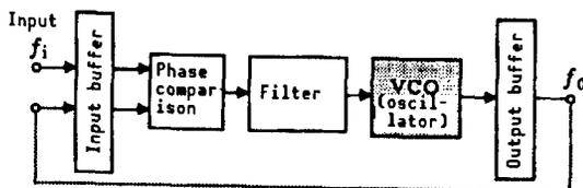
Figure 11. Configuration of PLL Circuit
