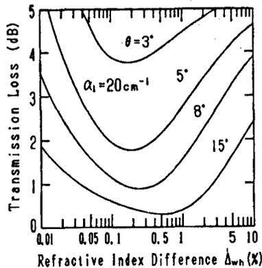
Figure 6. Insertion Loss at Transmission Side Port<sup>10</sup>
