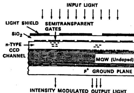
Figure 1. Block Diagram of AlGaAs/GaAs MQW Spatial Light Modulator
