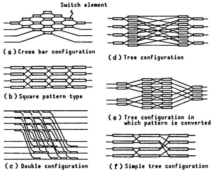
Figure 2. Configuration of Nonblocking Matrix Optical Switch
