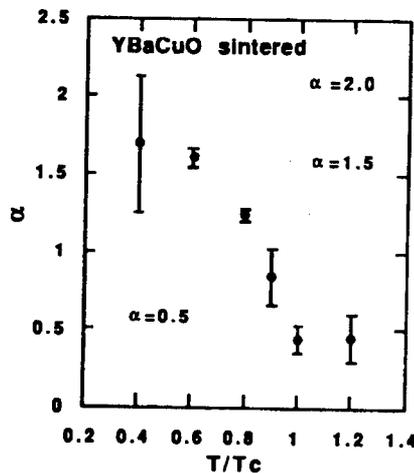
Figure 8. Frequency Dependency of an Oxide Superconductor
