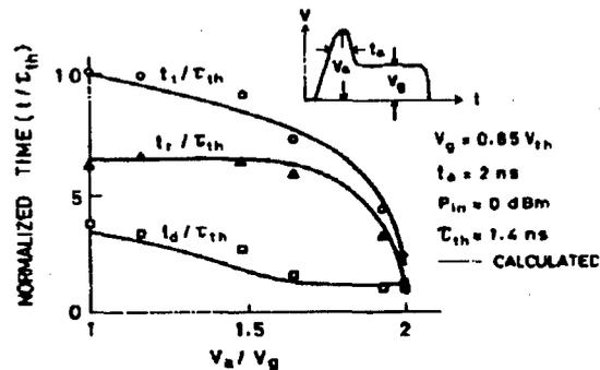
Figure 4. Rise Time Shortening Effect by Overshoot Waveform<sup>7</sup>
