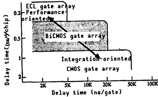
Figure 2. Trend of Gate Array Integration and Speed
