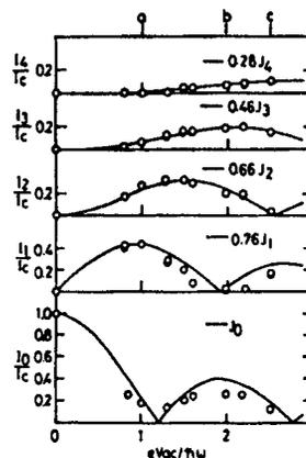
Figure 6. Irradiation Power Dependency of Shapiro Steps in a YBaCuO Point-Contact Junction
