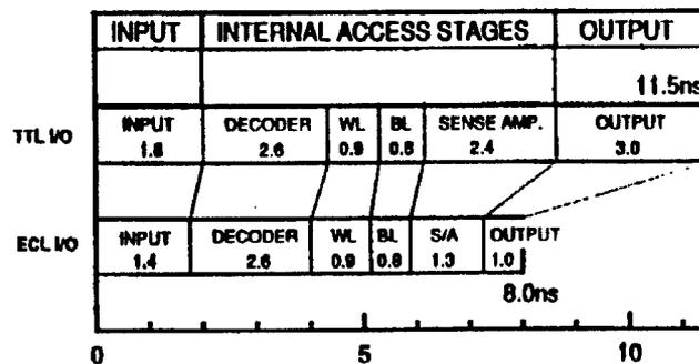
Figure 8. Comparison of Access Time Between TTL-/ECL-Specification SRAMs
