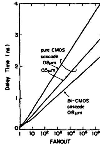
Figure 4. Total Fanout Dependency of Inverter Chain
