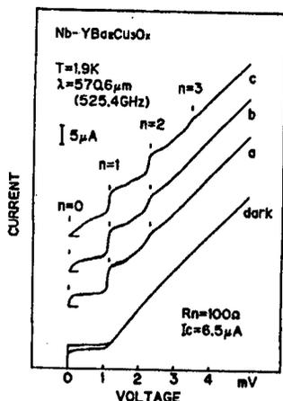
Figure 7. I-V Characteristics of a YBaCuO Point-Contact Junction (Wavelength =  $570.6 \mu\text{m}$ , frequency =  $525.4 \text{ GHz}$ )
