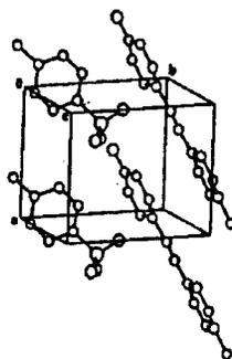
Figure 2. Crystal Structure of Merocyanine·pTS Complex Salt
