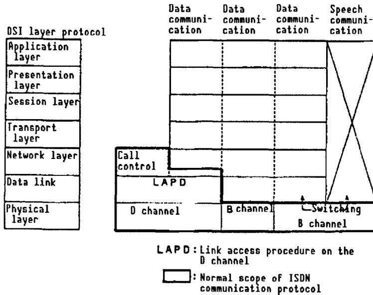
Figure 8. Configuration of ISDN Communication Protocol
