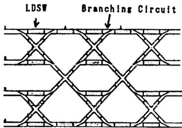
Figure 12. Example of Configuration of Link-Type 4 x 4 Optical Matrix Switch<sup>16</sup>
