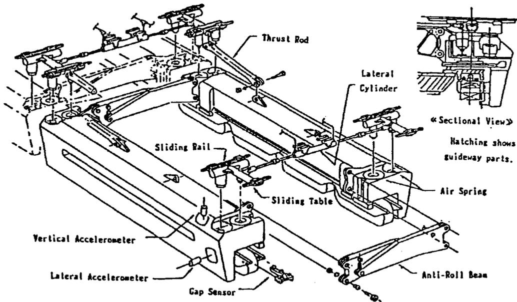
Figure 2. Module Installation
