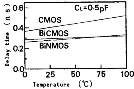
Figure 8. Relationship Between Delay Time and Temperature of CMOS, BiCMOS, and Bi-nMOS Invertors (calculated result)
