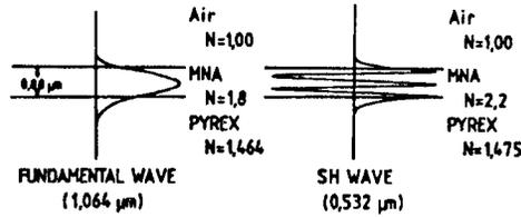
Figure 3. Field Distribution in MNA Waveguide
