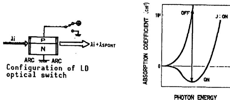
Figure 1. Principle of LD Optical Switch
