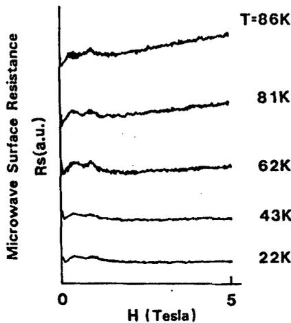
Figure 9. Magnetic Resistance of a  $\text{YBa}_2\text{Cu}_3\text{O}_y$  Single Crystal
