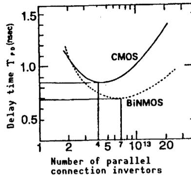
Figure 6. Relationship Between Delay Time  $T_{pd}$  and  $L$ , the Number of Parallel Connections of the Drive Circuit (calculated result)
