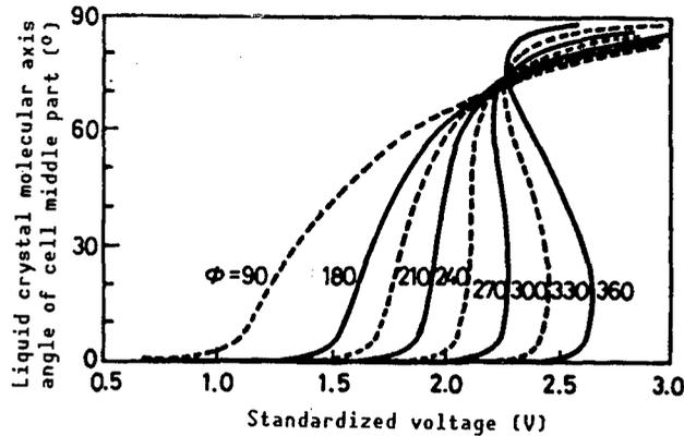
Figure 2. Characteristics of Liquid Crystal Molecular Axis Angle and Applied Voltage in Liquid Crystal Cell Layer Middle Part of Twisted Angle  $\phi^2$
