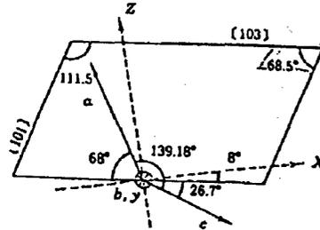
Figure 1. Parallelogrammic Plate Shape of MNA Crystal
