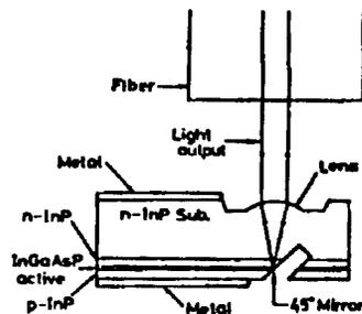
Figure 15. Monolithic Beam Spot Size Matching Circuit<sup>17</sup>
