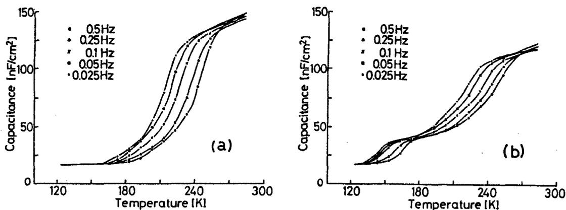
Figure 4. Temperature and Frequency Characteristics of Sample Capacitance
