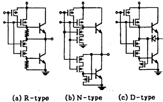
Figure 4. Gate Circuit Constructions
