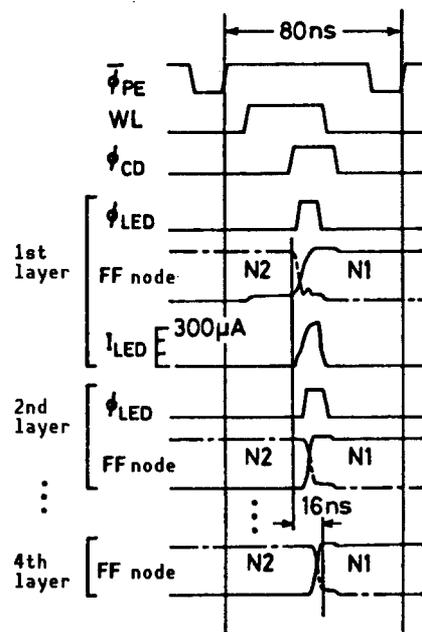
Figure 9. Transfer of Data Through Multilayers in a Three-Dimensional Photocoupled Shared Memory
