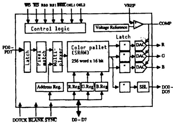
Figure 9. Configuration of Color Pallet LSI
