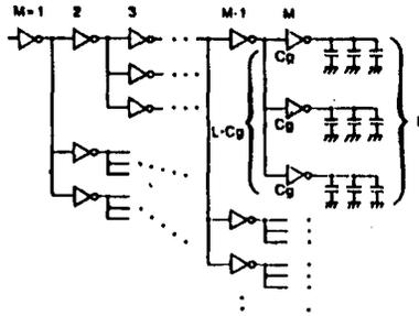
Figure 5. Drive Circuit With Its Inverters Connected in Serial and Parallel Multiple Stages in the Form of a Tree
