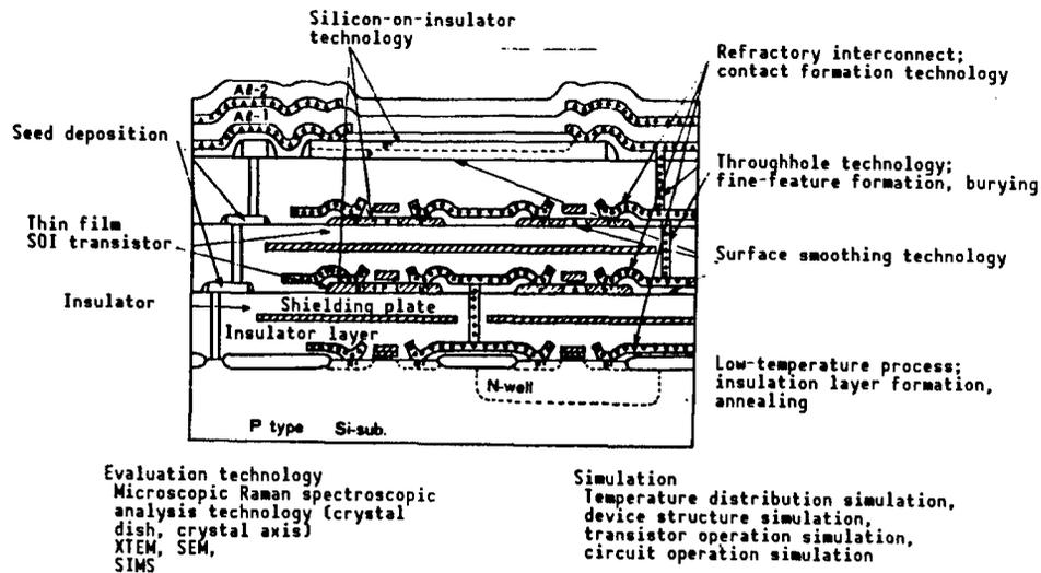
Figure 1. Cross Section of Multilayer Device Structure With Description of Device Fabrication Technologies Involved
