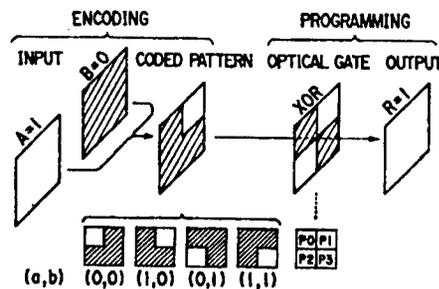
Figure 4. Composition of Optical Computing System by Pattern Coding
