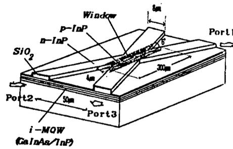
Figure 10. Three-Dimensional Drawing of Transposition-Type Optical Switch<sup>6,7</sup>
