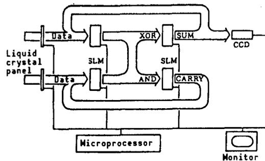
Figure 8. Composition of Parallel Optical Adder
