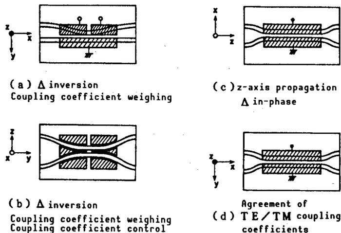
Figure 3. Optical Switch Element Without Dependence on Light Polarization
