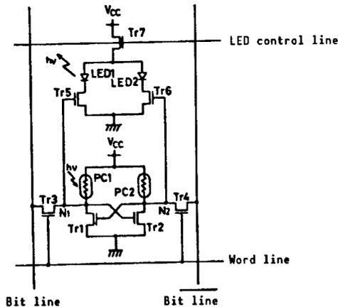
Figure 7. Circuit Diagram of Memory Cell of a Three-Dimensional Photocopied Shared Memory
