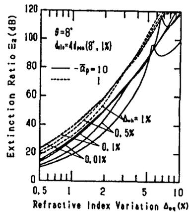
Figure 5. Extinction Ratio at Transmission Side Port<sup>10</sup>
