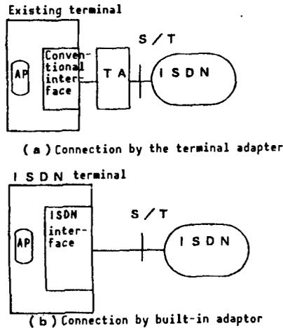
Figure 6. Terminal Connection to ISDN
