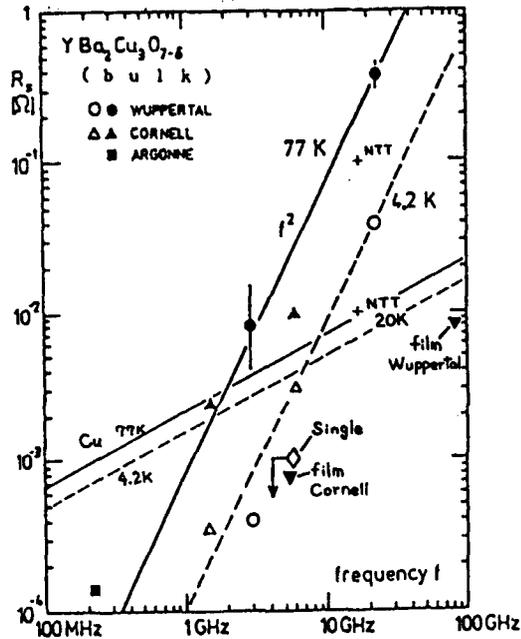
Figure 2. Surface Resistance Value Data of Oxide Superconductors
