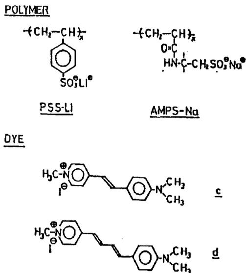
Figure 4. High Concentration Pigment Dispersion Polymer Complex
