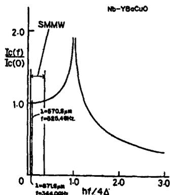
Figure 1. Frequency Dependency of Josephson Current in a YBaCuO-YBaCuO Junction
