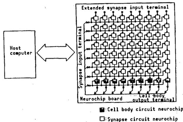
Figure 5. Circuit Construction of a Neural Network System
