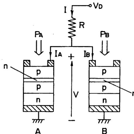
Figure 4. Block Diagram of Differential-Type Optical Switch Element
