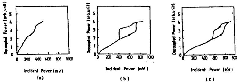
Figure 6. Input/Output Characteristics of Optical Bistability
