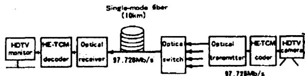
Figure 10. High Definition Video Distribution Transmission Experiment System<sup>14</sup>
