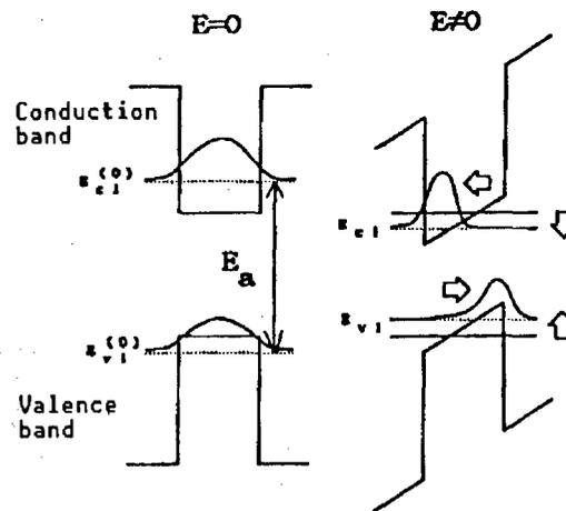
Figure 1. Change of Quantization Level and Wave Function by Electric Field Impression on Quantum Well
