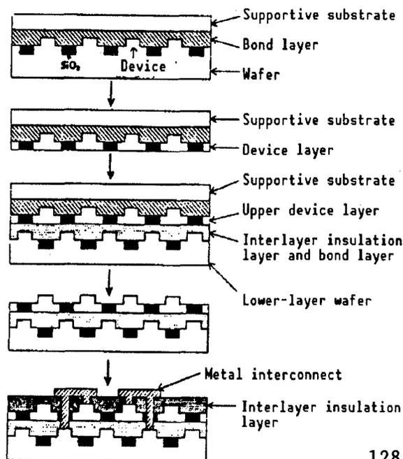
← Figure 3. Device Transfer Method
