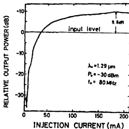
Figure 2. Characteristics of Injection Current Against Optical Output<sup>2</sup>
