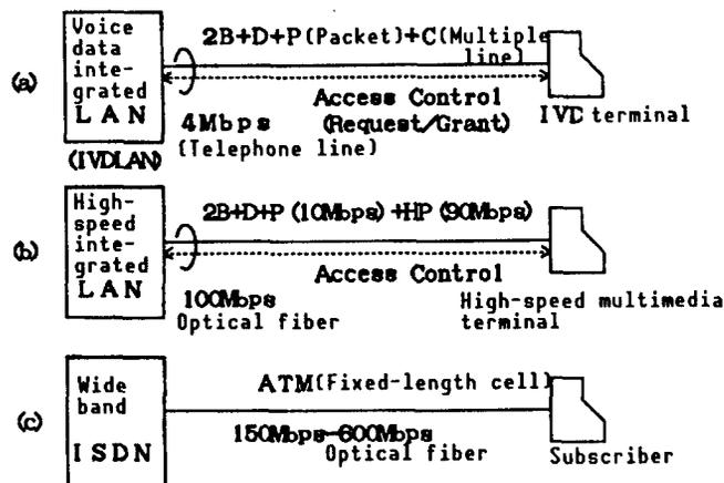
Figure 3. User Access Interfaces of Integrated Networks
