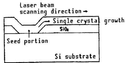
Figure 2. Laser Beam Recrystallization Using a Seed Crystal
