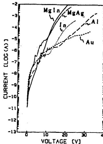
Figure 3. Metal Electrode Material Dependency Against Current-Voltage Characteristic
