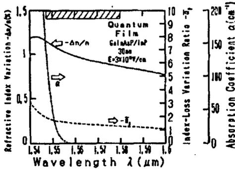
Figure 2. Change of Refractive Index of Quantum Well and Spectra of Parameter  $\bar{\alpha}_p$  10,11
