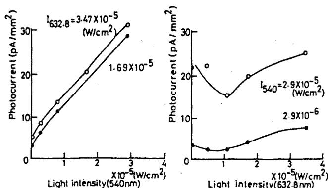
Figure 7. Photoelectric Effect of Selective Adsorption LB Film
