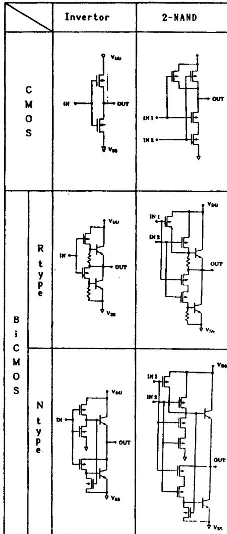
Figure 2. Examples of CMOS and BiCMOS Logic Circuits
