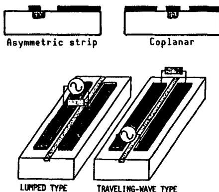
Figure 1. Typical Electrode Structure of and Feeding Current Method for Waveguide-Type Electrooptic Modulator
