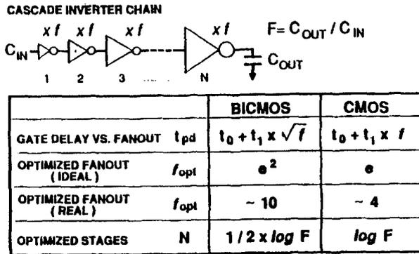
Figure 3. Minimum Delay Design of Inverter Chain
