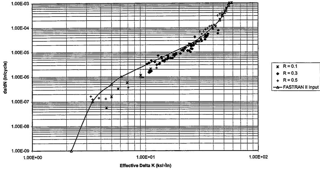
Figure 5  $da/dN$  vs  $\Delta K$  Effective Data for  $\alpha = 3.0$ , based on raw data
