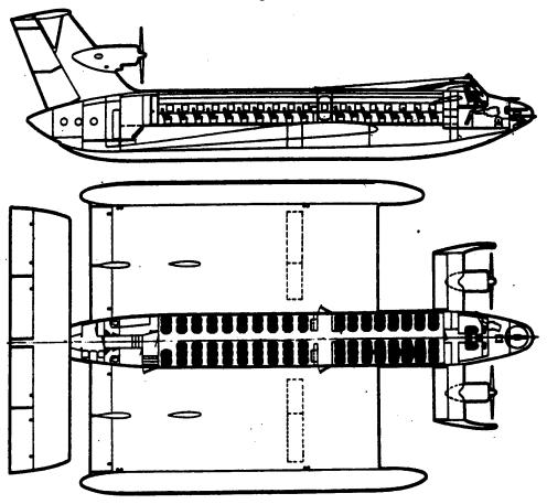
nozzles in front of the wing. Four VAZ-413 model series production, four-stroke, two-section, rotating piston gas- powered engines with air-liquid cooling systems are used as the main engines. A reduction gear and an expanding clutch have been installed in the air propeller drive system. There are remote-controlled horizontal blades-flaps on the rear section of the ring nozzles that are designed to divert the air stream and also additional rudders behind the propellers.
